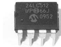
Figure 17-2: Microchip Technology's 24LC512 EEPROM
