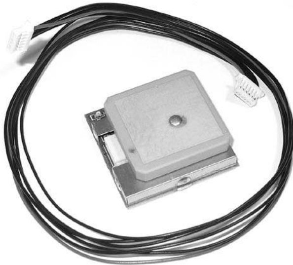
Figure 13-3: A long GPS-receiver-to-shield cable
