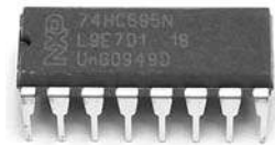
Figure 6-4: The 74HC595 shift register IC
