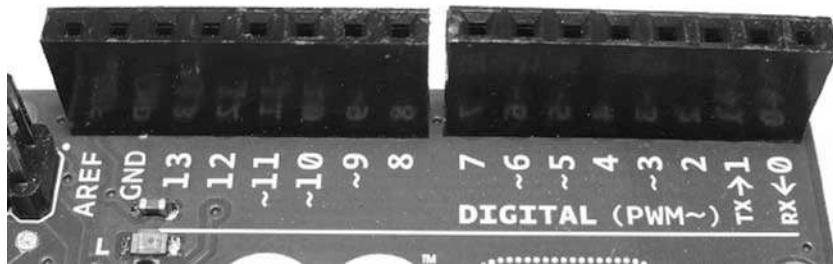
Figure 3-15: The PWM pins are marked with a tilde (~).
