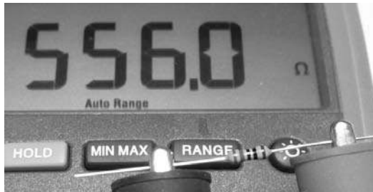
Figure 3-4: Multimeter measuring a 560-ohm 1 percent tolerance resistor
