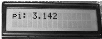
Figure 7-4: LCD displaying a floating-point number
