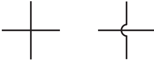
Figure 4-8: Nonconnecting crossed wires
