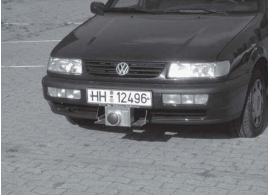
Figure 6–21 Experimental car of the Technical University of Hamburg–Harburg equipped with a 77 GHz far range radar sensor. (From [10], © IEEE 2001)
