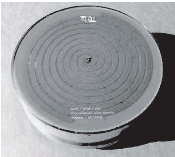
Figure 10–10 Spiral antenna. (Courtesy IRCTR: Reprinted with permission.)
