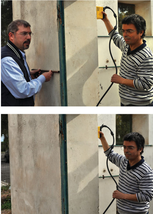
Figure 2.1. Upper panel: A metallic rod is placed horizontally on the other side of the prospected wall. Lower panel: The metallic rod is removed. The antennas have been moved in both cases downward along a vertical line.
