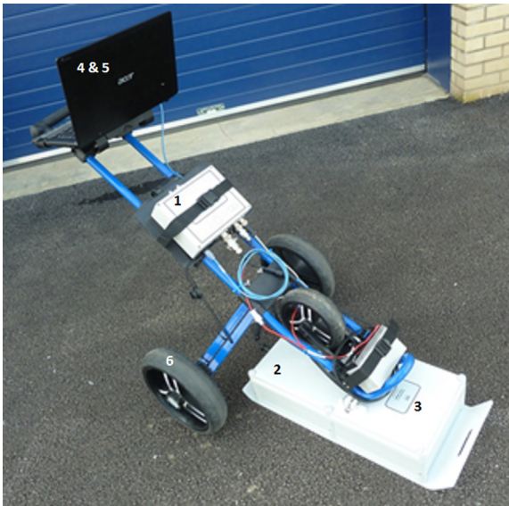
FIGURE 1.1 The basic elements of a GPR system: 1, controller; 2, transmitter antenna; 3, receiver antenna; 4 and 5, laptop for data storage and monitoring; and 6, encoder wheel for distance measurement.
