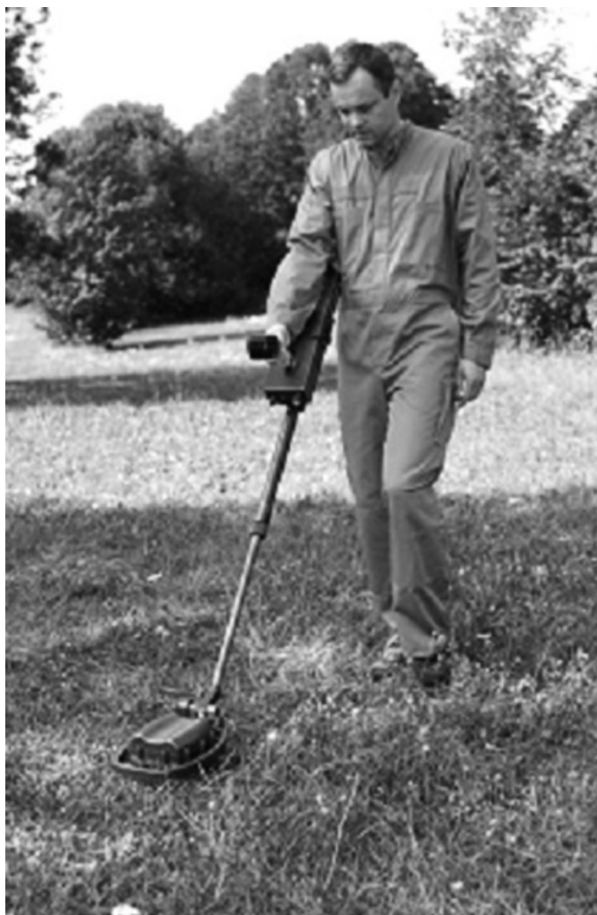
Figure 14.9 Ground survey with ALIS system (Courtesy: Prof. M. Sato). Two shielded spiral antennas are seen within the coil of a metal detector.
