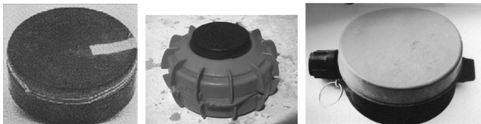
Figure 14.1 Photos of antipersonnel (AP) mines: PMA3 (left), VS-50 (center), and PMN2 (right).
