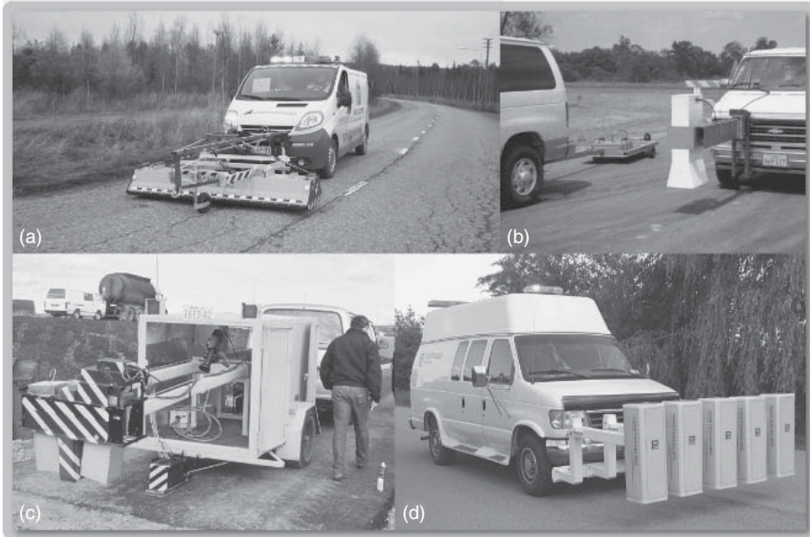
Figure 13.2 Different GPR systems and antenna configurations used in road surveys. Photo (a) presents a multichannel stepped frequency radar by 3D Radar from Norway; photo (b) presents a 100 MHz GSSI ground-coupled antenna and a 1.0 GHz Pulse Radar antenna used by the Texas Transportation Institute (TTI); photo (c) presents a Canadian Road Radar system that has a horn antenna system and a multichannel ground-coupled antenna array (see Davis et al., 1994), and photo (d) presents a multichannel air-coupled horn antenna system by Penetradar.
