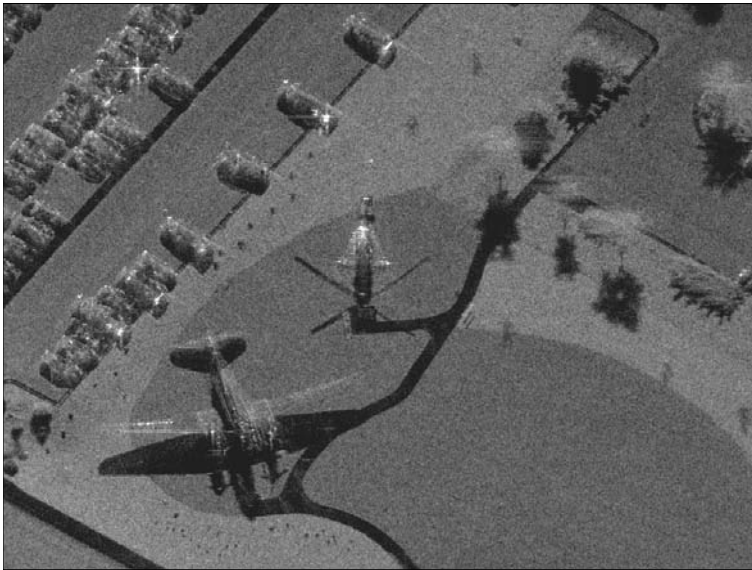
Figure 11.1. A 4-inch resolution Ka-band image from Sandia National Laboratories [127]. Note the shadows of the historical airplane, helicopter, and trees (courtesy of Sandia National Laboratories and SPIE).
