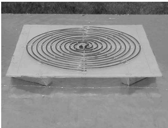
Figure 8.5. A spiral antenna (courtesy of North American Astronomical Observatory).
