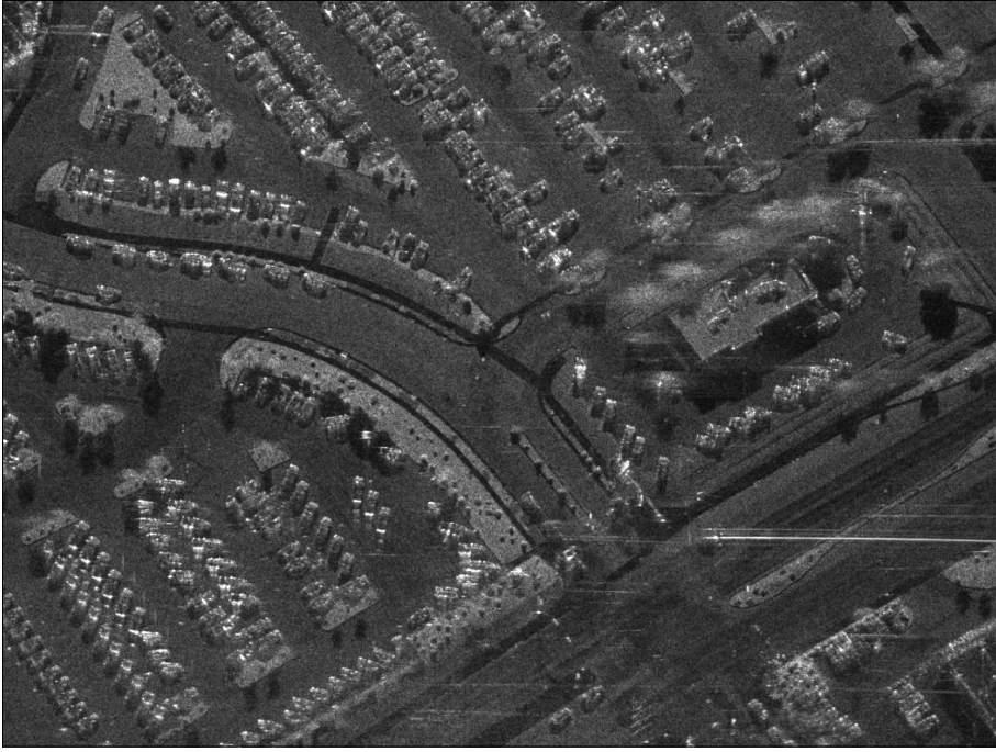
Figure 10.2. A Ku-band image showing streaking due to objects moving in the scene (courtesy of Sandia National Laboratories and SPIE).
