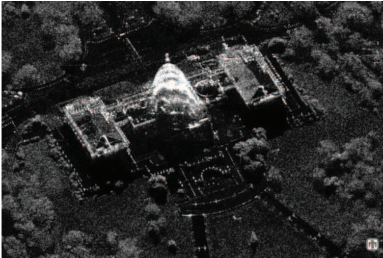
Figure 9.11. The U.S. capitol building in Washington, D.C. Notice the shadows under the trees at the bottom and the layover effect in the image of the dome (courtesy of Sandia National Laboratories).
