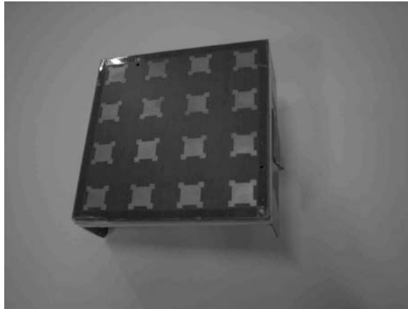
Figure 8.14. An array antenna (courtesy of Air Force Research Laboratory, Sensors Directorate).
