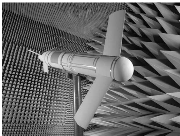
Figure 8.16. A microstrip antenna that fits into an aerodynamic structure. Such antennas are called conformal antennas (courtesy of Ball Aerospace).
