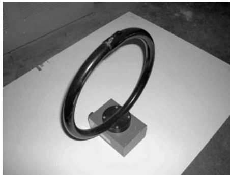
Figure 8.3. A loop antenna (courtesy of Air Force Research Laboratory Sensors Directorate).
