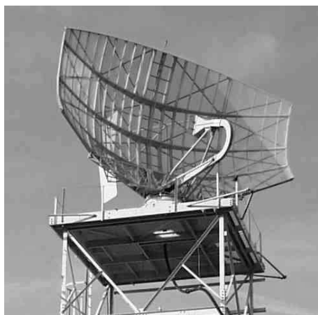
Figure 8.9. An L-band reflector antenna (courtesy of Air Force Research Laboratory Sensors Directorate).
