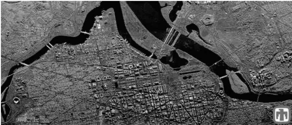
Figure 1.7. A SAR image of Washington, D.C. Although the antenna footprint is typically on the order of tens of kilometers, the images show much smaller features (courtesy of Sandia National Laboratories).
