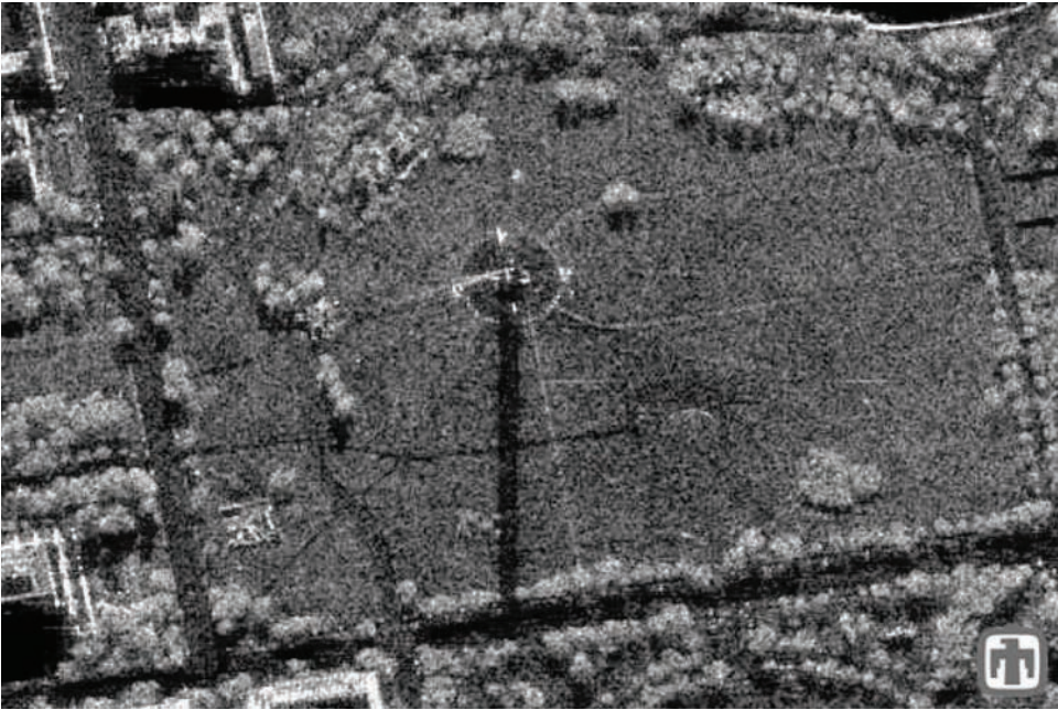
Figure 9.10. An image of the Washington Monument. The radar antenna flew along the top, as can be seen from the radar shadow of the monument. The top of the monument appears as a bright spot much closer to the radar (courtesy of Sandia National Laboratories).
