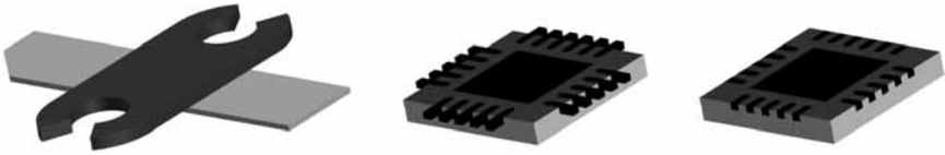
Figure 7.6 Bottom view of flange-mount, quad flat lead (QFL), and quad flat no-lead (QFN) packages.
