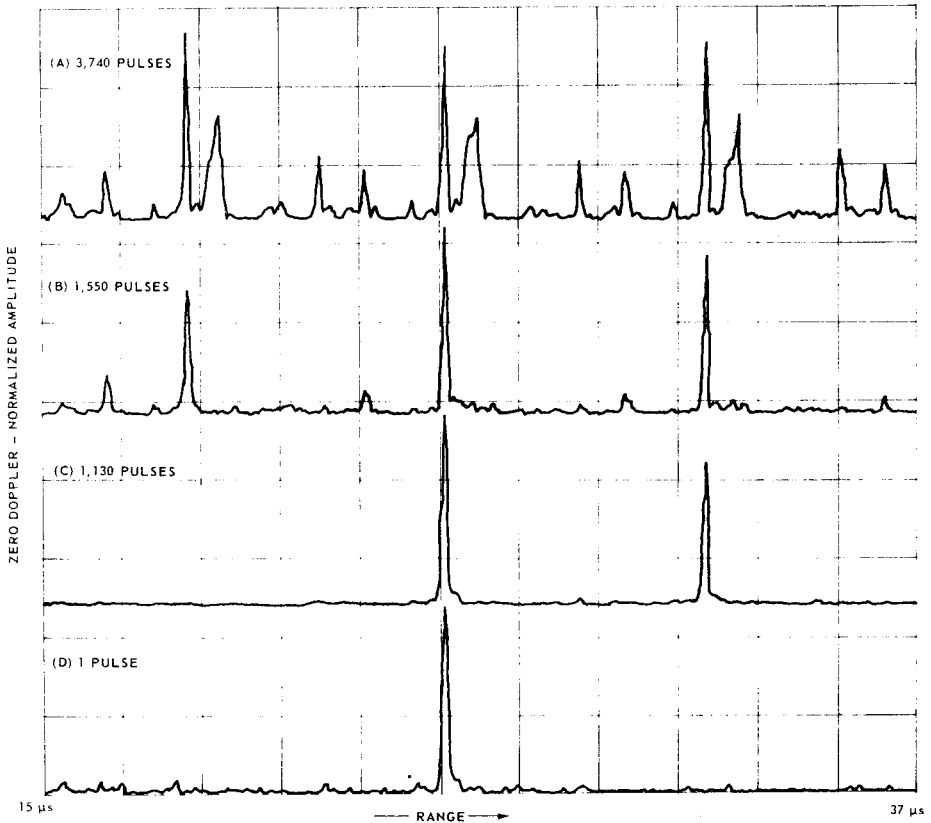
Figure 11.24 Effect of geometric programming on land clutter echoes. (A) 3740 pulses, 150 kHz—no programming; (B) 1550 pulses, geometric programming—no clutter decay; (C) 1130 pulses, geometric programming—12.8 \mu\text{s} clutter decay; (D) single 0.15 \mu\text{s} pulse. (Courtesy of A. Chwastyk)
