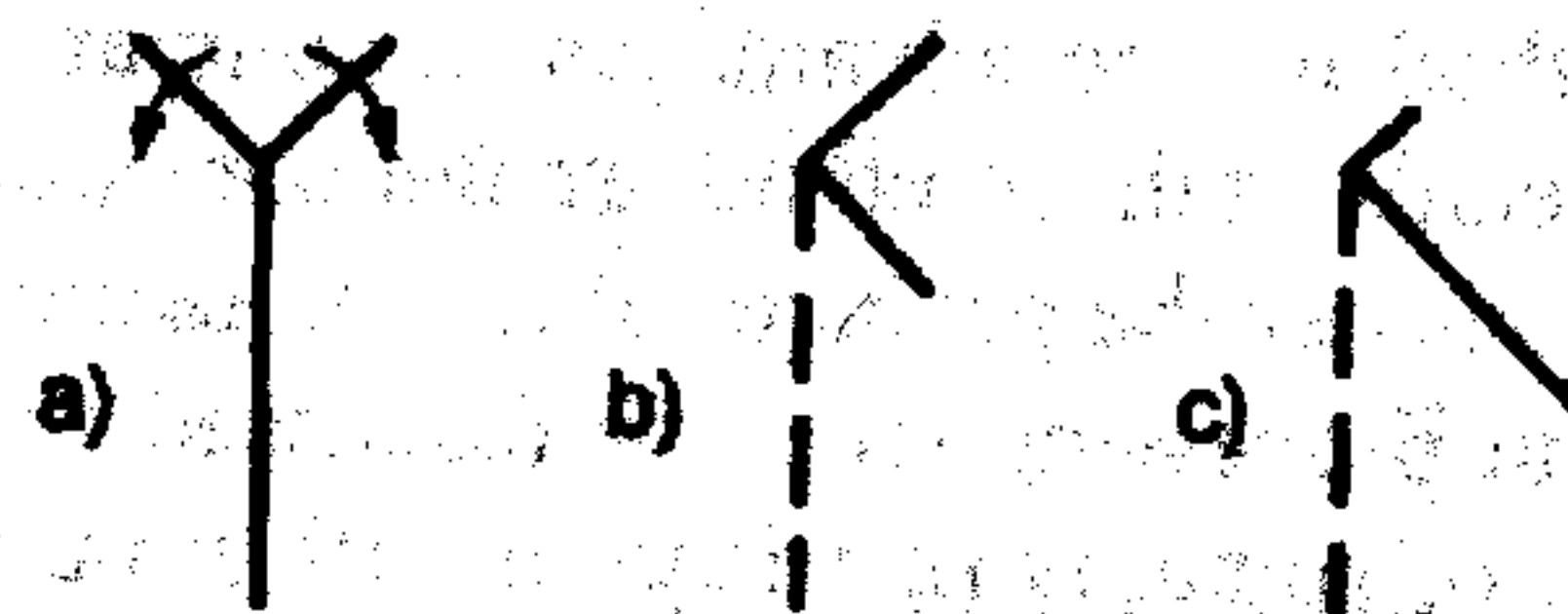
Figure 5.18 Phasor diagrams: (a) AM signal, (b) detected signal for sinusoidal modulation, and (c) detected signal for asymmetrical sawtooth modulation.
