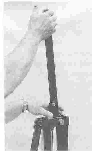
Fig. 77 Push down on the linkage with your thumb while pulling forward on the injection lever.
