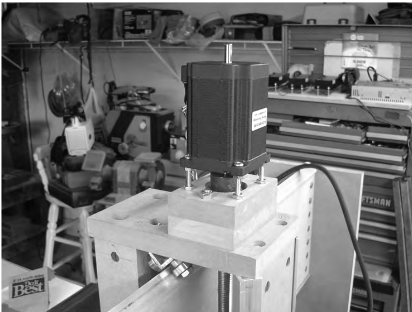
Figure 17-9. Tighten down each nut (four to the motor and four to the motor mount).
