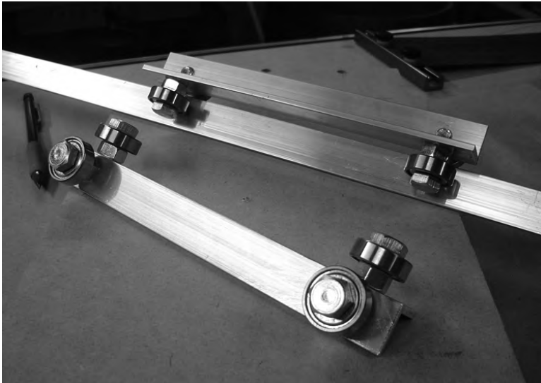
Figure 10-13. Add bolt-bearing-nut assemblies to the rails to complete your BRAs.
