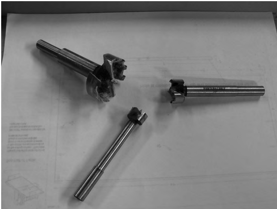
Figure 2-1. Forstner drill bits in various sizes
