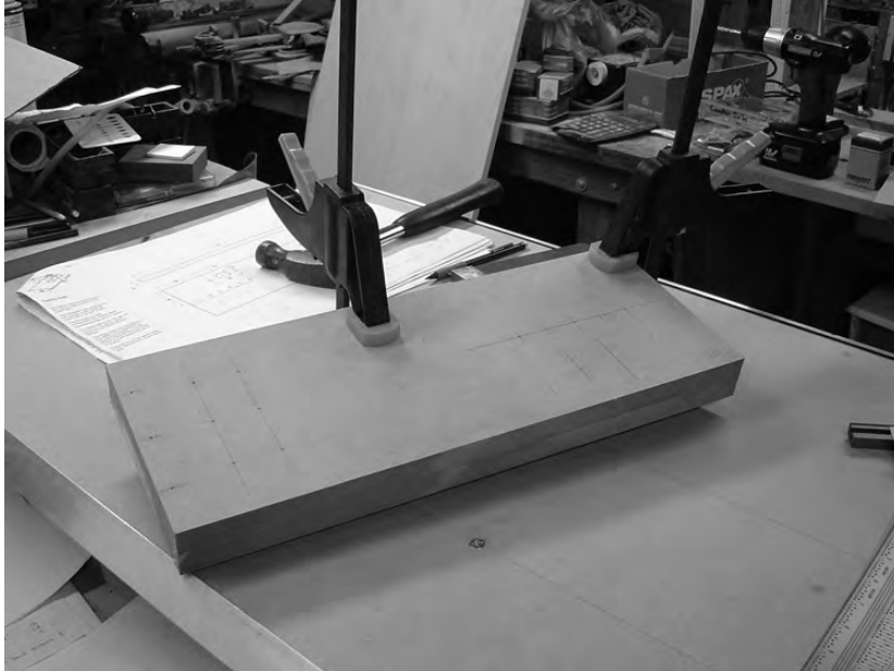
Figure 10-4. Clamp parts Q and R together before drilling.
