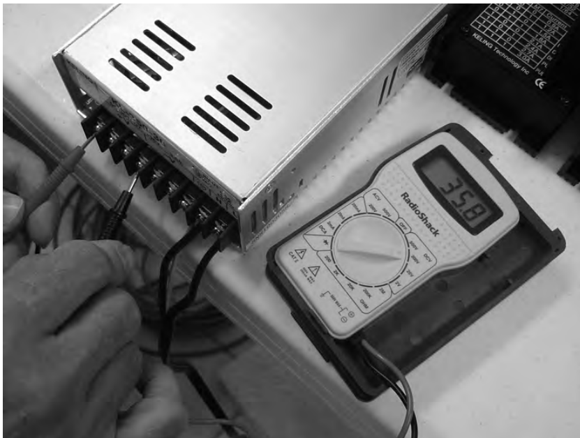
Figure 6-12. Test the voltage being supplied by your power supply.
