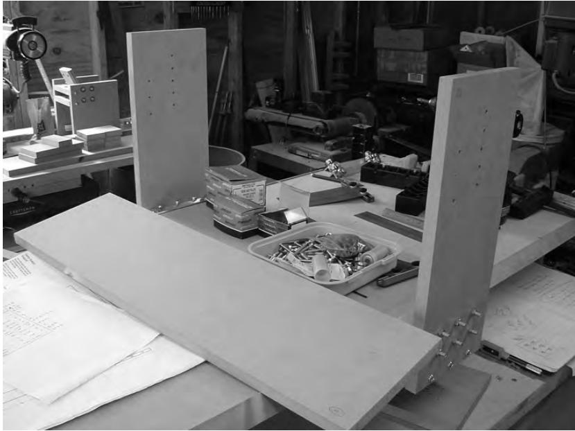
Figure 12-2. The y-axis frame is partially completed.
