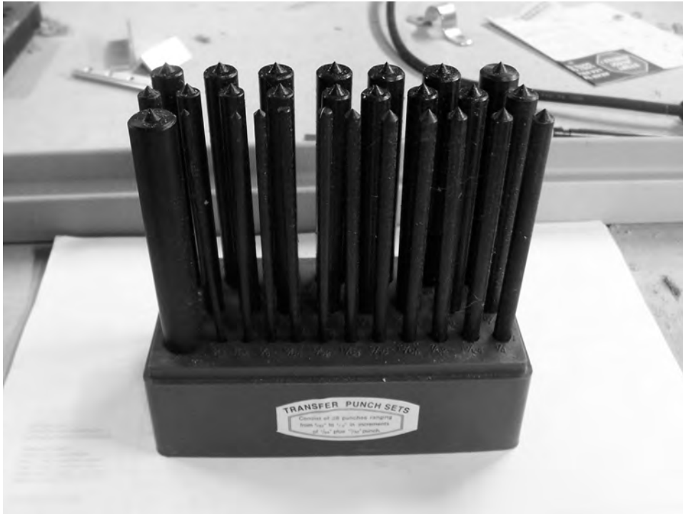
Figure 2-2. Transfer punches let you mark other pieces accurately for drilling.
