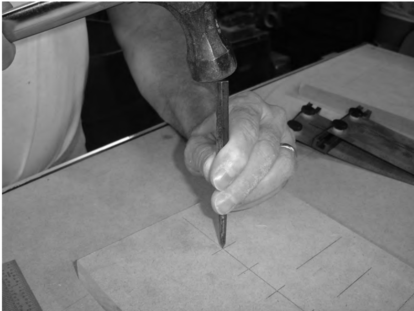
Figure 10-3. Use a center punch to create small holes to assist with drilling.
