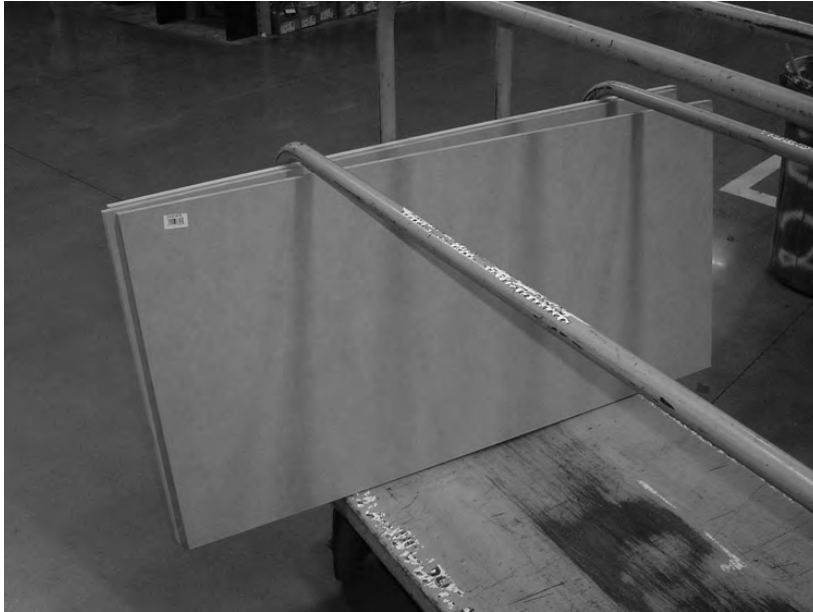
Figure 7-2. Quarter-sheets of MDF will save some cutting time—two of these make the table.
