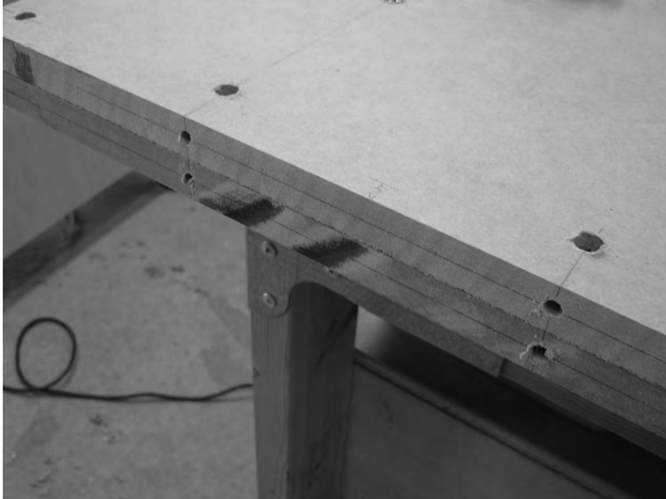
Figure 8-7. Holes drilled into the table's edges will let you attach the legs.
