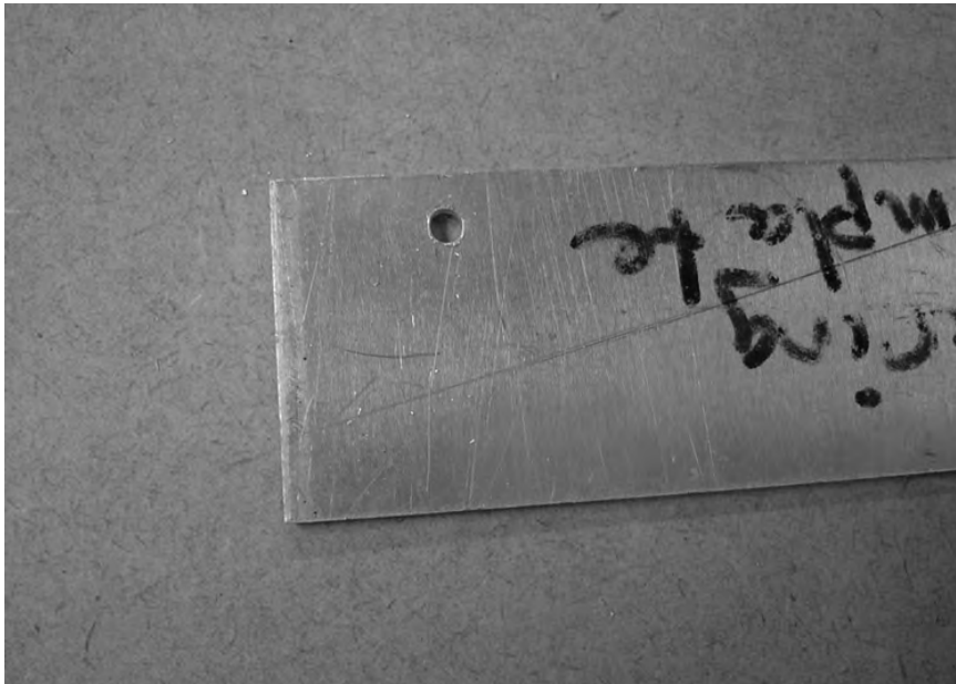
Figure 4-5. A piece of metal with a single pilot hole in it
