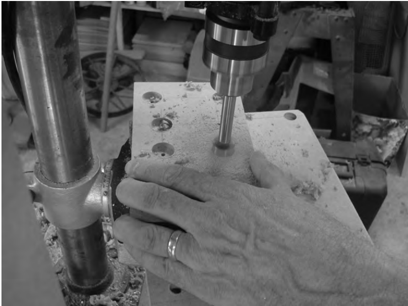
Figure 13-6. Drilling the counterbored holes in Part C
