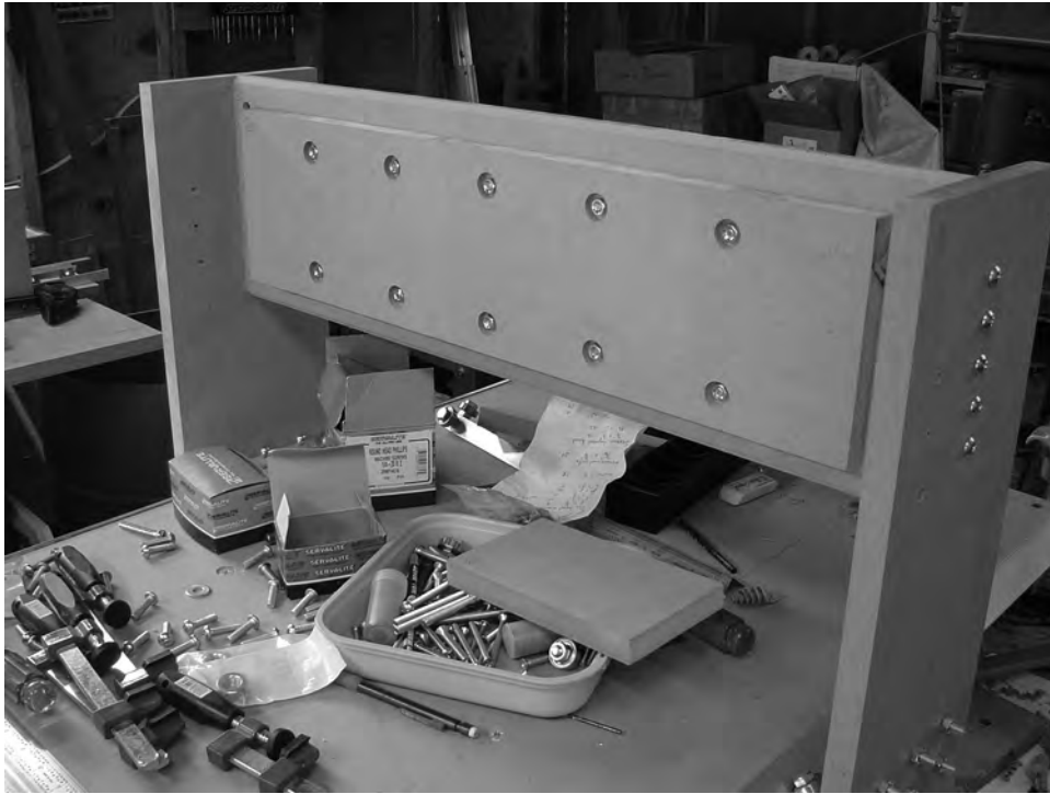
Figure 12-14. Parts O and S bolted to the gantry sides
