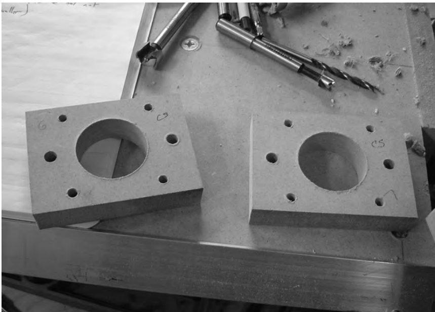
Figure 17-3. A top and bottom motor mount with corner holes drilled for motors
