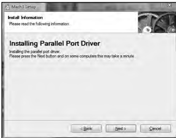
Figure 18-3. Let Mach3 install the parallel port driver.
