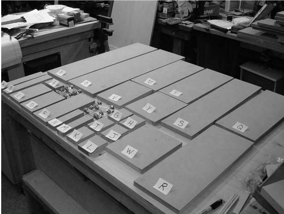
Figure 3-3. It's easier to find what you need when you label each of the MDF pieces.
