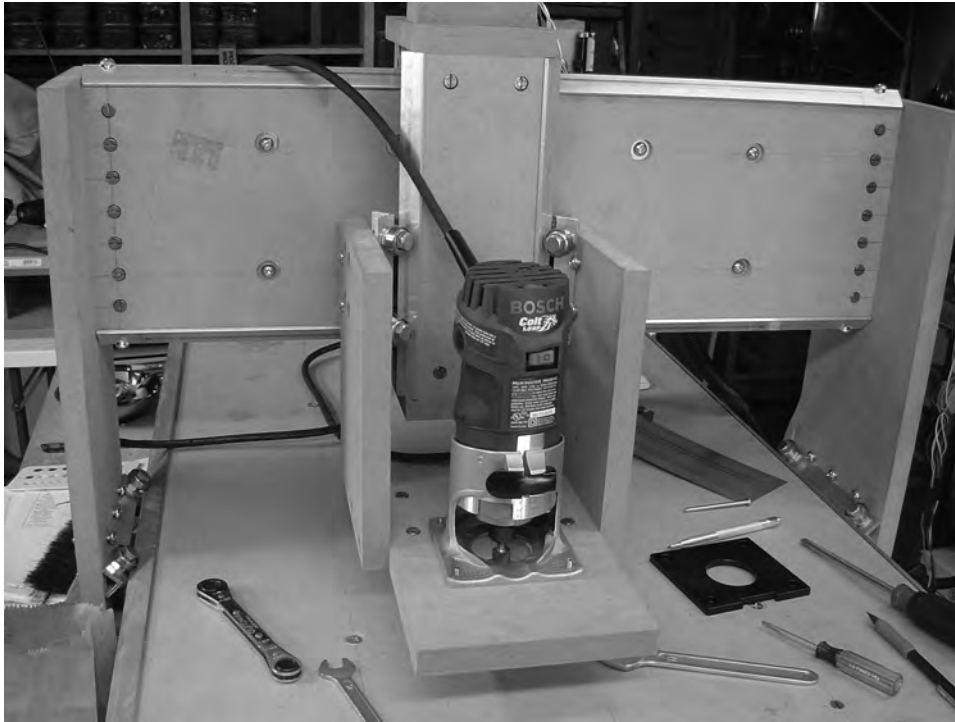
Figure 17-14. Part V is bolted back to the z-axis frame.
