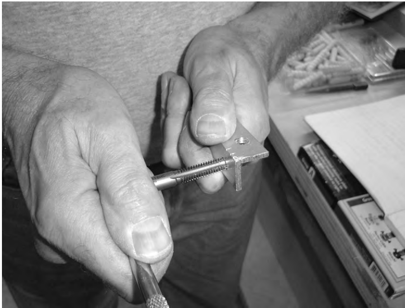
Figure 4-11. Cutting threads into one of the holes in the aluminum rail
