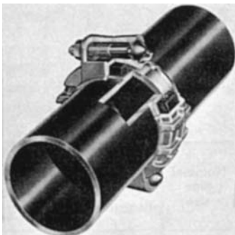
FIGURE A2.34 Victualic coupling for grooved-end cast-iron or steel pipe.
