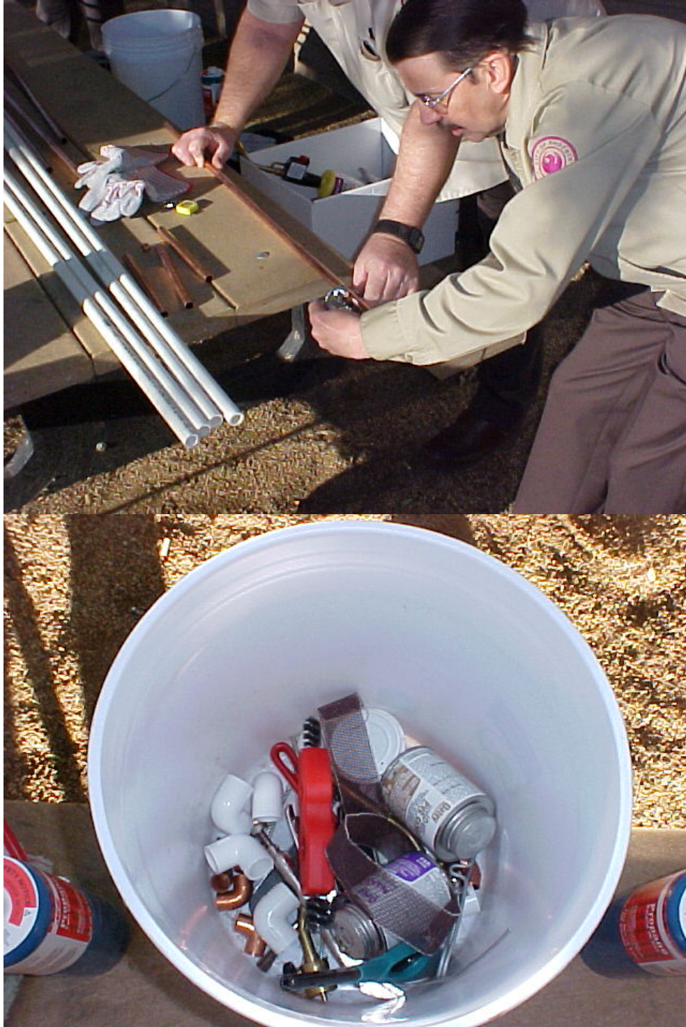
Commonly found materials used for sweating (Soldering) copper pipe and gluing (Cementing) PVC. Plumbers like to utilize 5-gallon buckets as a tool box of sorts.
