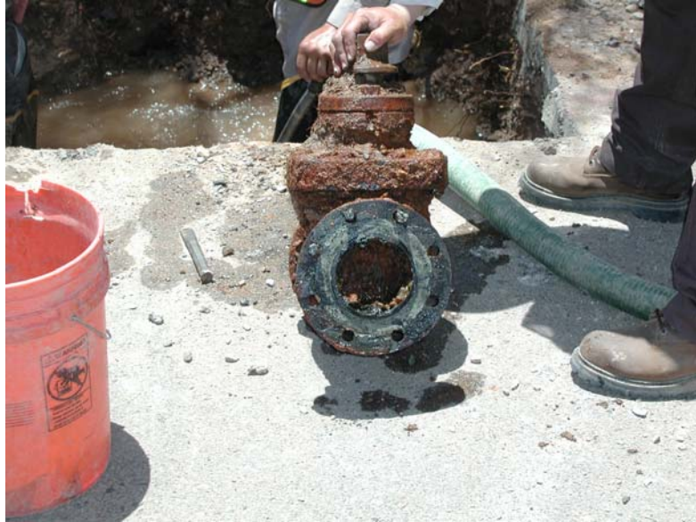
Broken gate valve with Tuberculation. Below, a large butterfly valve.
