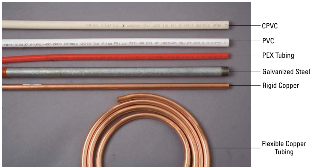
Figure 2-2: CPVC pipe, PVC pipe, PEX tubing, galvanized steel pipe, rigid copper pipe, and flexible copper tubing.
