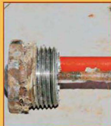
123 | Replacing Anode Rods
