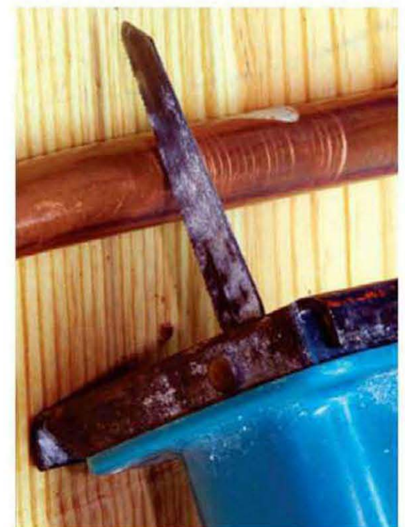
A mini recip saw can cut a tiny sliver off a copper pipe ( left ) as well as cut a copper pipe flush to the wall ( right ).
