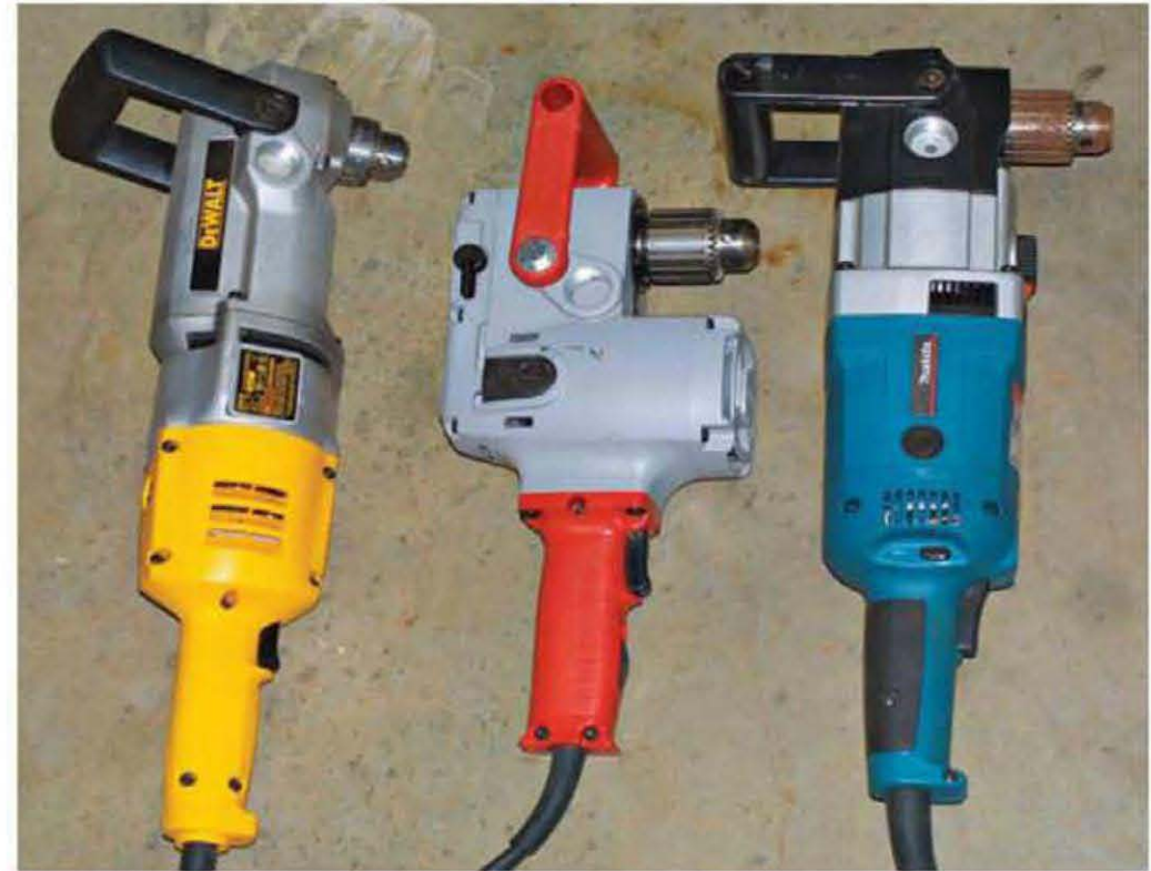
Heavy duty right-angle drills: DeWalt ( left ), Milwaukee ( center ), Makita ( right )
