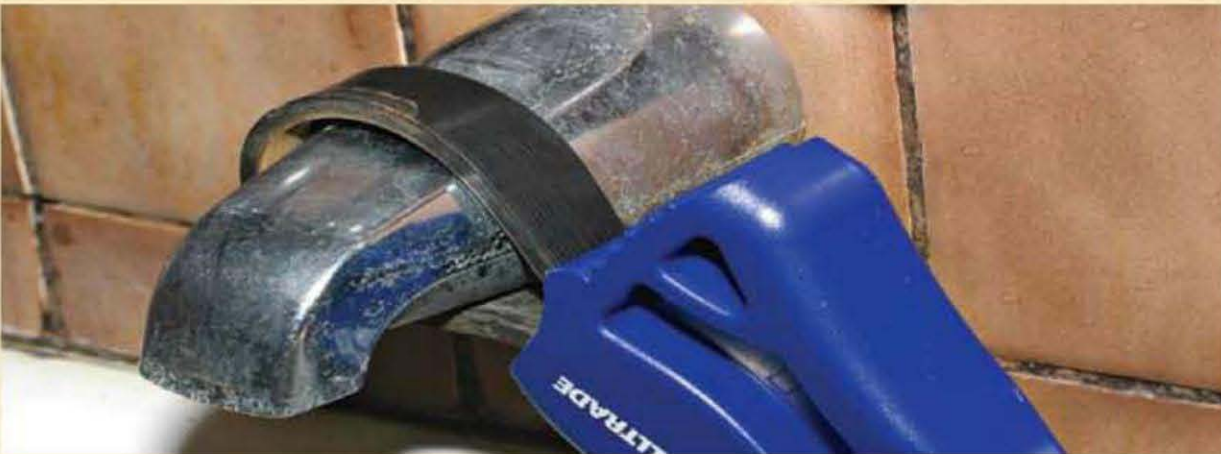
The strap wrench works well on unusual-shaped items such as tub spouts ( left ) and on rough-edged objects like glue caps ( below ).
