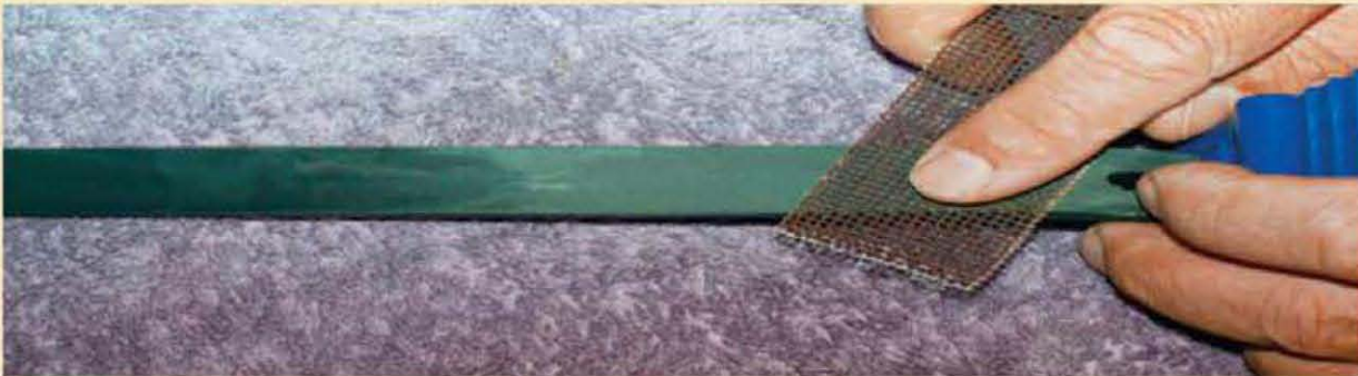
To work properly, rough up the smooth strap with sandpaper.
