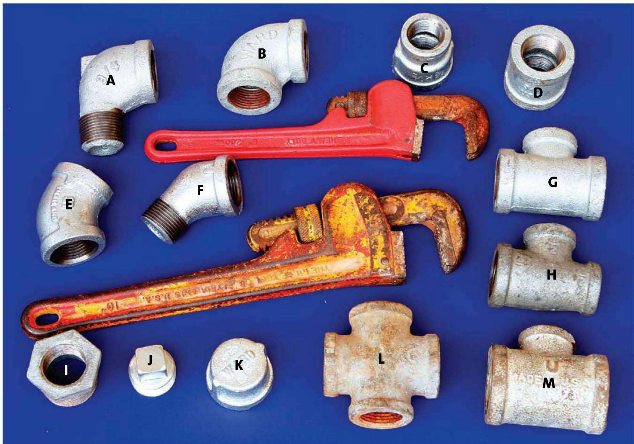
Most commonly used galvanized fittings.
