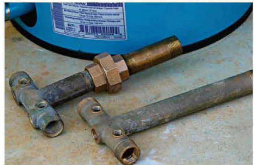
Tank Ts come with long and short shanks. The short shank allows you to install a union if the tank doesn't already have one—and most don't.
