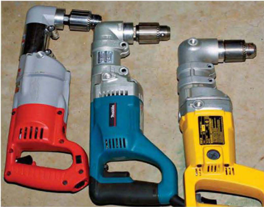
Tubular arm, right-angle drills are light and easy to use, especially overhead, but they have limited torque capability.
