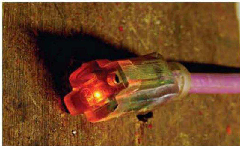
Lighted-end cords are my favorite—the second I pick it up I know if it has power.
