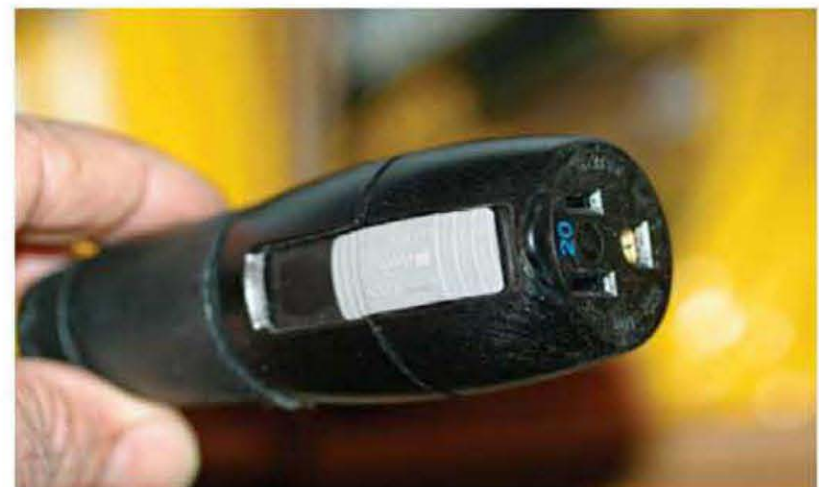
Auto locking cord ends keep the tool's plug from pulling out.
