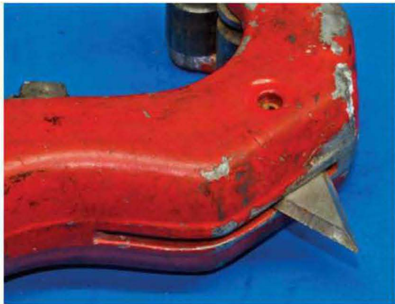
The blade that folds out on some tubing cutters ( bottom ) is used to ream out the inside of the pipe, but I have never had much luck with it. Instead, I use a stepped bit that is designed to cut steel. I simply install it in my cordless drill and press it onto the pipe ( top ).
