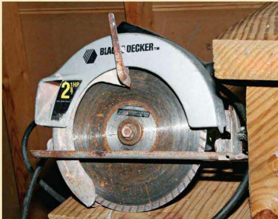
A diamond blade on a circular saw works well to cut cast iron.
