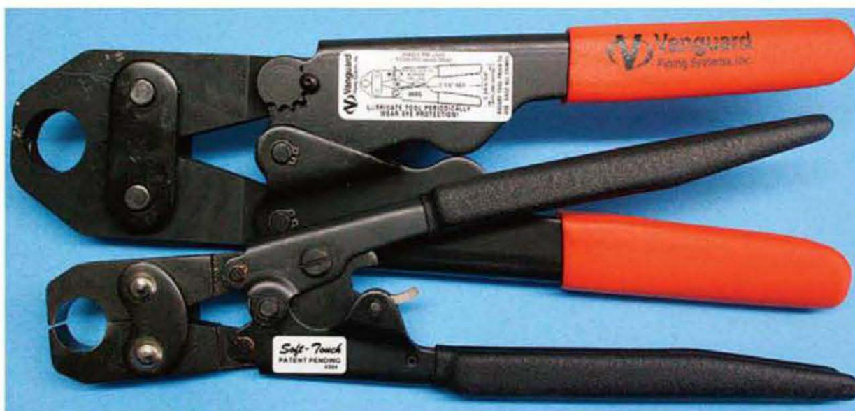
Modern crimpers are short and close easily.
