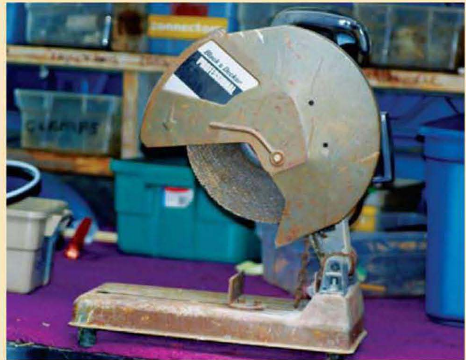
A chop saw with a solid blade works well when used to cut cast iron before it is installed.
