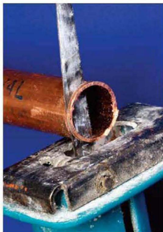
A mini recip saw can cut a tiny sliver off a copper pipe ( left ) as well as cut a copper pipe flush to the wall ( right ).
