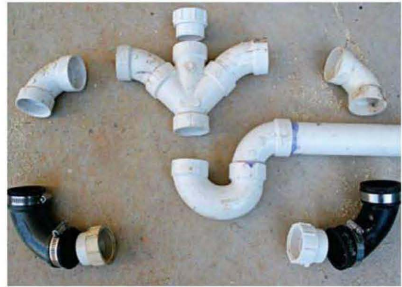
Here are all the parts to my custom kitchen sink drain: two 1 1/2-in. flexible elbows (the two PVC female adapters are only used if I need to extend the drain lower for different bowl depths), two PVC elbows, a double Y, insert male adapter on top of Y, trap, and (not shown) a few lengths of PVC pipe to connect it all.
