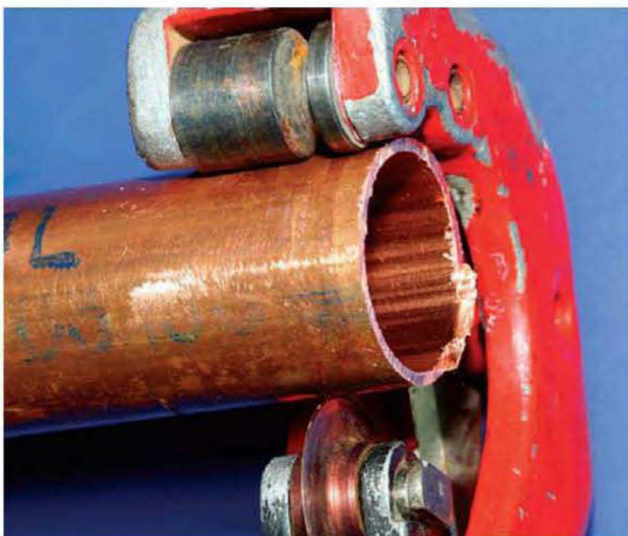
A tubing cutter, no matter how good, cannot cut really close to the edge of a pipe because of design limitations.
