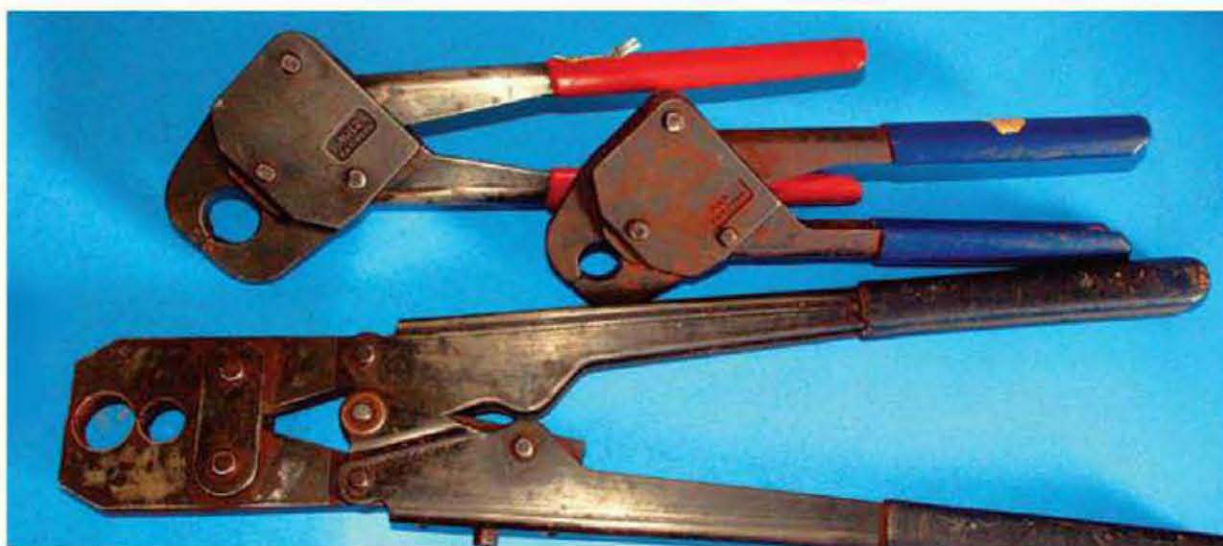
These old crimpers are a carryover from the PB days, but they still work for PEX.
