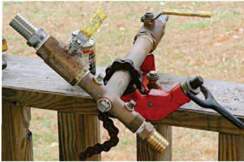
A chain vise is perfect for locking down a tank T for the installation of all its individual components.
