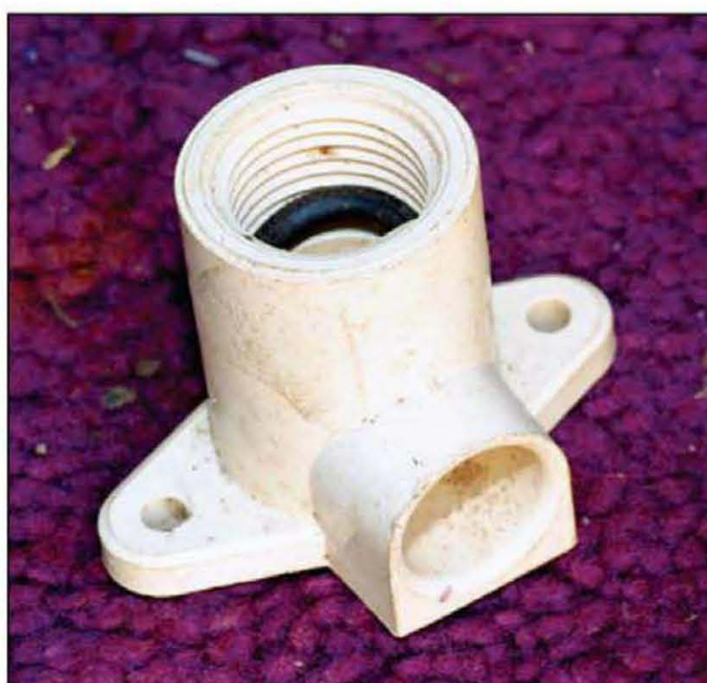
Plastic drop-ear elbows have a tendency to crack as pipes are threaded into them.
