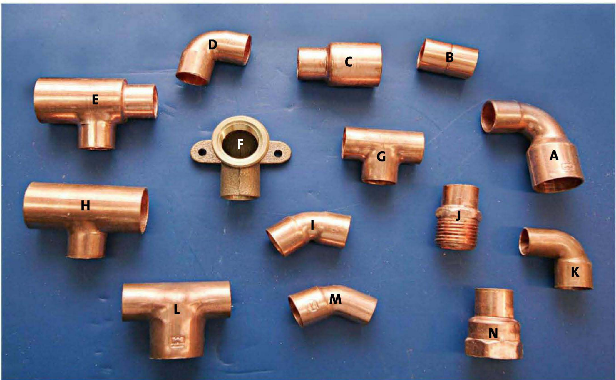
Most commonly used copper fittings. A—Reducing 90, B—Coupling, C—Reducing coupling, D—Elbow or 90, E, H, and L—Reducing T, F—Drop-ear elbow, G—T, I—45, J—Male adapter, K—Street elbow, M—Street 45, N—Female adapter
