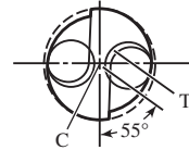
Fig. 3. The chisel edge C after thinning the web by grinding off area T .
