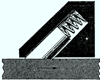
Wedge action locks the movement in the direction of the arrow.
