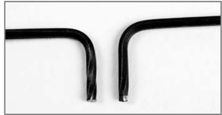
FIGURE 2-2 Allen keys that failed in torsion
