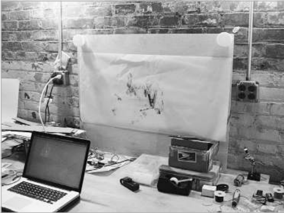
FIGURE 10-24 Motors mounted at the top corners of the plywood canvas
