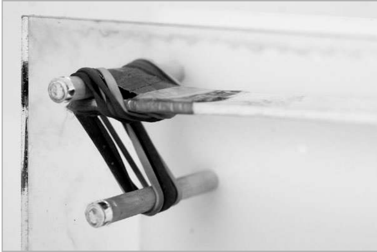
FIGURE 1-28 Fixing the paint stick in place with rubber bands
