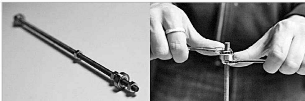
FIGURE 7-5 Installing a bearing on a threaded rod (images used with permission from MakerBot Industries)
