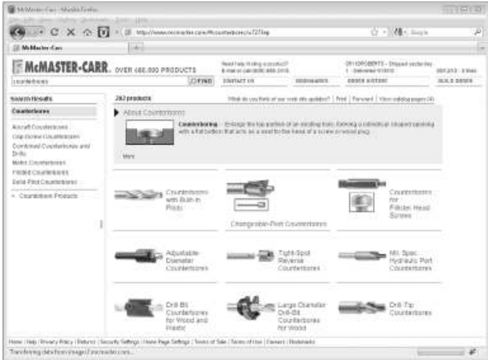
FIGURE 7-13 Counterbore bits can be used to create recesses for bearings (credit: McMaster-Carr).
