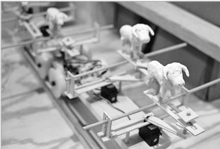
FIGURE 8-10 Scotch yoke in running of the bulls (CC-BY-NC-SA image used with permission from Greg Borenstein and Scott Wayne Indiana)
