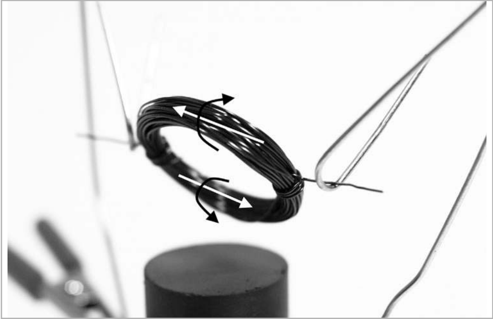
FIGURE 6-3 White arrows show direction of current flow and black arrows show the direction of the resulting magnetic field in the wire coil
