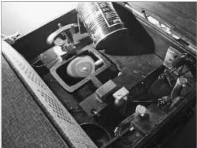
FIGURE 8-16 In this example from Andrew Jordan's Sound Creatures project, the spiral painted cam in the center throws its housing back and forth, creating irregular reciprocating motion from continuous rotary input.
