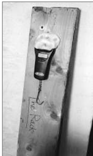
FIGURE 4-13 MakerBot Industries used The Rack to measure the pull force of its plastruder motor.
