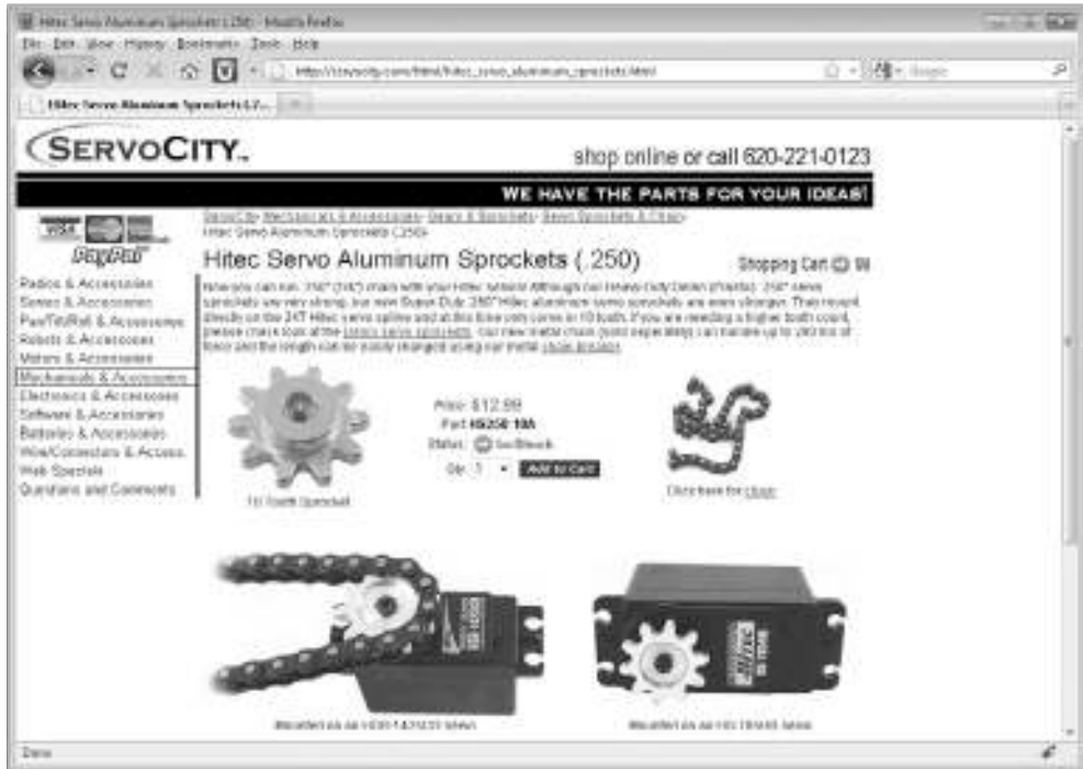
FIGURE 7-41 An aluminum sprocket and 1/4 in chain mounted to a servo motor (credit: ServoCity)
