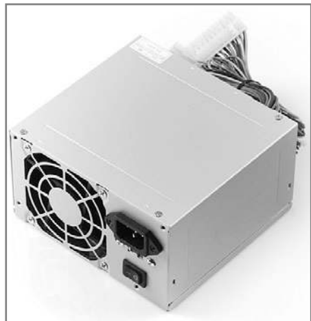
FIGURE 5-7 A computer ATX power supply (image used with permission from SparkFun Electronics)
