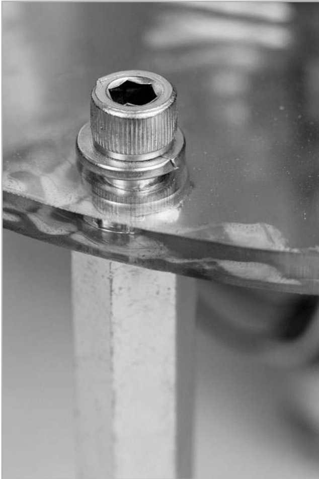
FIGURE 10-12 Detail of installing the standoffs
