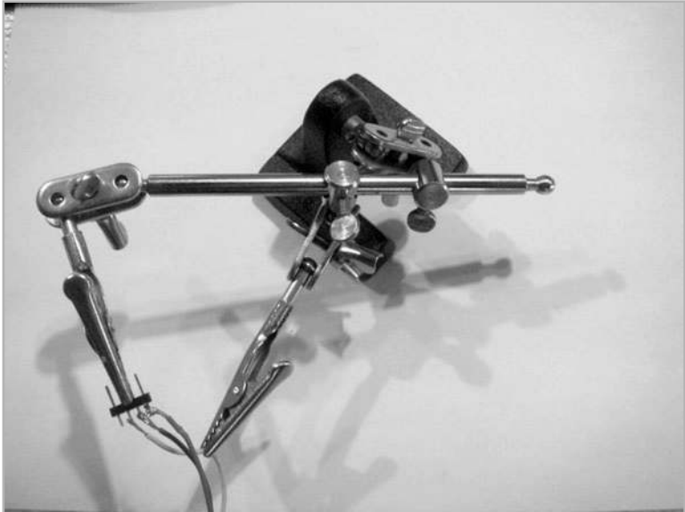
FIGURE 6-37 Soldering male headers onto the stepper motor wires before (top) and after strain relieving with a cable tie and insulating with hot glue (bottom)
