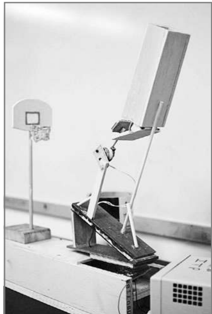
FIGURE 6-13 Using a rotary solenoid to launch ping-pong balls (CC-BY-NC-SA image used with permission from Greg Borenstein)
