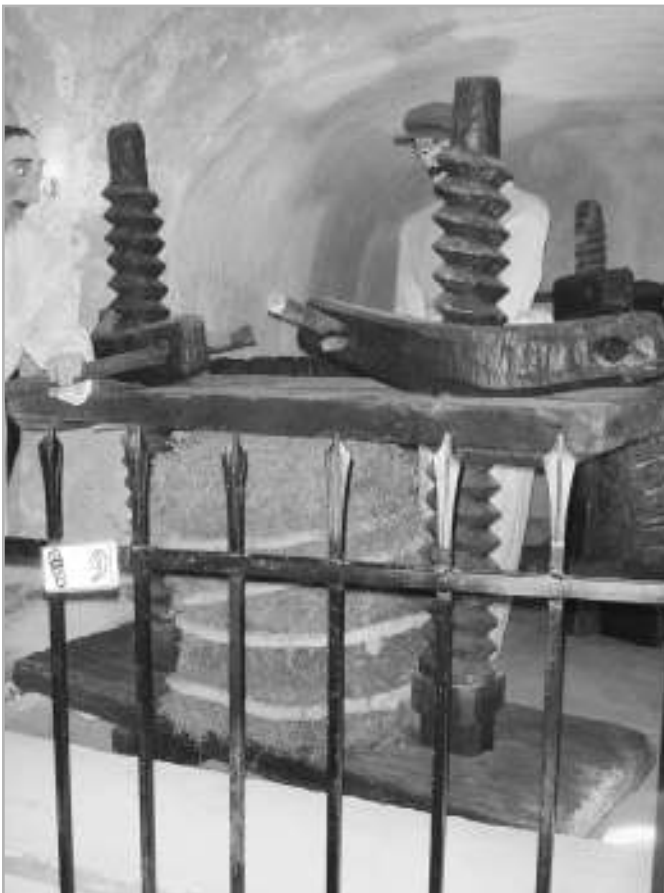
FIGURE 7-42 A diorama in a winery museum shows wooden power screws that were used to press the grapes.
