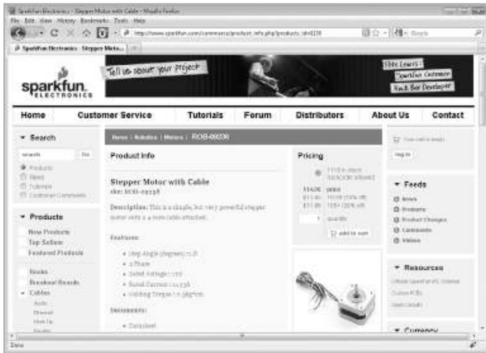
FIGURE 6-11 Features of SparkFun's ROB-09238 stepper motor
