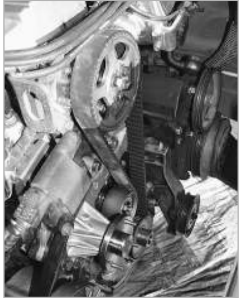
FIGURE 1-10 Timing belt on the engine of a car as a closed pulley system
