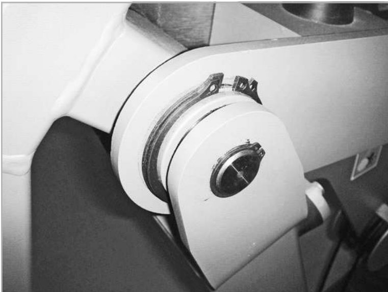
FIGURE 3-10 Retaining rings on gym equipment keep the shaft of a pivoting joint in place.
