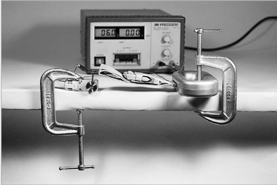
FIGURE 4-14 Measuring motor torque
