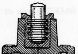
1282. COLLAR BEARING AND STEP for a vertical shaft. The thrust sleeve of bronze is split and should have a key to prevent rotation.
