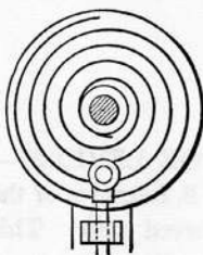
1081. SPIRAL-GROOVED FACE PLATE, for feed motion. Obsolete; but useful for irregular motion, in which the spiral grooves may be wavy or zigzag.
