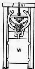
1457. RELEASING GRIP of a pile-driving machine. The bow ends of the grip are compressed when they reach the slot B in the frame and cast off the ram W. The springs between the bowed handles of the grip close the jaws to pick up the ram.
