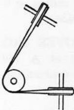
86. BELTING TO A SHAFT AT ANY ANGLE.— The two idler pulleys must be placed on a shaft at right angles to the driving and driven shafts, with their peripheries at the central line from centres from the driving and driven pulleys.
