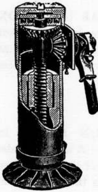
1586. BALL-BEARING SCREW JACK.— The balls run in grooves between the bearing plates.
