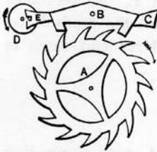
1184. LEVER ESCAPEMENT.—The anchor pallet B is attached to the lever C E, at the end E of which is a notch to receive the pin in the balance-wheel disc D. The impulse is given to the balance wheel at the middle of its oscillation by the escape of the teeth from the stop surface to the impulse planes of the pallets.
