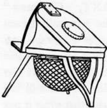
625. FOOT BELLOWS, for a blowpipe. A spring raises the top of the bellows. The rubber bag is confined to the netting to prevent bursting. The step at the left is for the foot.
