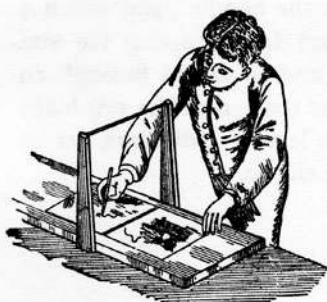
1531f. REFLECTING DRAWING BOARD.—A vertical plate of glass in a frame on a drawing board. The picture on one side and a plain sheet of paper on the other side of the glass. On looking into the glass on one side the picture is plainly projected on the other, and can be readily traced with a pencil.
