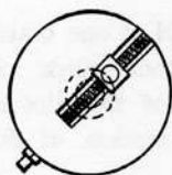
1124. VARIABLE CRANK THROW by a movable pin block in a slotted face plate and transverse screw.
