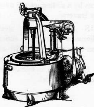
1145a. HYDRO - EXTRACTOR, showing method of belting with adjustable idler and cone pulleys.
