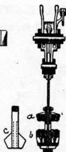
1599. CABLE GRIP FOR STREET RAILWAYS.— a , b , grip jaws and blocks; c , pull-up to throw the cable out of the jaws; d , d , frame plates; e , grip plate connected to b , and operated by the bell crank levers g , g ; f , f , pull-up attached to frame and disengaging pieces c , c .
