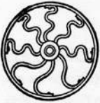
851. SPRING WHEEL.—Two forms of curved spring spokes and spring rim.
