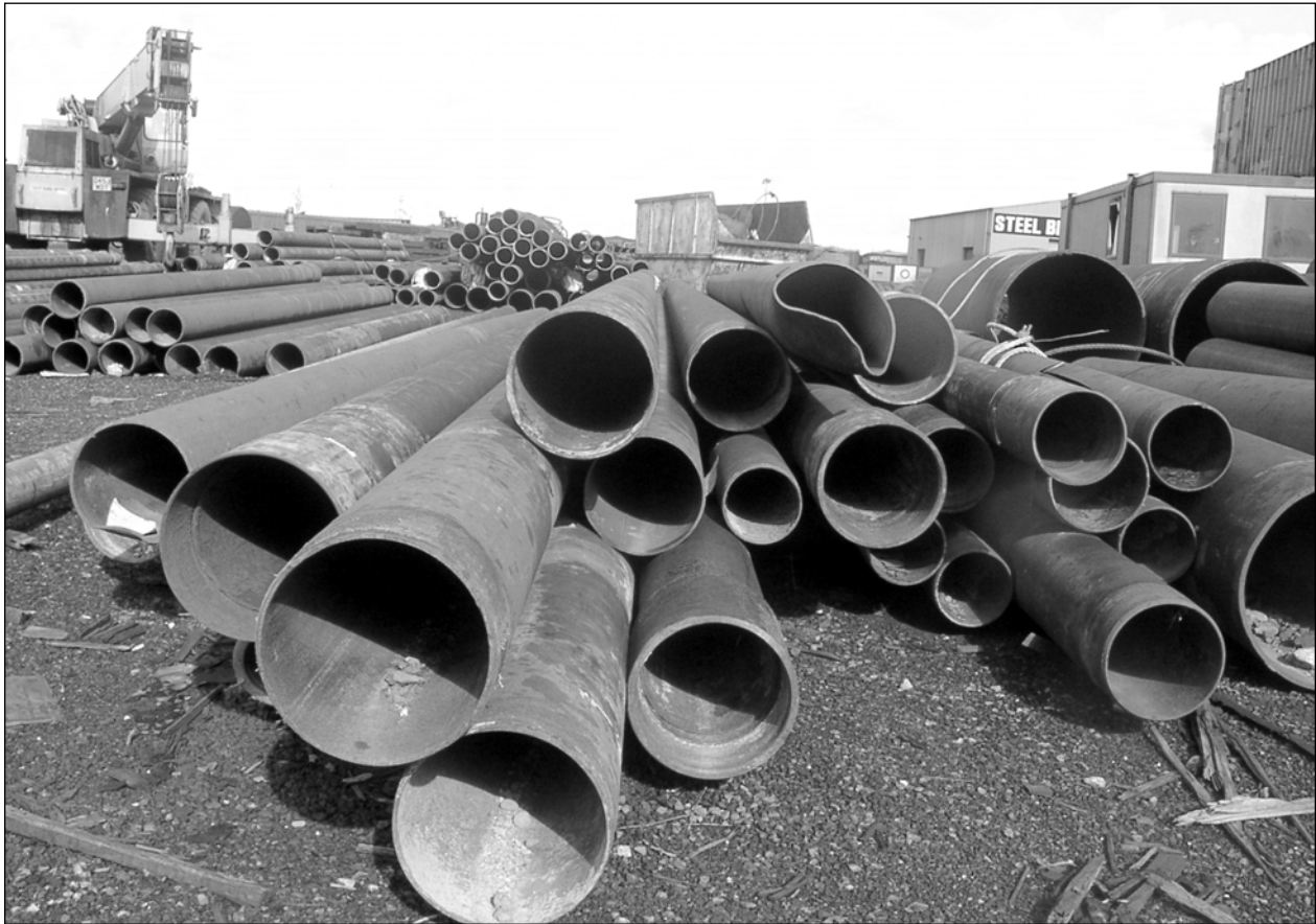
Figure 4.2 Reclaimed steel pipes are refurbished by the firm Greenpiles and used to form piles for foundations
