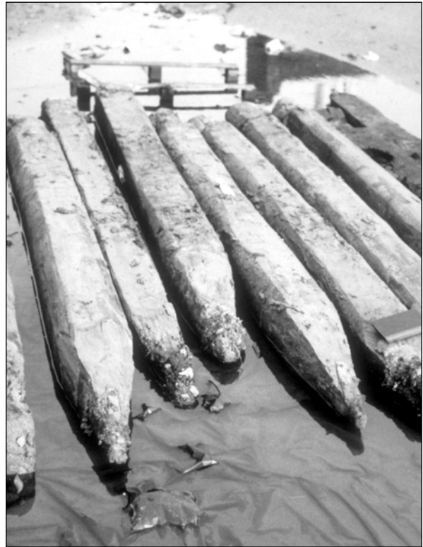
Figure 4.5 Several timber piles that would not be needed were extracted, inspected and found to be in excellent condition
