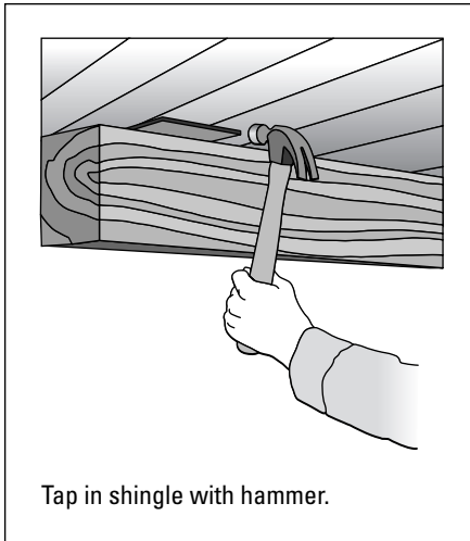
Figure 4-8: Tapping in a shingle with a hammer.
