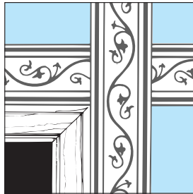
A. Apply a horizontal border and lay a vertical border over it. (Steps 1 and 2)
