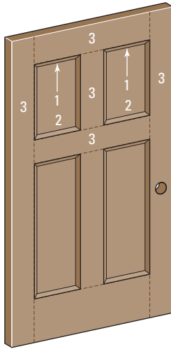
Figure 3-3: Paint the top pair of door panels first, then the wood around them.
