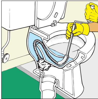
Figure 5-2: Using a toilet auger.
