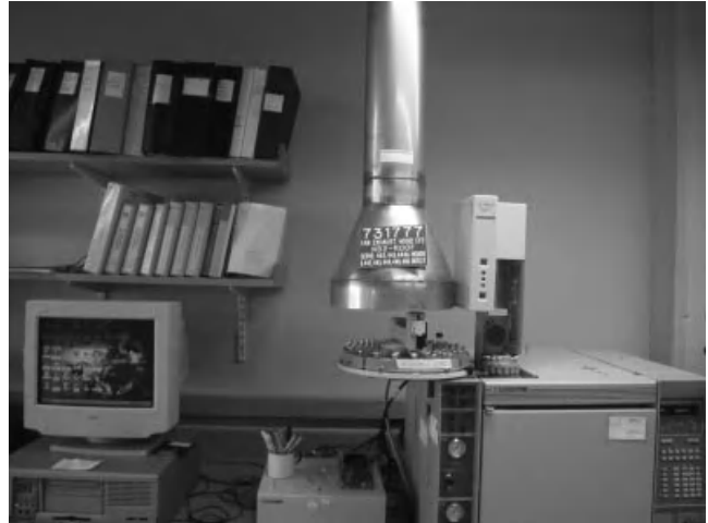
FIGURE 32-7. View of a capture hood in a physics laboratory.
