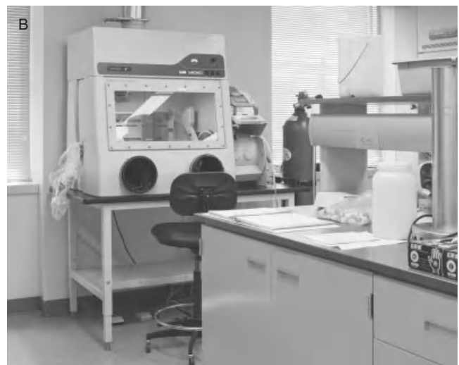
FIGURE 32-4. A. Glovebox: Section. (Approximate percentages shown for descriptive purposes only.) B. Glovebox in a laboratory setting.
