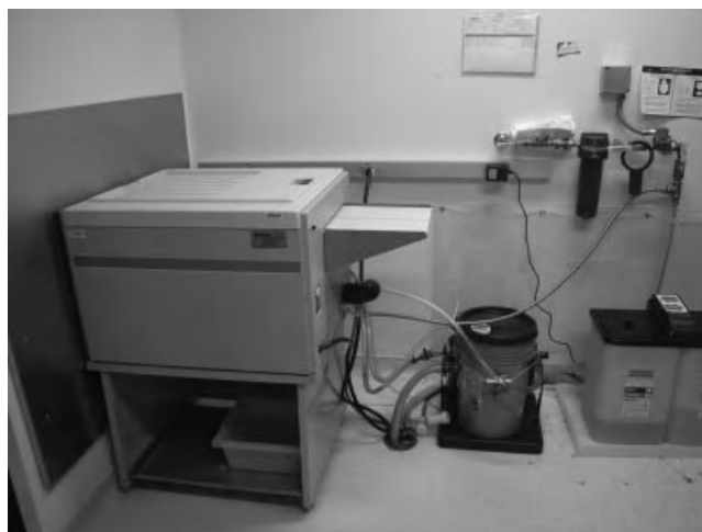
FIGURE 25-4. X-O-Mat with silver recovery system.
