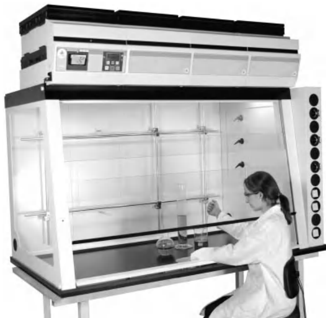
FIGURE 32-10. Ductless fume hood. (Courtesy of Erlab Inc., Rowley, MA.)
