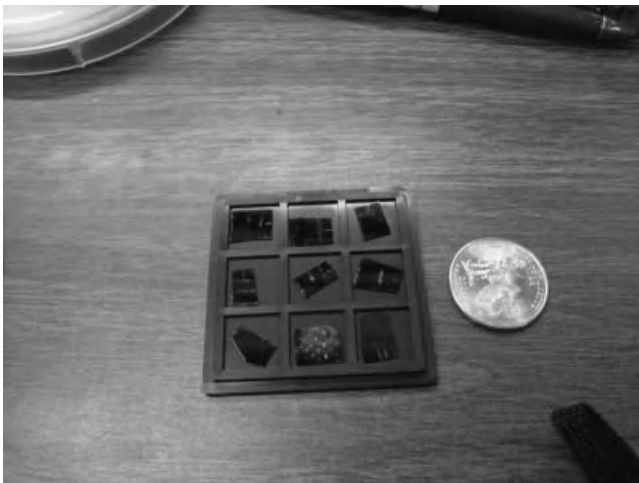
FIGURE 7-2. Carbon nanotubes grown on a substrate.
