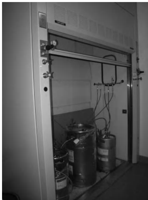
FIGURE 16-7B. Back view of chemical fume hood with solvent-dispensing device.
