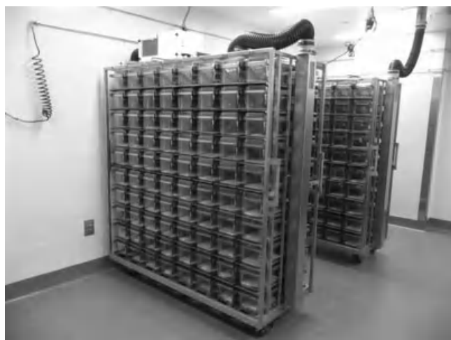
FIGURE 22-2. View of ventilated cage rack.
