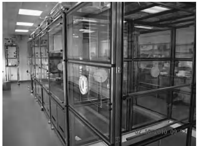
FIGURE 7-4. Example of a large enclosure hood used to control nanoparticles.
