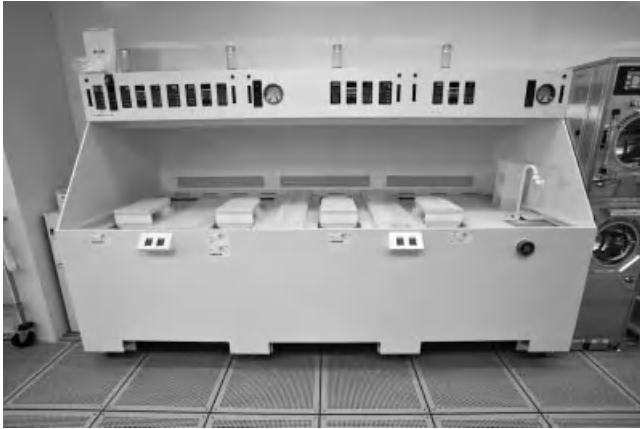
FIGURE 23-8. View of a microelectronics vented wet workstation.
