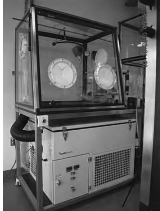
FIGURE 7-3. Example of a standard-sized enclosure hood used to control nanoparticles.
