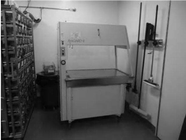
FIGURE 22-1. View of ventilated animal cage changing station.
