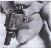
This unusual .22-caliber firing device was made by taking the detonator top from an inert grenade, drilling out the primer area, and inserting a .22 round. The firing pin is spring-loaded. (Courtesy of Oceanside, California, Police Department.)
