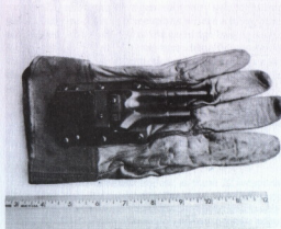
A production model of the ONI fist gun as used during World War II. (Courtesy of Maj. Richard Keogh.)
