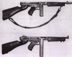
At top, a VC Thompson copy with original sling. The bottom item is the real thing. In the copy, note the imprecise cut on the cocking slot, the missing fin on the aluminum compensator, plus other assorted M1A1, M1928A1, and homemade parts. (Courtesy of Fred Rexer, Jr.)
