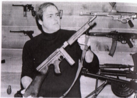
Fred Rexer, Jr., displays his VC-made Thompson SMG copy, captured in Vietnam. The weapon has no rear sight. (Courtesy of Fred Rexer, Jr.)
