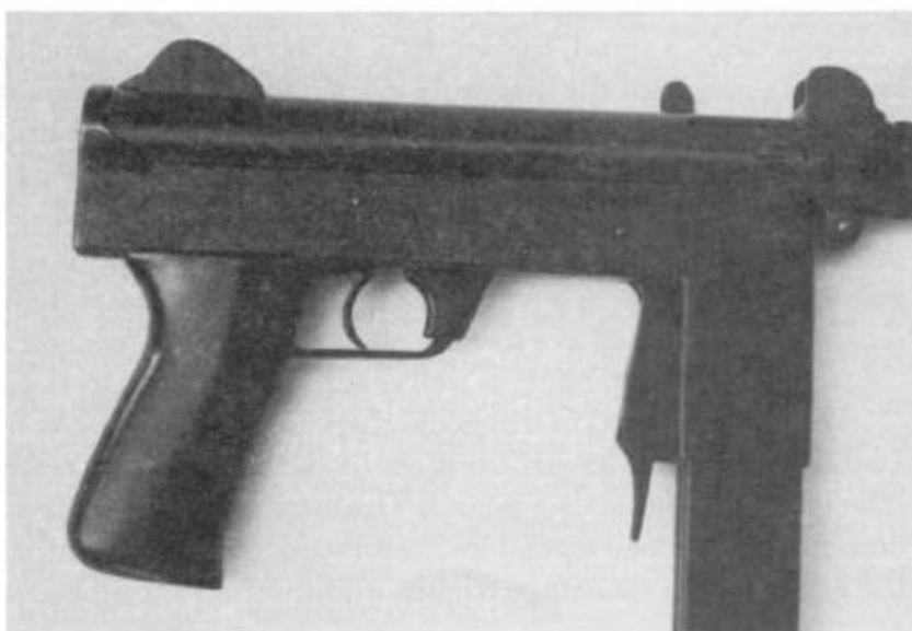
Above: Removable trigger assembly of the MP83A1.
