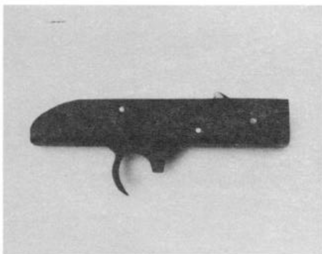
Above: Removable trigger assembly of the MP83A1.
