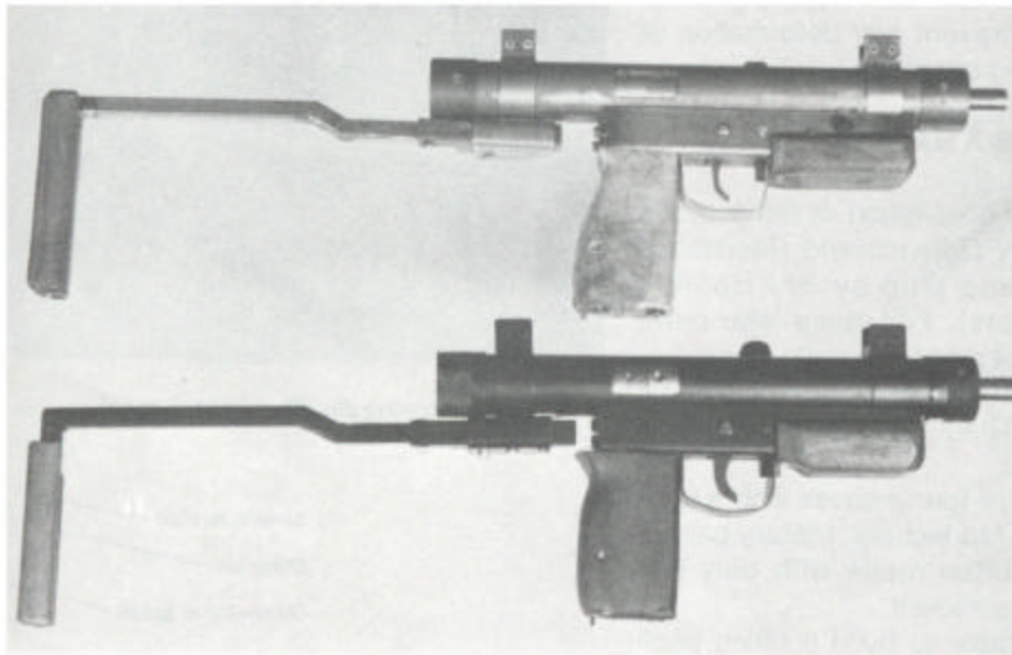
Imvised prototype, including plugs without threading, welded bracket, and plastic pistol grip (top) compared with the standard prototype (bottom).
