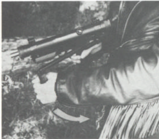
Unfolding the stock.
