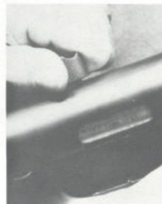
Rotating the bolt handle.
