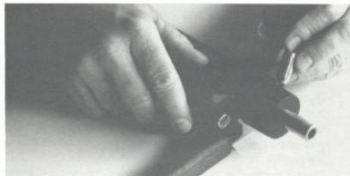
Use the tip of a bullet to release the front plug.
