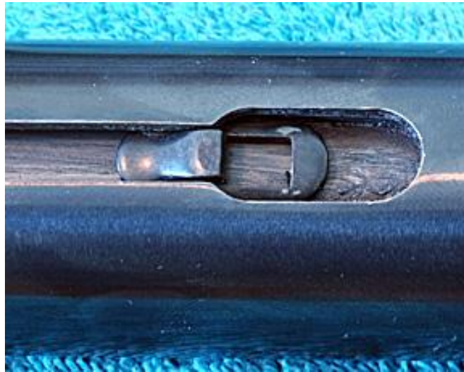
When the sliding cocking link is installed, it keeps the piston from rotating. It's also lubed with moly.
