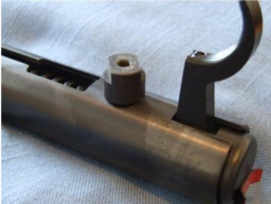
A large vertical bolt holds the FWB 124 together
