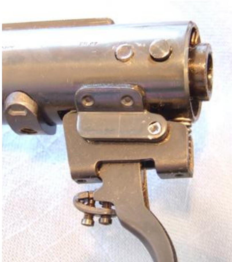
This vintage Diana 27 has two pins at the very rear of the spring tube. Modern pins are farther forward than this.
