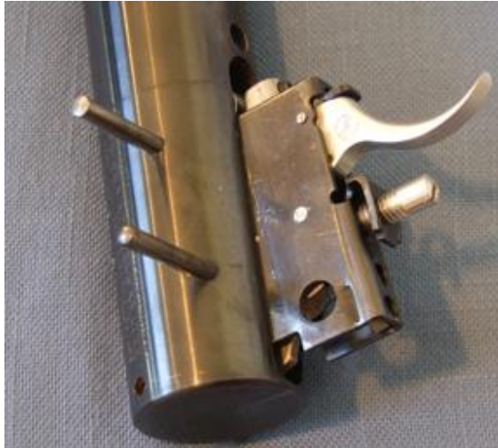
Two pins are drifted out and the Rekord trigger is free.
