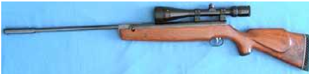
My R1 has a plain walnut stock, a Vortec muzzlebrake and a Bushnell Trophy 6-18x in Leapers Accushot medium rings. The low-power tune makes it very enjoyable.
