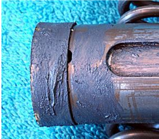
The piston seal is coated uniformly with a thin layer of moly grease. Note that I also coated the front part of the piston body, as well as the cocking slot.
