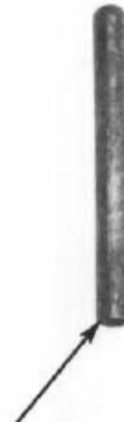
one of the pins used to retain the ramrod loops, fore loop and muzzle cap in position
