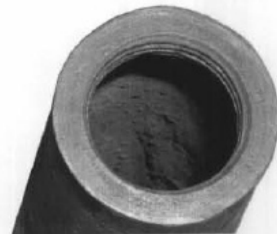
Threaded insert, note there are only three threads in the reservoir insert
