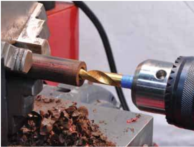
1. Mark the drill depth on the drill bit using some tape.
