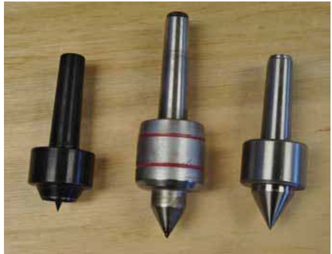
5. Live centers: From the left: A center with a sharp point that comes standard with many lathes. This type is not usable for pen turning; a 60-degree live center; the compact 60-degree live center I use on my pen lathes wastes less space than the larger center in the middle.
