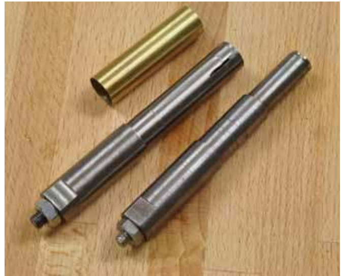
6. The finished mandrel is on the left. A stepped expansion mandrel that allows more show on the cap is on the right.
