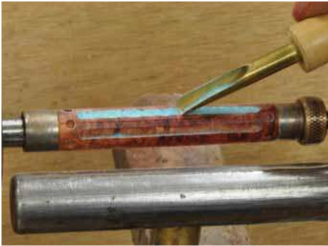
4. The grooves are filled level with crushed turquoise.
