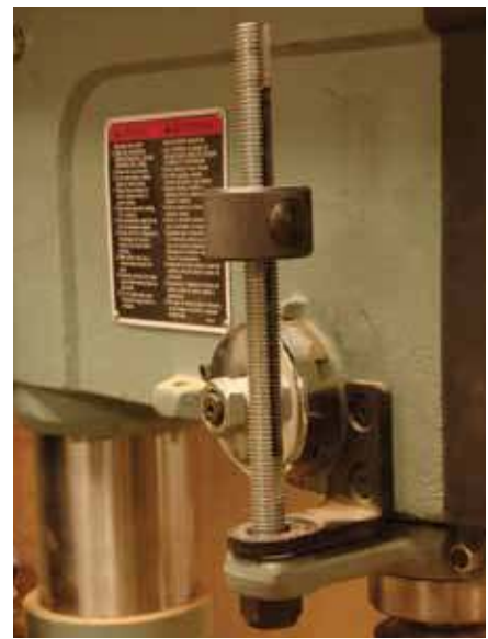
3. A rod-type depth stop has some advantages.
