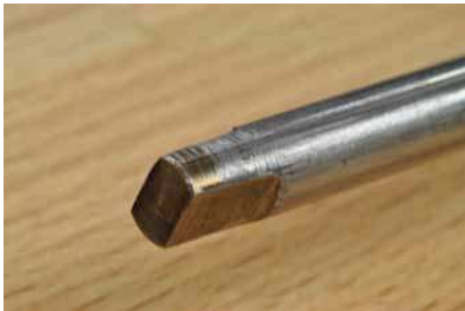
2. The other end of the mandrel is ground to accept a wrench.
