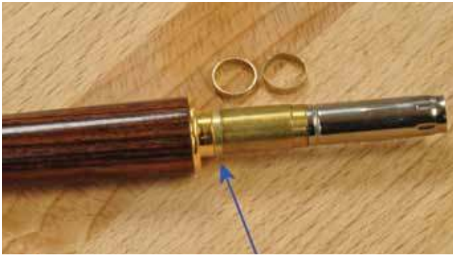
12. A small brass spacer moves the transmission up a little to let a Parker-style refill tip retract fully.
