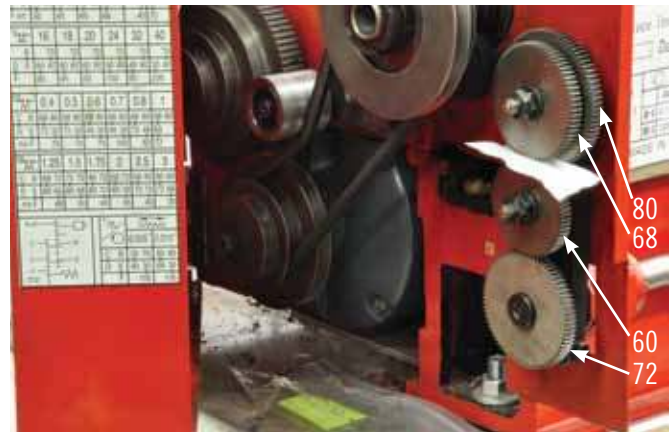
4. Change gears are used to set up the metric thread on the imperial lathe. The temporary piece of typing paper between the gears is a convenient way to set the proper clearance.
