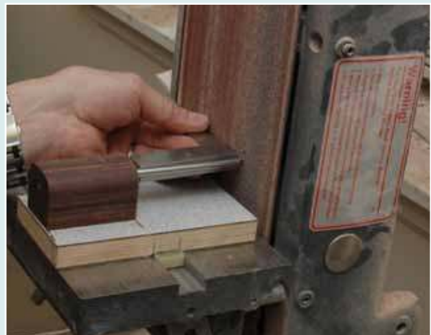
Before the runner is fixed in place carefully square the rod horizontally.
