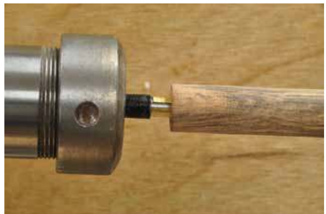
5. A brass shim may be needed if the hole is too large.
