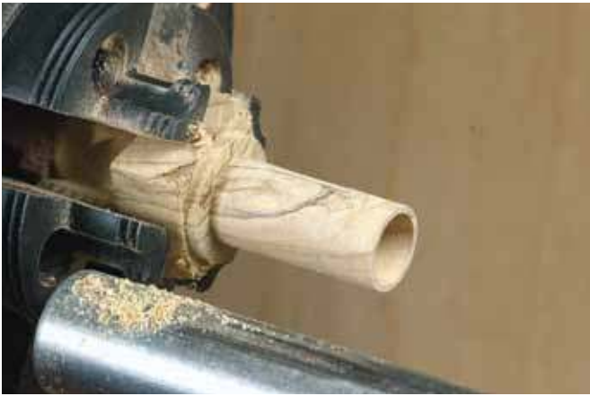
13. The finial needs to be drilled to make room for the nib.
