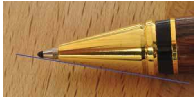
8. Proper ballpoint tip extension.
