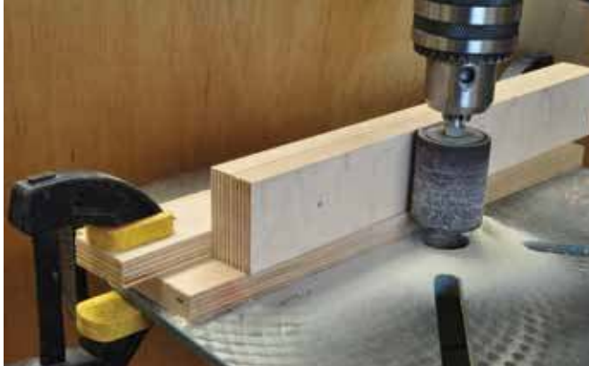
6. The fence is trued to the drum which may not be running like a perfect cylinder.
