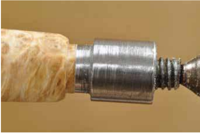
6. Use a thin parting tool to make a short tenon down to the smaller bushing diameter.
