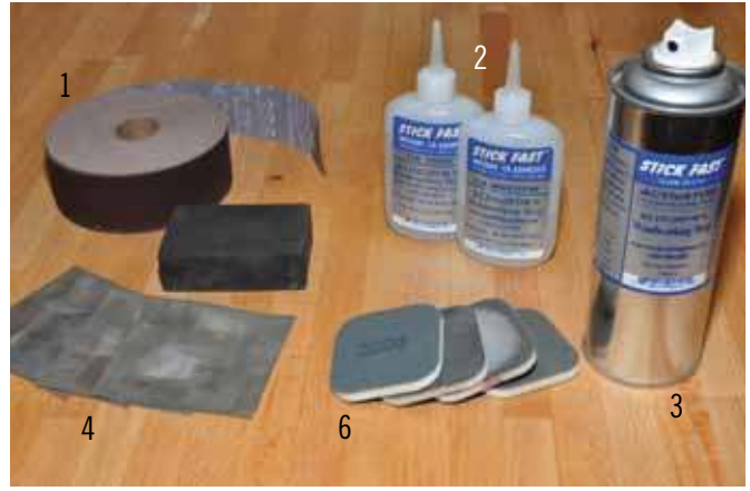
8. Supply for a CA finish: (1) sand paper, (2) CA thin and medium, (3) accelerator, (4) micro-mesh sheets with (5) rubber backing block or (6) micro-mesh pads.
