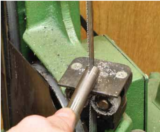
5. A relatively inexpensive band saw comes in handy to cut the slot freehand.
