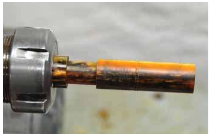
12. A test fit verifies a good thread. The carriage should remain engaged to the lead screw.
