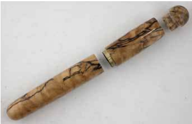
15. The turned parts for this pen. From left: Main barrel, cap barrel with appropriate tenon for centerband, and cap finial with tenon to fit inside cap barrel tube.
