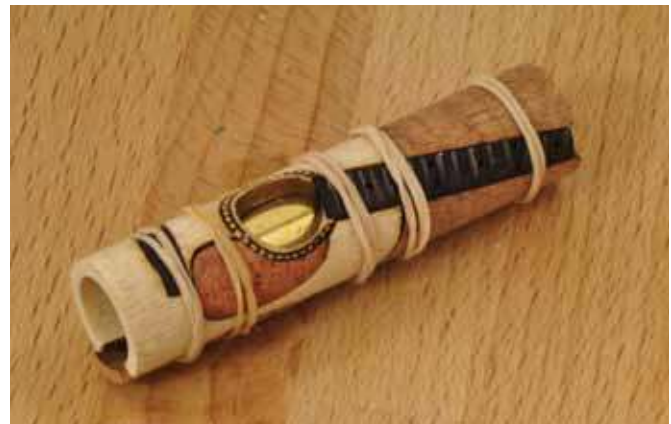
2. After assembly on a temporary brass tube, parts are held together by small rubber bands.
