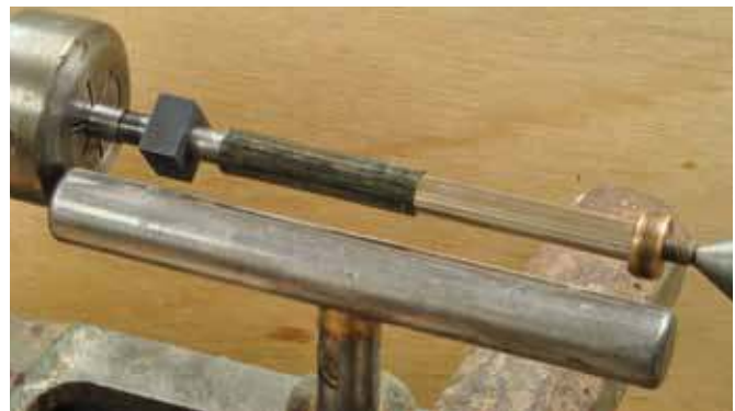
4. Use filler pieces to mount a single center band on a mandrel.
