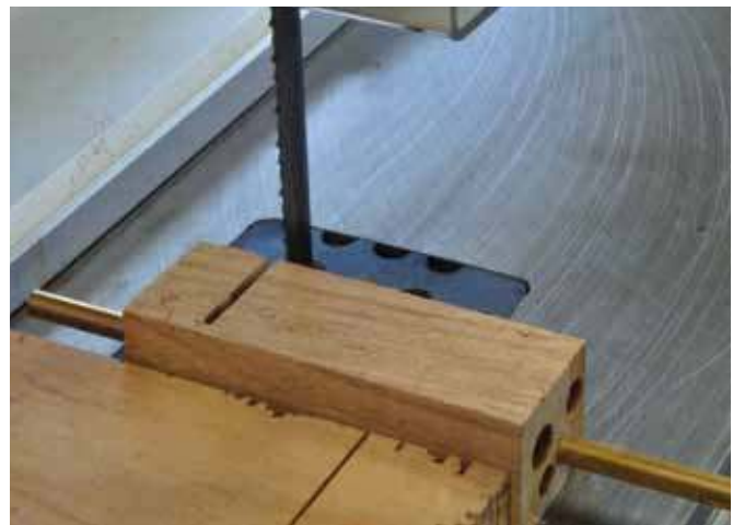
4. A wood block with a hole for the brass tube prevents the tube from collapsing when sawn on the band saw.
