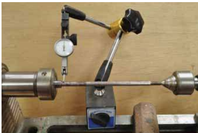
2. A dial indicator or a dial test indicator (shown) can be used to measure runout on a mandrel.
