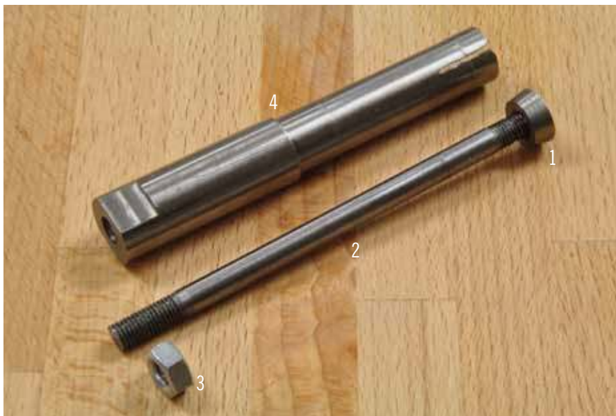
1. Anatomy of an expansion mandrel. (1) tapered expansion plug, (2) draw bar, (3) nut, (4) main body with slotted end.
