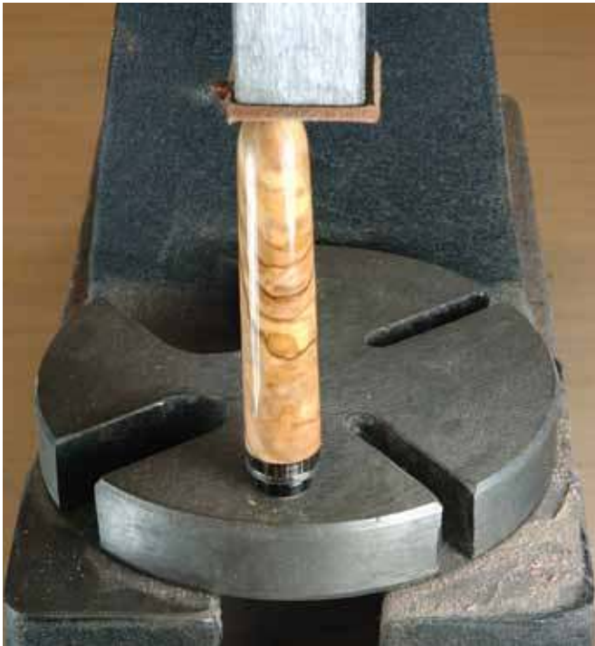
9. Assemble with care, excessive pressure can ruin the finish at the end of the barrel.
