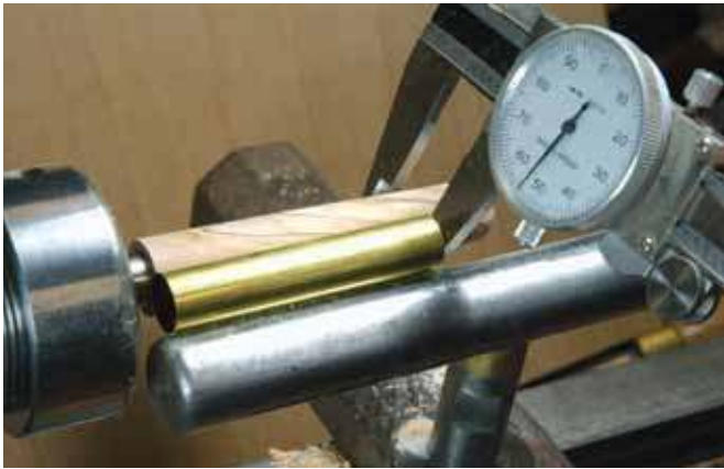
7. Be mindful of the end of the internal brass tube and use calipers to be certain there is sufficient wall thickness at that weak spot.
