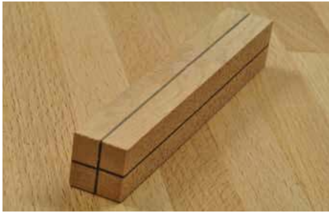
1. Two black veneer strips at right angles sandwiched in a maple blank create the starting blank.
