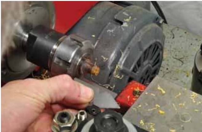
5. A fish-tail gauge is used to set the thread cutter square to the lathe. When there is no long, straight section of the workpiece available, sight against the lathe bed.
