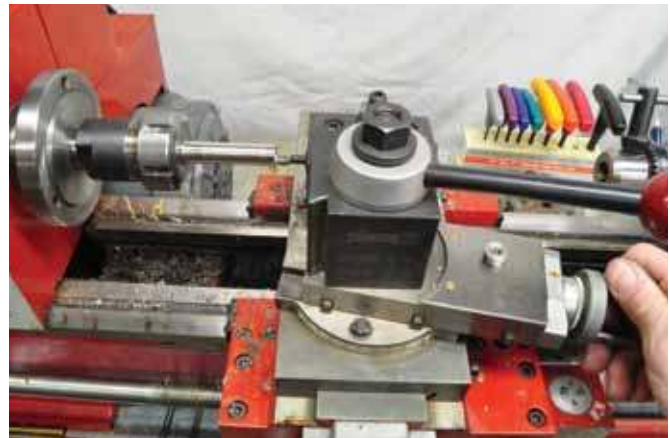
4. A boring bar cuts the internal taper with the same compound setting.
