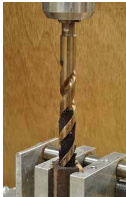
2. Keep an eye on the chips. When they start packing into the flutes heat and pressure can crack blanks.
