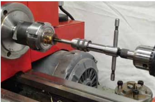
3. A tap guide is used to keep the tap straight on a lathe.
