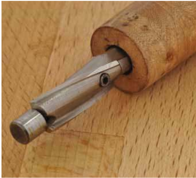
5. A piloted counterbore can be used to cut a recess into the center band to create an overlap on the lower barrel.
