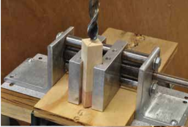
1. Glue a wasteblock to the ivory to increase the safety margin when drilling.
