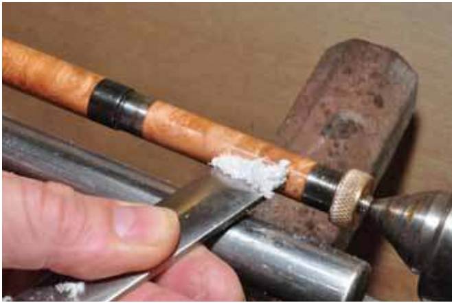
7. Scrape the cured CA with a skew laid flat on the tool rest.
