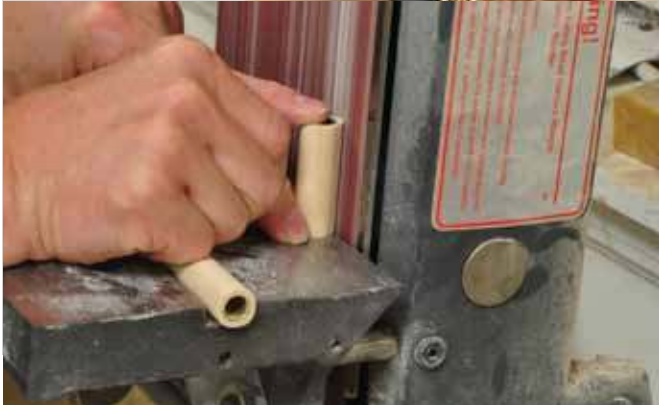
2. Knock the corners off on the belt sander to avoid stress to the barrels during roughing cuts.
