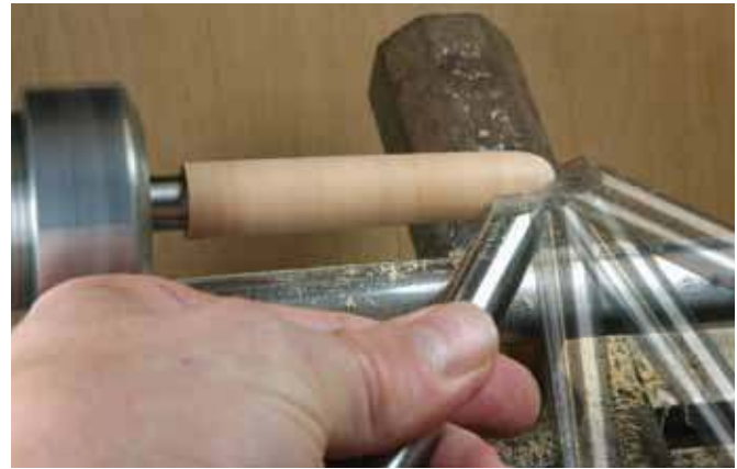
8. A pyramid tool makes it easy to round over the end of the barrel.
