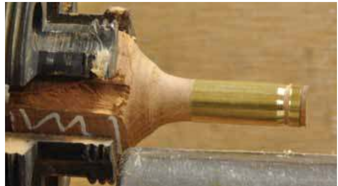
11. Turn a dowel to fit inside a brass tube. Proceed to part off a narrow ring.
