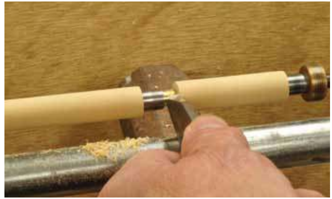
6. Use a parting tool to cut a tenon down to the brass tube for an integrated center band.
