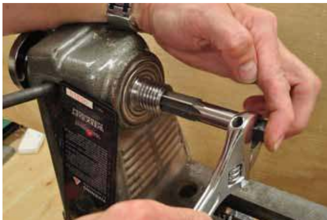
1. Use a Morse-taper reamer to clean up a damaged Morse-taper that has internal marks and burrs.
