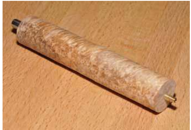
4. Test the fit and look for the proper protrusion. A few threads need to be exposed to secure the tip.
