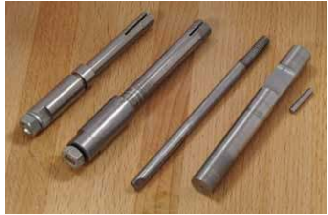
6. Mandrel options for closed end pens. From the left: commercial expansion mandrel, a shopmade expansion mandrel, a universal mandrel tap, and a pin chuck.
