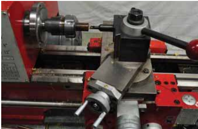
11. The interior threading tool ready for use. Notice the compound is swung 29.5 degrees to the left for the proper feed.
