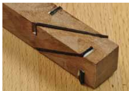
9. Making partial cuts and filling them with wood strips creates an interesting effect.
