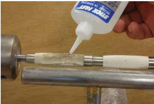
3. Fill porous sections of the antler with thin, followed by medium CA.
