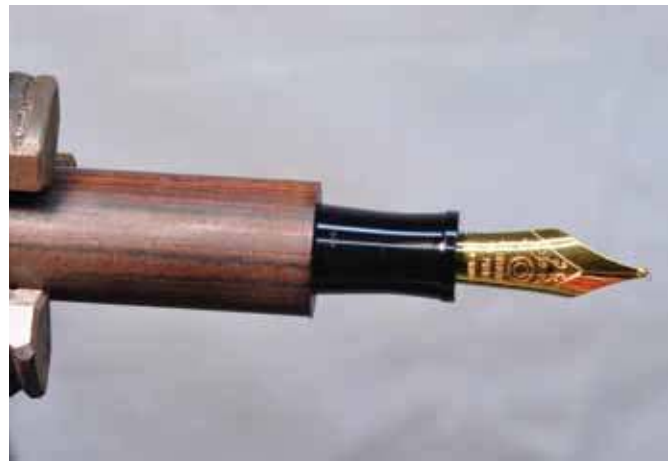
4. Test fit the grip section; there should be no gap.
