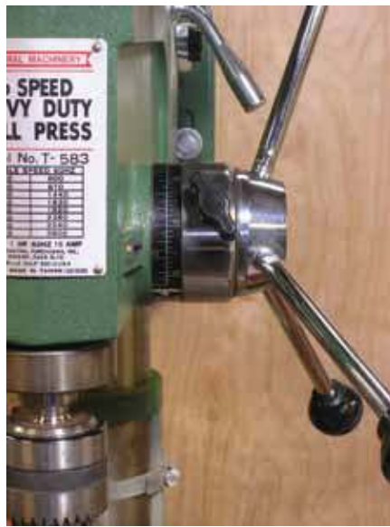
2. A rotating collar depth stop allows you to set the drill depth so you can avoid having the drill bit exit the blank.
