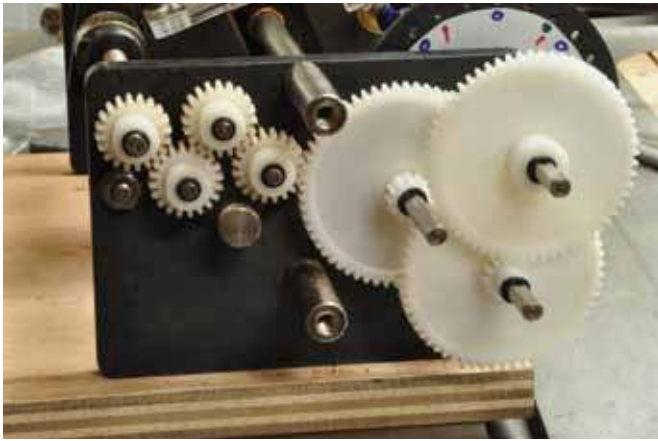
1. A gearing setup for a slow twist. Always arranged from the smallest cog to the largest.
