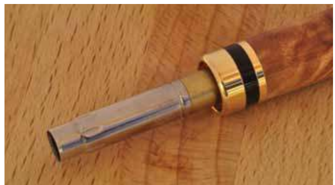
20. Before assembling 8 mm pens reverse the transmission and test the fit in the barrel. It has to slide freely.
