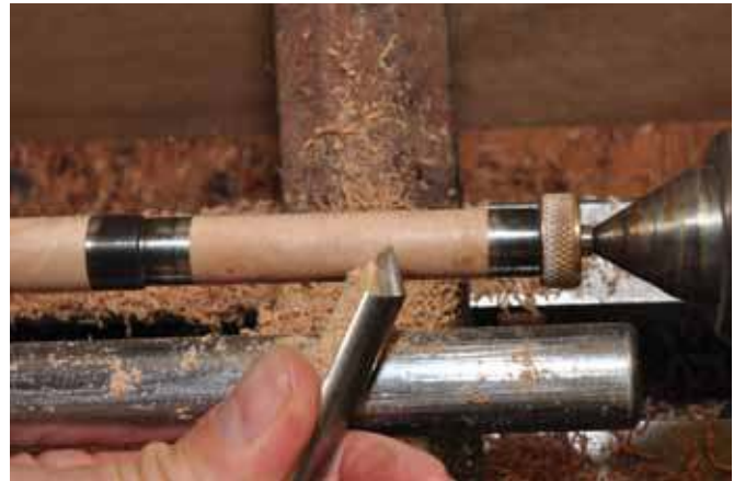
4. Cutting with the side of the fingernail-ground spindle gouge lets you achieve a fine finish that requires little sanding.
