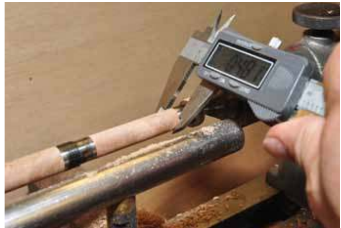
5. Use calipers to check the turned diameter rather than relying on the bushings which will wear over time.
