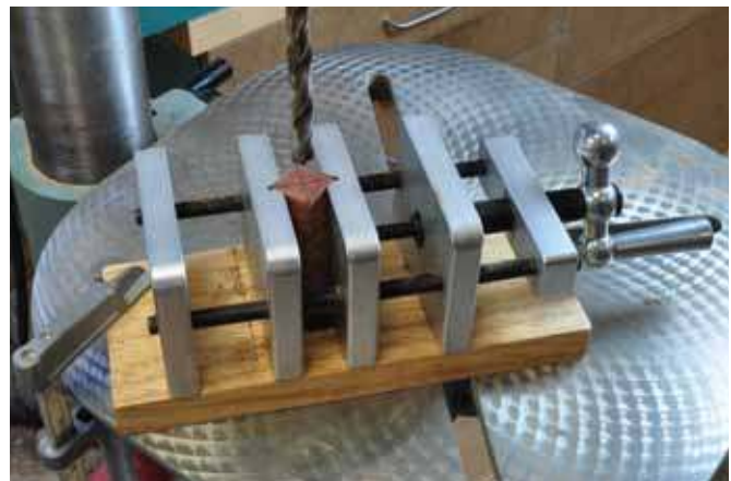
8. A drill jig sold by Penn State Industries holds the blank securely. A newer version of this jig has a replaceable waste block which is a nice feature.
