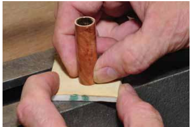
10. Removing glue burr.
