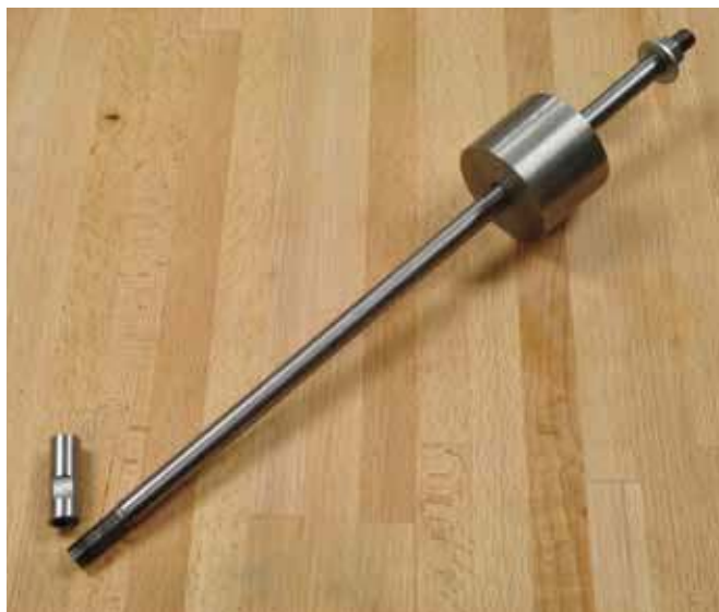
19. A homemade slide hammer allows disassembly of closed end barrels. Add adapters as needed for other pens.
