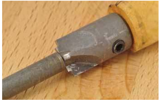
2. The recess for a clip is cut using a pen mill modified on a grinder.
