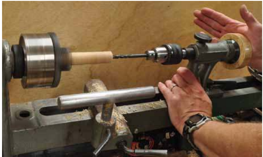
3. After the hole is drilled about 2" deep, use the ram to loosen the tailstock and advance it as a unit.
