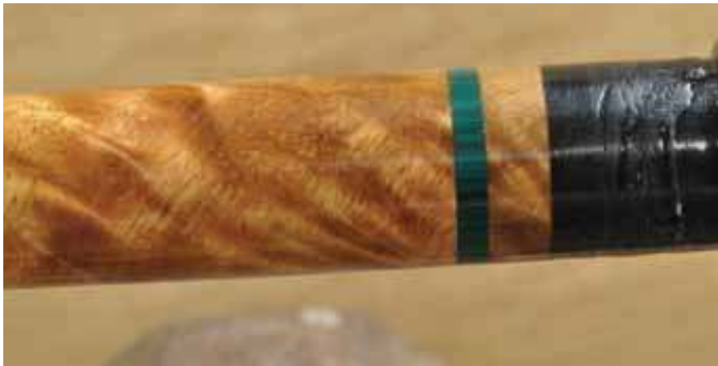
5. The repair used a cutoff from the same piece of wood and it looks like it belongs there.
