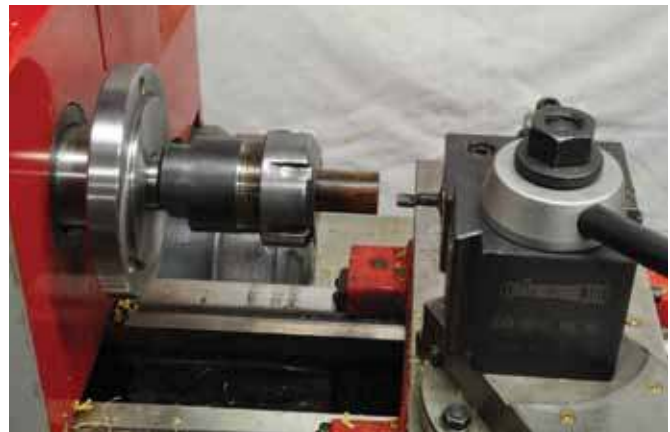
14. A boring bar is used to cut a recess for the center band fitting.
