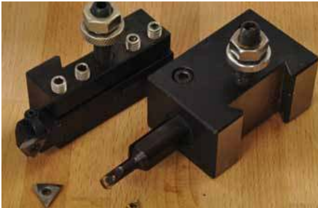
1. Threading tools. The interior tool can be used for exterior threads also, but working on the backside of the lathe.
