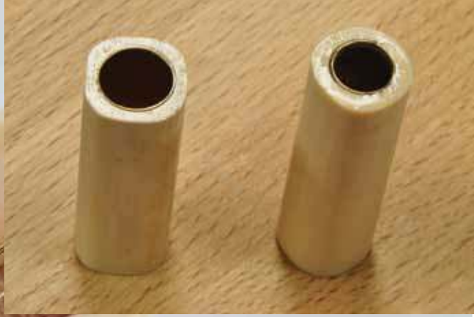
3. Flood the barrel ends with CA before turning.
