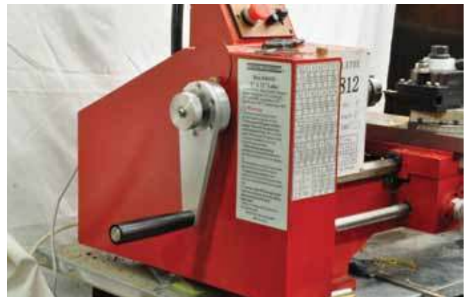
2. A hand crank is very useful for threading, unless the lathe has extremely low gearing.
