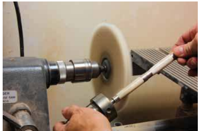
4. A polishing wheel lets you achieve a great sheen directly without the need for a finish.
