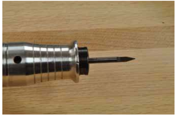
2. An engraving bit has a very sharp point.
