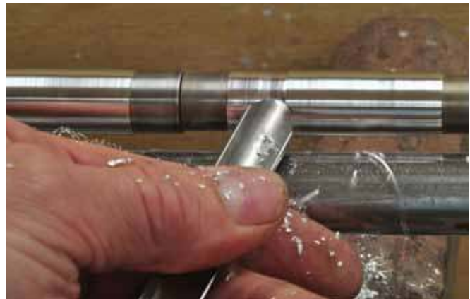
3. The \frac{1}{2} " gouge works quickly on aluminum.
