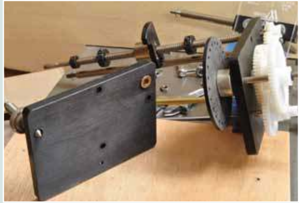
5. Disassembling the Pen Wizard to convert it to a mirror image for better right-handed operations.
