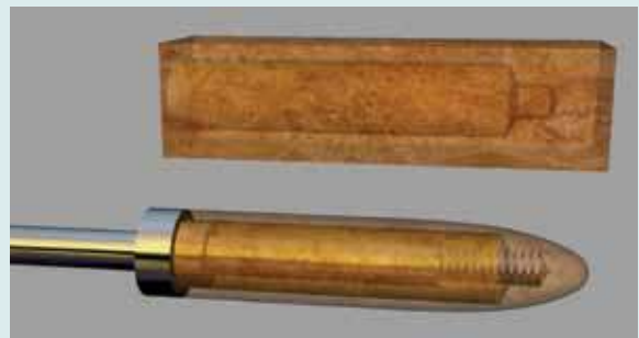
D. In use, a standard bushing supports the open end of the barrel.
