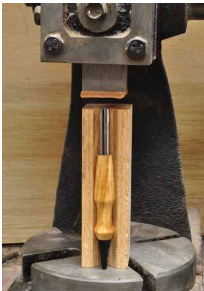
1. A simple gauge for assembling slimline pens.
