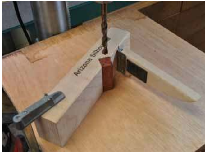
6. This simple drill jig is no longer commercially made but it is easy to make it yourself and it performs excellently.
