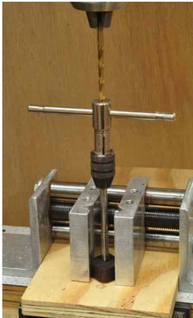
9. The drill bit guides the tap to keep it vertical.
