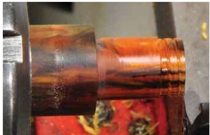
8. The first groove of a triple-lead thread is cut.
