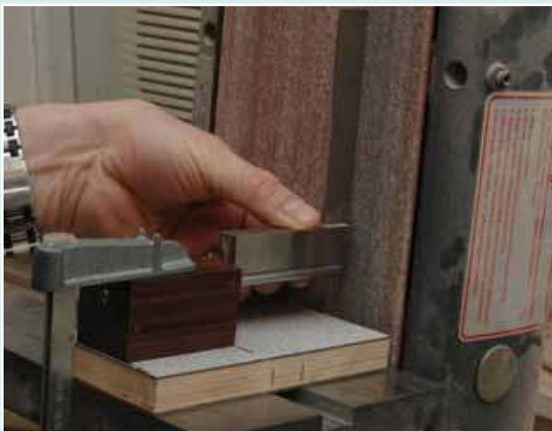
The rod must be perfectly square to the belt sander. Check before attaching the block to the base.
