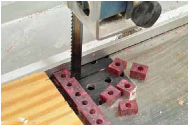
1. Drill holes in a strip of material and use the band saw to separate the material into squares.
