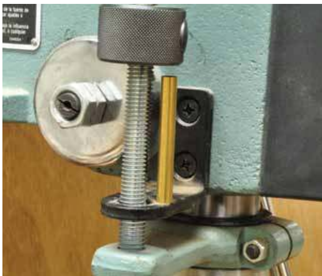
3. With the tip of the drill bit even with the top of the blank, use the brass tube to set the depth of the hole a little longer than the tube.
