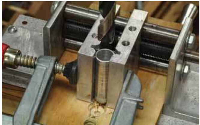
2. Drilling the cap barrel.
