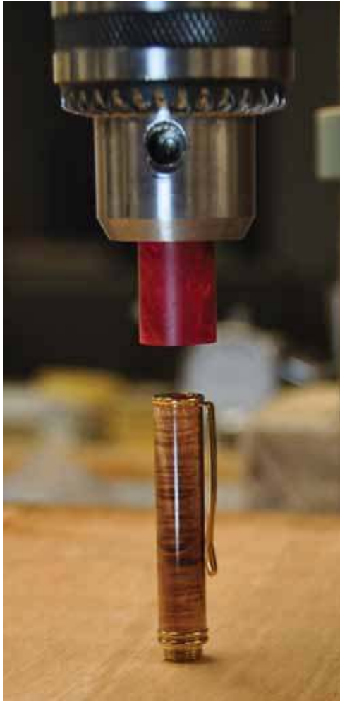
15. A little anvil turned from a cutoff converts the drill press into an assembly press.
