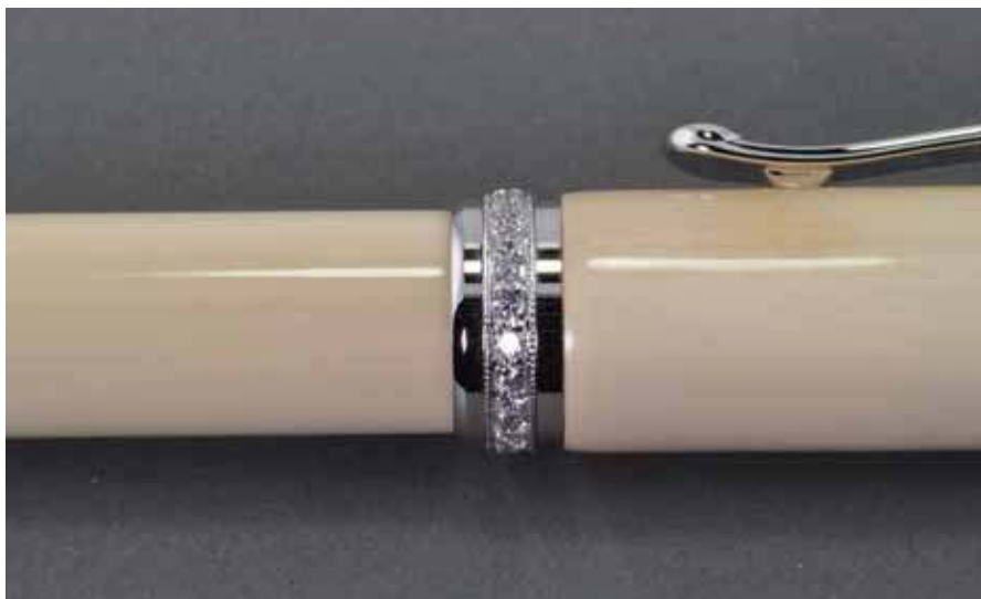
4. A barrel turned oversize and gently rounded over to the fittings is barely noticeable.
