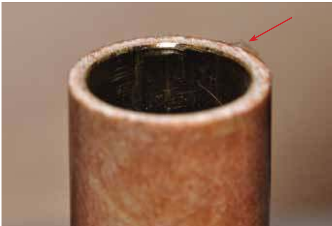
9. After taking the barrels off the lathe there is often some glue burr that must be removed.
