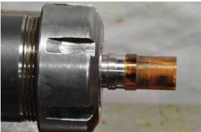
13. The center band fitting on a short shopmade mandrel.
