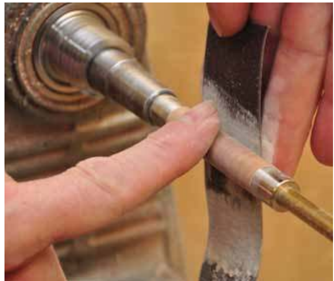
11. Hold the sand paper behind the blank to let the dust fall away.
