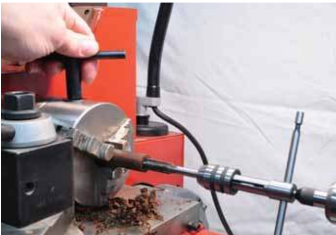
3. Use a tap guide in the drill chuck to keep the tap straight, and use the chuck key to hold the chuck while tapping.
