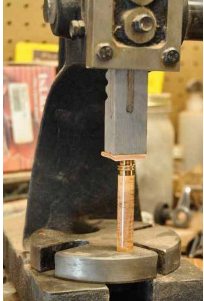
16. A small arbor press makes a great assembly tool.
