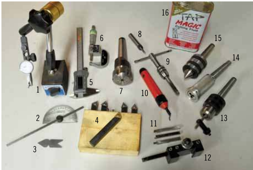
2. Lathe tooling: (1) dial test indicator with magnetic stand, (2) machinist's protractor, (3) fishtail gauge, (4) indexable tools, (5) calipers, (6) 0-1" micrometer, (7) collet chuck with ER32 collets, (8) tap center, (9) tap holder, (10) deburring tool, (11) HSS tools, (12) boring bar, (13) drill chuck for tailstock, (14) tailstock die holder, (15) revolving center, (16) cutting fluid.
