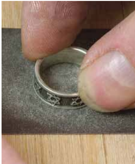
11. Sand one side of the silver ring flat so that it will fit flush.
