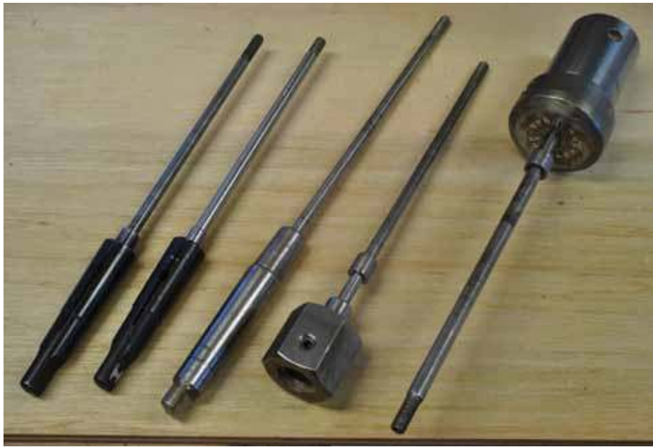
4. Pen mandrels, from left: “A” precision mandrel, “B” precision mandrel, standard pen mandrel in Morse-taper two, a specific mandrel for use on the Shopsmith, my usual setup, a mandrel-rod in a Beall collet chuck.
