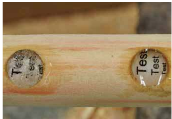
4. The test holes after filling. Epoxy on right, CA on left.
