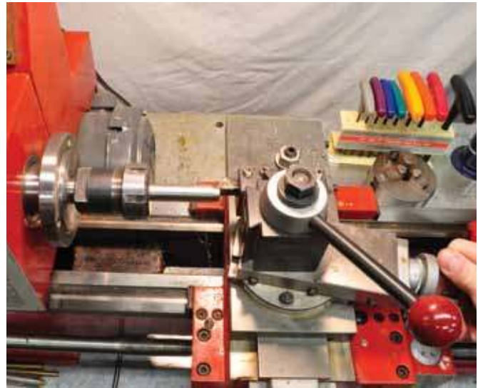
3. Run the lathe in reverse and work on the back of the workpiece to cut the taper with the compound.
