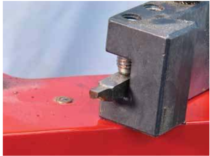
2. A specially ground tool bit for machining small recesses.
