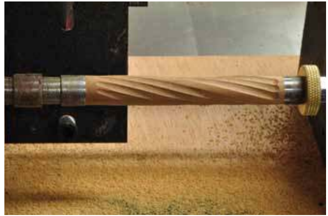
2. Test cuts are necessary to find the right settings.
