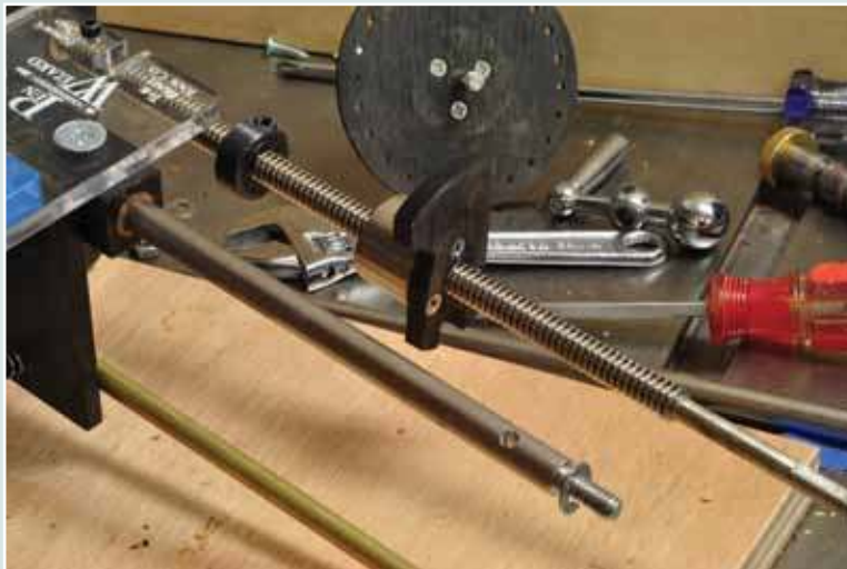
8. The Acme nut with the tool platform pusher also needs to be reversed so the "R" points forward.
