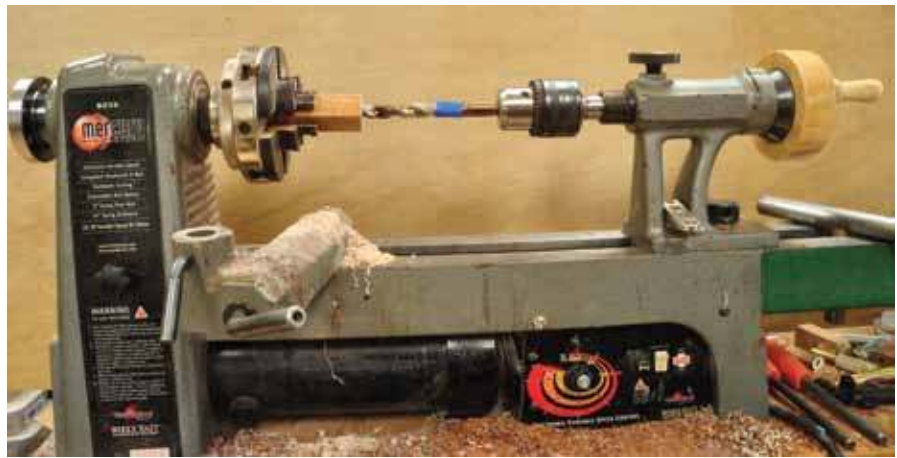
1. Drilling on the lathe using a four jaw chuck and a drill chuck in the tailstock.
