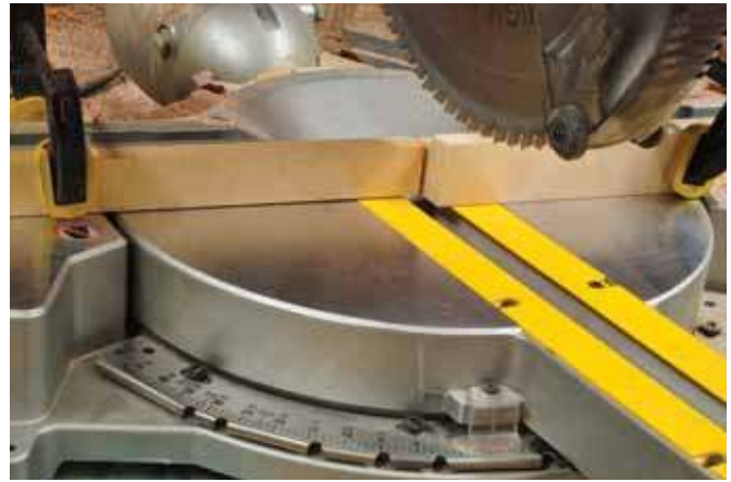
2. The chop saw needs an auxiliary fence and a stop-board.
