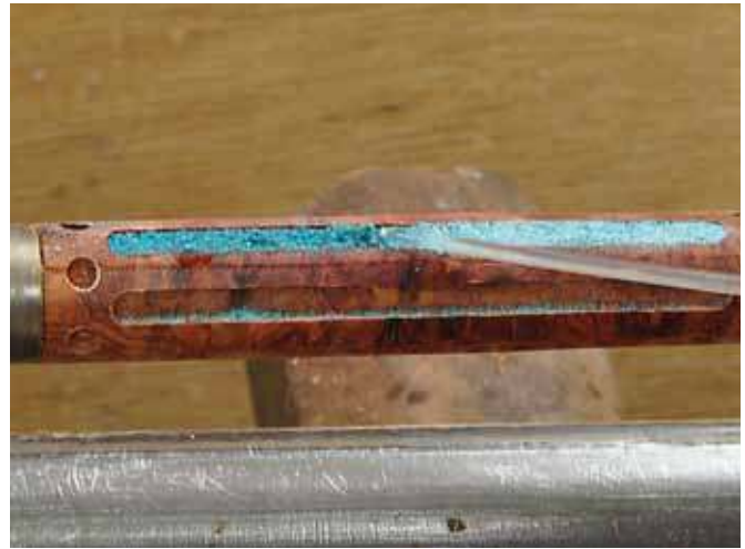
5. Let thin CA glue wick in carefully. The nozzle does not touch the stone.
