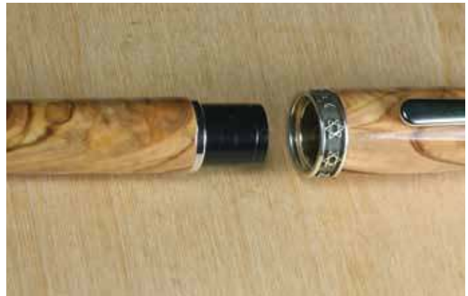
16. Mount the threads on the center coupling and epoxy them into the cap.
