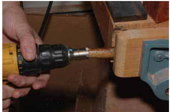
2. Using an electric drill with a pen mill to square up a pen barrel.
