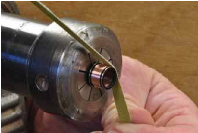
10. Sanding the fitting will allow it to slip into the brass tube and be glued in place.
