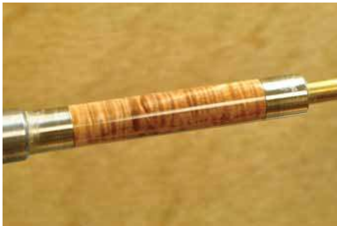
14. After applying Shellawax as a final finish, the blank should be allowed to cool on the lathe.
