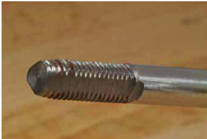
1. Three flats ground on an old pen mandrel turn it into a tap and effective mandrel for desk pens.
