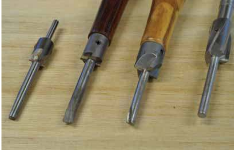
6. Various pen mills. From the left: a pen mill for use in a drill; a pen mill with a larger shaft for larger diameter brass tubes in a homemade handle; a pen mill with a standard shaft in a homemade handle, and a counterbore with a replaceable pilot adapted for pens.
