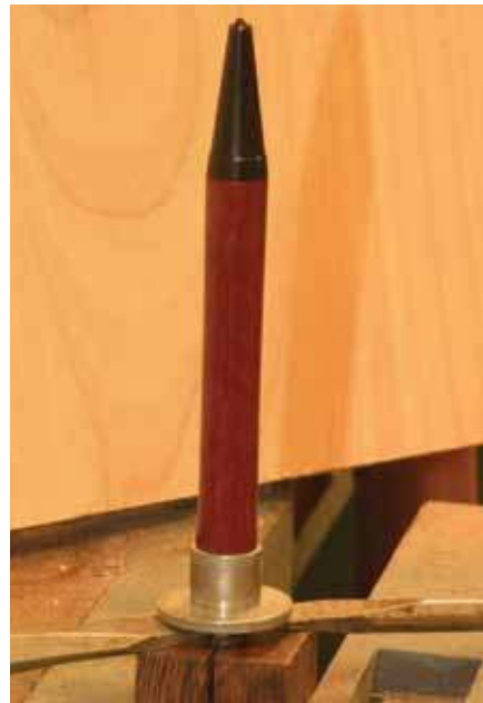
8. Proper ballpoint tip extension.
