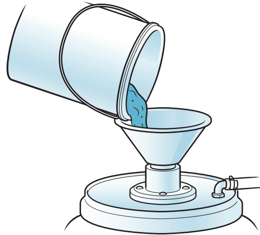
3. slurry poured into digester
