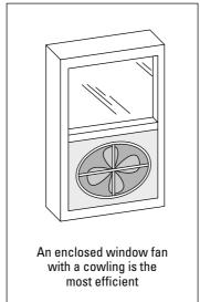
Figure 13-5: A cowling on a fan directs airflow and improves efficiency.
