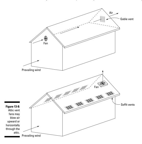
For the most efficient setup, place the fan at the apex of the roof, where the most heat collects due to the chimney effect. Note in the figure that the roof-top vent is on the downwind side of the house to complement the natural ventilation scheme from prevailing winds. The following steps explain what to do as you choose your ideal setup:
