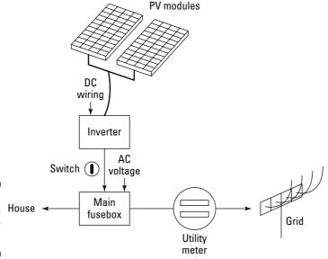
Figure 16-1: Solar intertie PV system.
