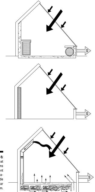
Figure 15-5: Storing heat maintains consistent temperatures inside a solar room.
