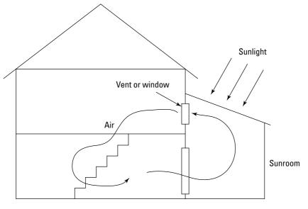
Vent fans can enhance the chimney effect. Solar-powered ceiling fans work well because they don't need to be hard-wired (no code problems or expenses associated with electricians), plus they work hardest when the sun is hottest, which is usually what you want.
