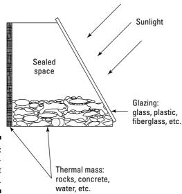
Figure 15-2: The greenhouse effect traps heat.
