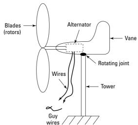
Figure 14-2: A wind turbine. And here are some drawbacks:
