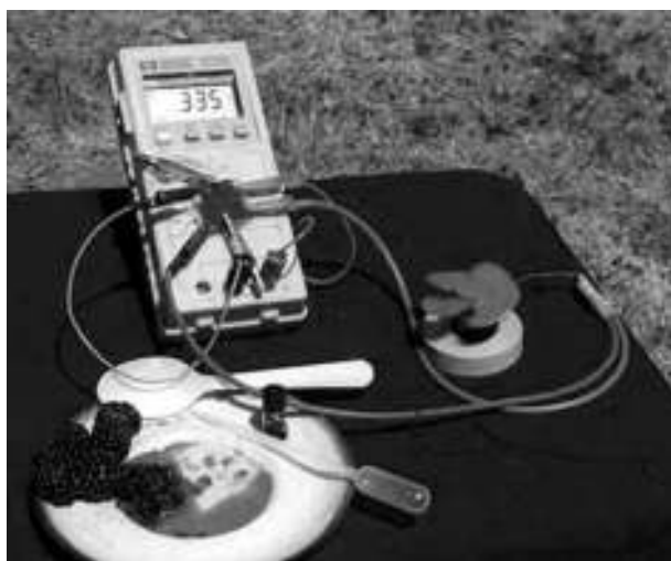
Figure 11-10 The cell driving a small motor. Image courtesy Greg P. Smestad.
