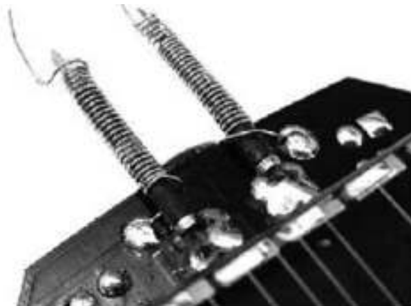
Finished sensor spring installation
