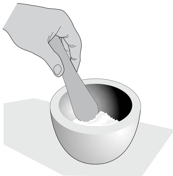
Figure 11-2 Grinding the nanocrystalline titanium dioxide. Image courtesy Greg P. Smestad.
