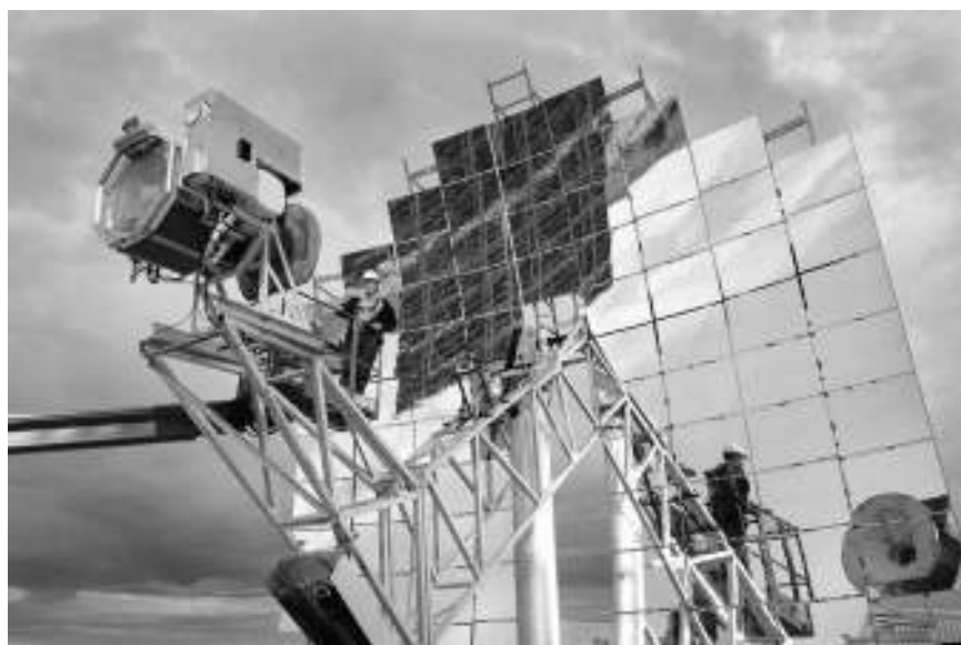
Figure 8-15 Solar dish engine system under test. Image courtesy Sandia National Laboratories/Randy Montoya
