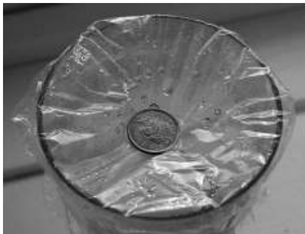
Figure 7-3 Precipitated water in the demonstration still.
