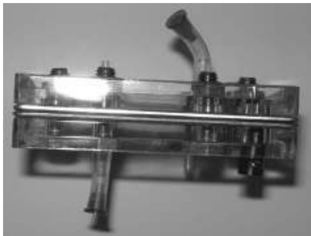
Figure 17-5 PEM fuel cell with rubber hoses.
