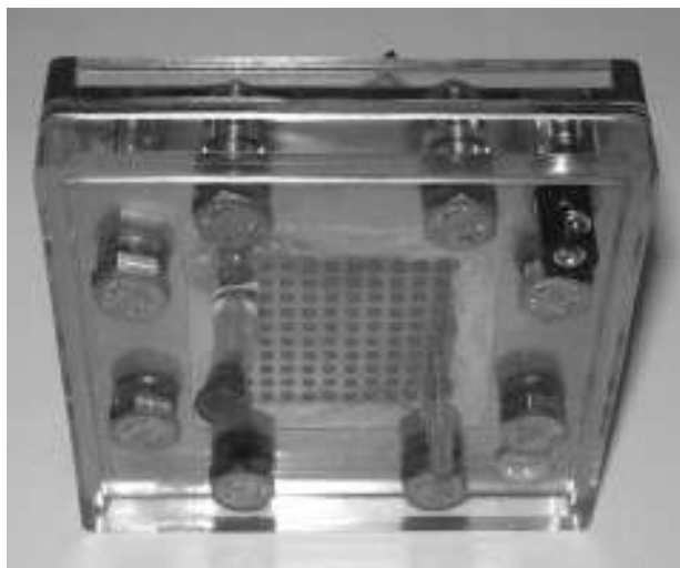
Figure 17-4 PEM fuel cell without caps.
