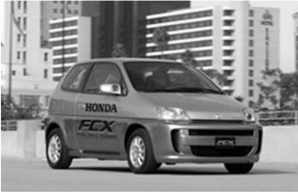
Figure 15-18 Honda fuel cell vehicle. Image courtesy Honda.
