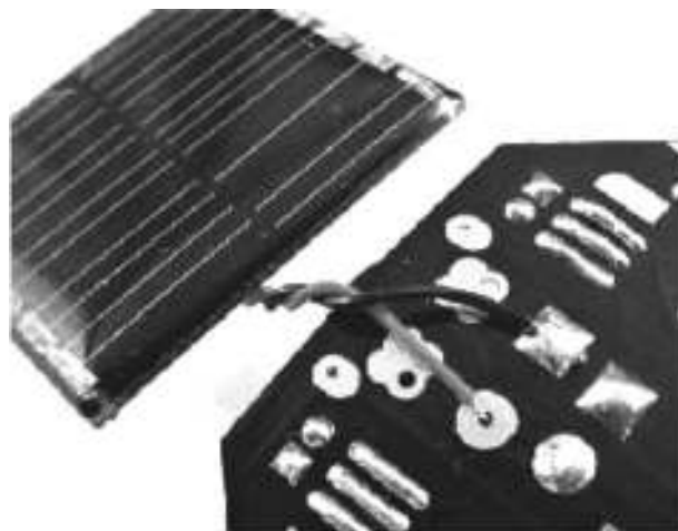
Figure 16-17 Connecting the solar cell to the PCB.
