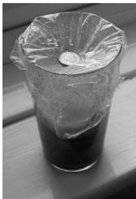
Figure 7-2 Demonstration solar still.
