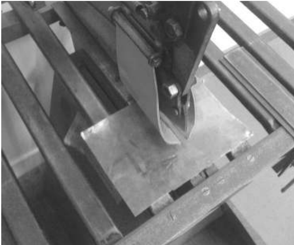
Figure 10-12 Cutting the copper with a guillotine.
