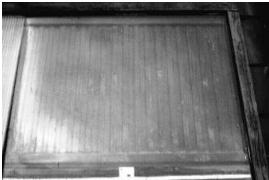
Figure 4-9 A recycled radiator collector.
