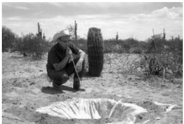
Figure 7-5 A solar still in operation. Image courtesy © U.S. Department of Agriculture—Agricultural Research Service.
