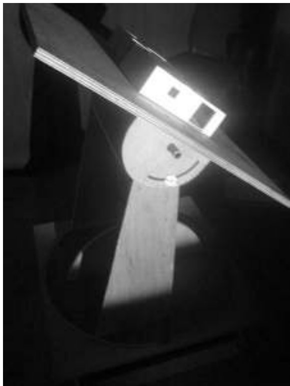
Figure 3-10 A professional architect using a heliodon to make estimations of solar gain on a model building.
