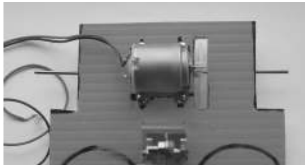
Figure 13-27 Axle and large gear wheel installed.
