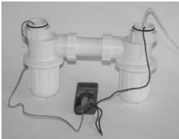
Figure 9-4 The completed microbial fuel cell.
