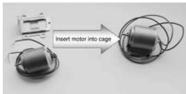
Figure 13-13 Insert the motor in the cage.
