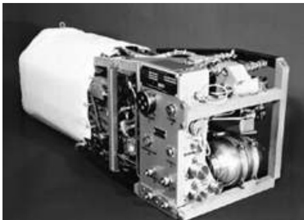
Figure 6-1 An early AFC used in the space program. Image courtesy NASA.
