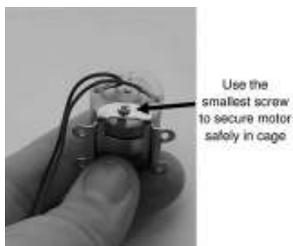
Figure 13-15 A screw secures the motor in the cage.
