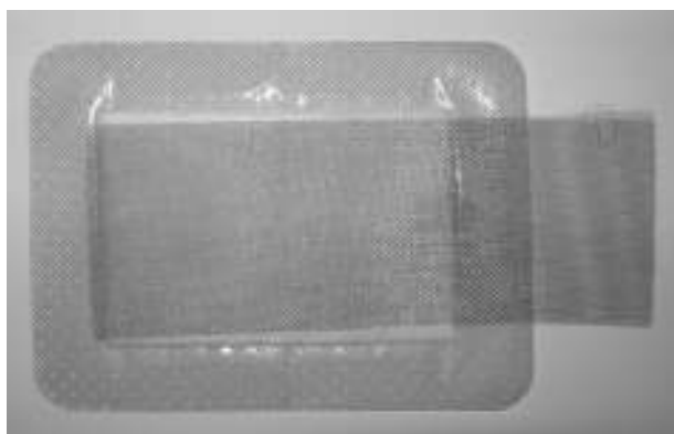
Figure 8-14 Laying the wire mesh on the first Band-Aid.
