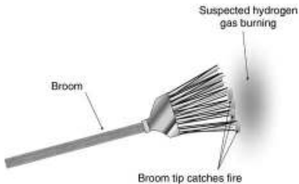
Figure 12-4 Identifying a hydrogen fire with a broom.
