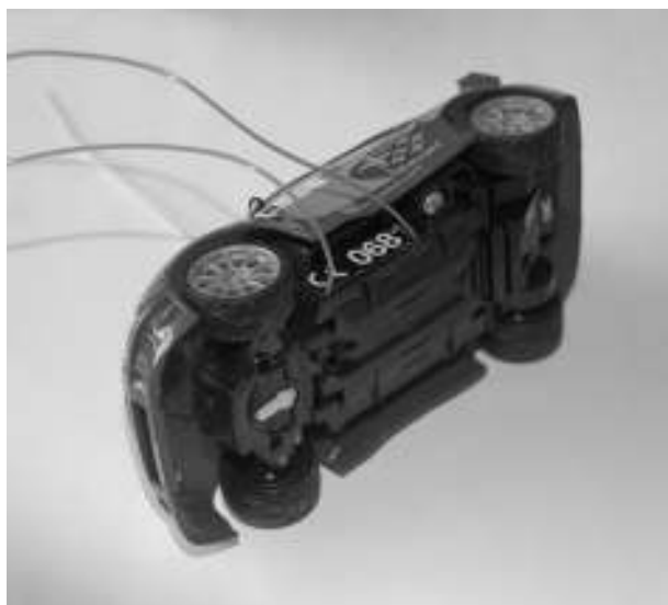
Figure 13-43 Underside of the RC car with wires leading to the battery compartment.
