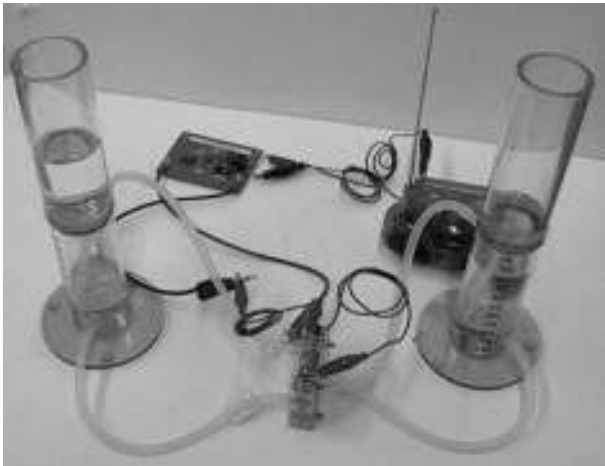
Figure 14-2 Hydrogen-powered radio connected up.
