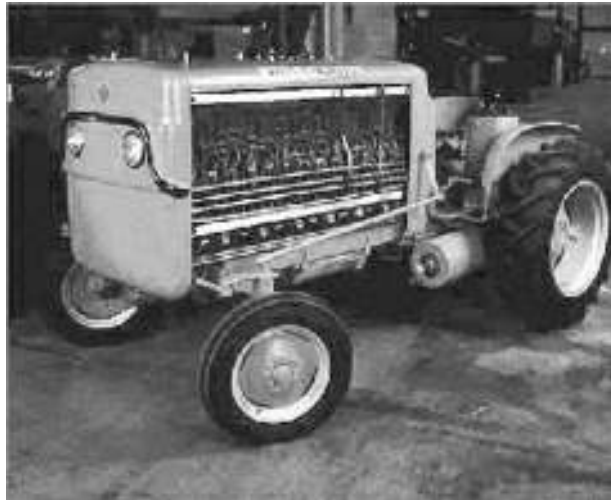
Figure 1-15 Harry Ihrig’s fuel cell tractor.
