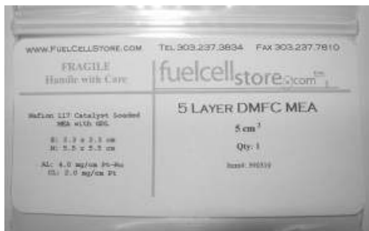
Figure 8-12 Details of the MEA we are using for the Band-Aid fuel cell project.
