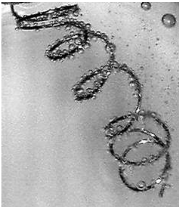
Figure 5-9b Close-up of the hydrogen electrode.
