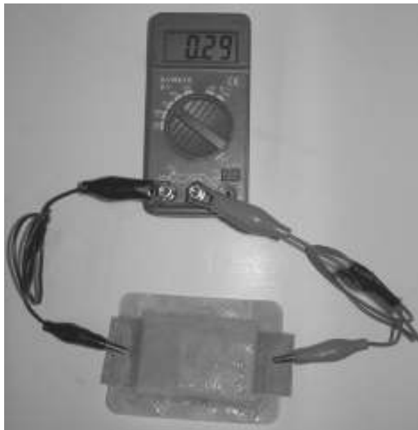
Figure 8-23 The Band-Aid fuel cell connected to a meter.
