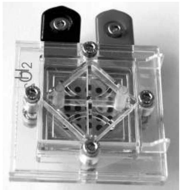
Figure 7-14 The complete dismantlable fuel cell.
