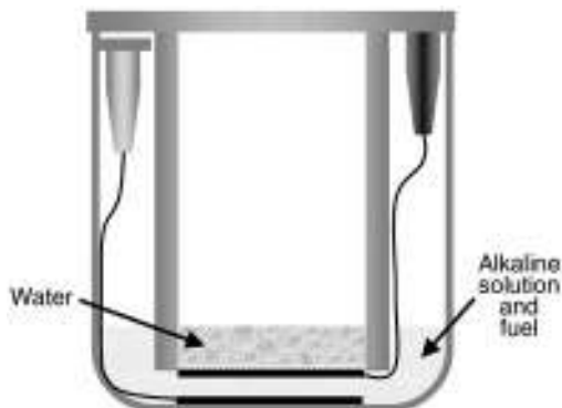
Figure 6-27 The water blocks oxygen.
