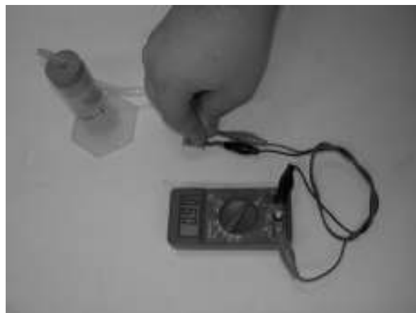
Figure 4-19 Hydrogen produced by the H-Gen powering a mini PEM fuel cell.
