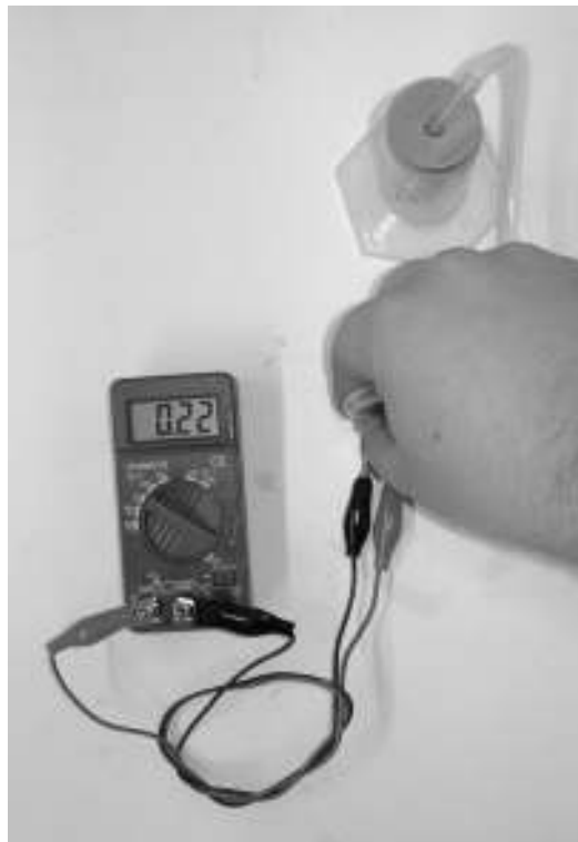
Figure 7-33 Use a multimeter to check power is being produced.
