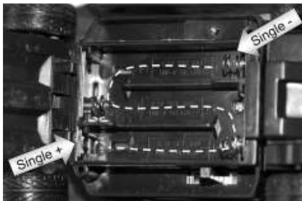
Figure 13-42 RC car battery compartment—terminals labeled.
