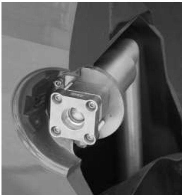
Figure 13-6 A hydrogen coupling on a car.
