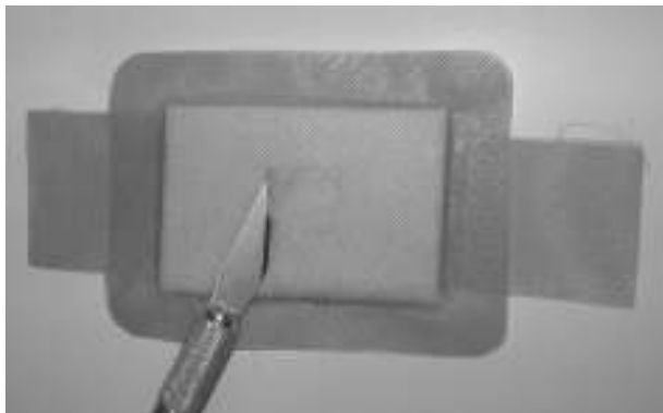
Figure 8-21 Using a scalpel to remove a square from the top layer of the Band-Aid (completing the cuts).
