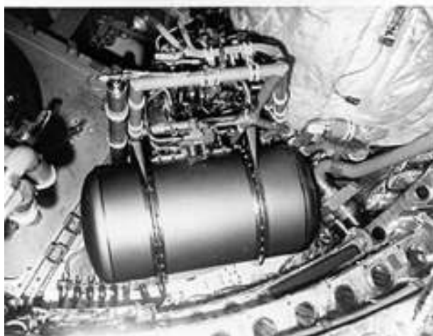
Figure 1-16 Proton exchange membrane fuel cell in Gemini V, 1965. Image courtesy NASA.
