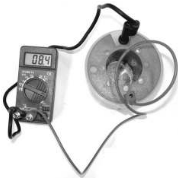
Figure 6-15 The alkaline fuel cell connected to the voltmeter.
