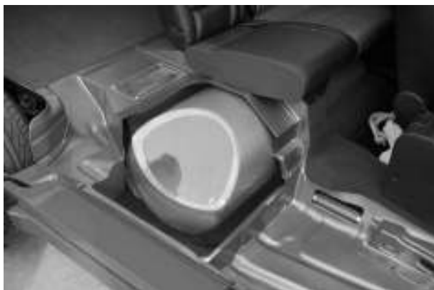
Figure 13-5 Hydrogen storage tanks under the seat of a car.
