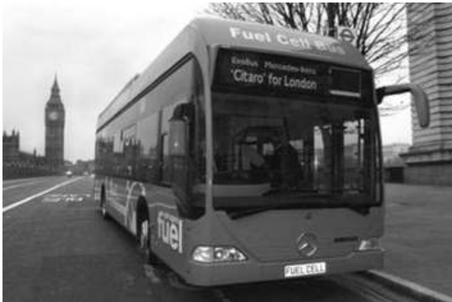
Figure 13-9 A London bus—powered by hydrogen. Image courtesy Ballard.
