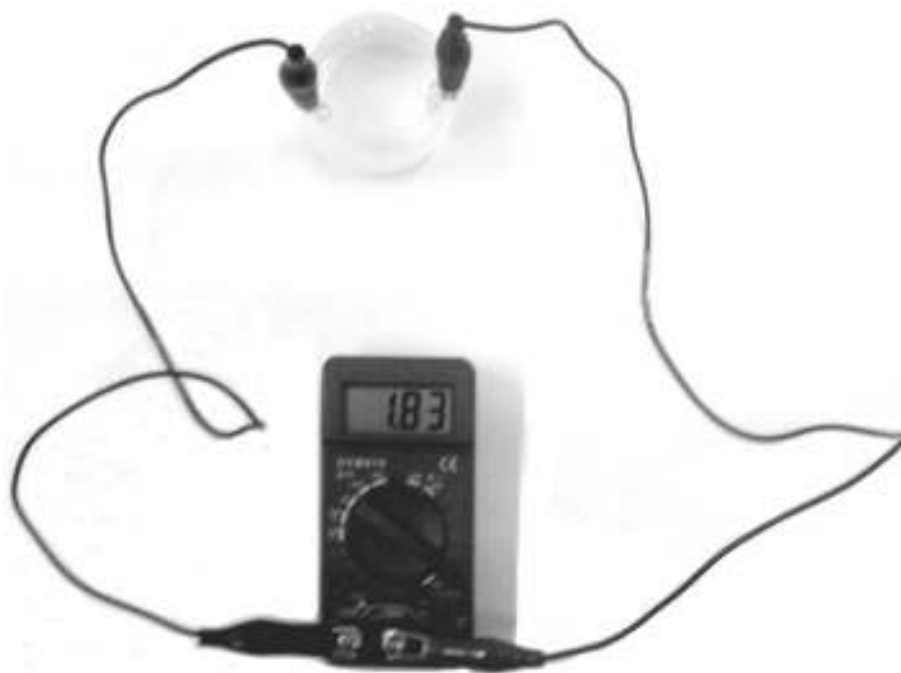
Figure 5-8 The platinum fuel cell generating electricity.
