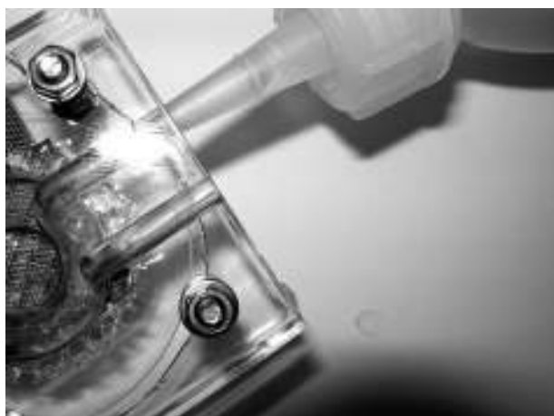
Figure 8-5 Closeup of filling the methanol fuel cell.
