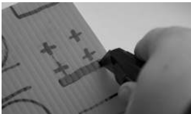
Figure 13-18 Use a sharp craft knife to cut through both layers of the plastic.
