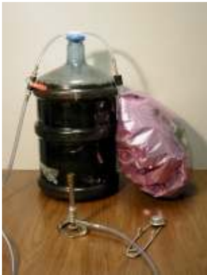
Completed biogas generator.
