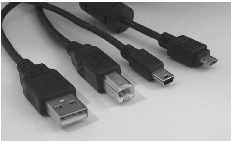
Figure 19-6. Approved cable plugs include (from left) Standard-A for hosts and Standard-B, Mini-B, and Micro-B for devices.
