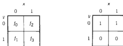
(A) General form. (B) Map for f = x'y' + xy' = \Sigma(0,2) - \Pi(1,3) .
