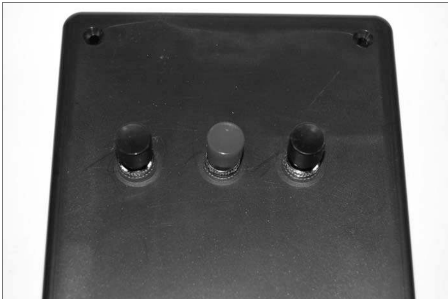
Figure 11-16: Transmitter box with switches installed.
