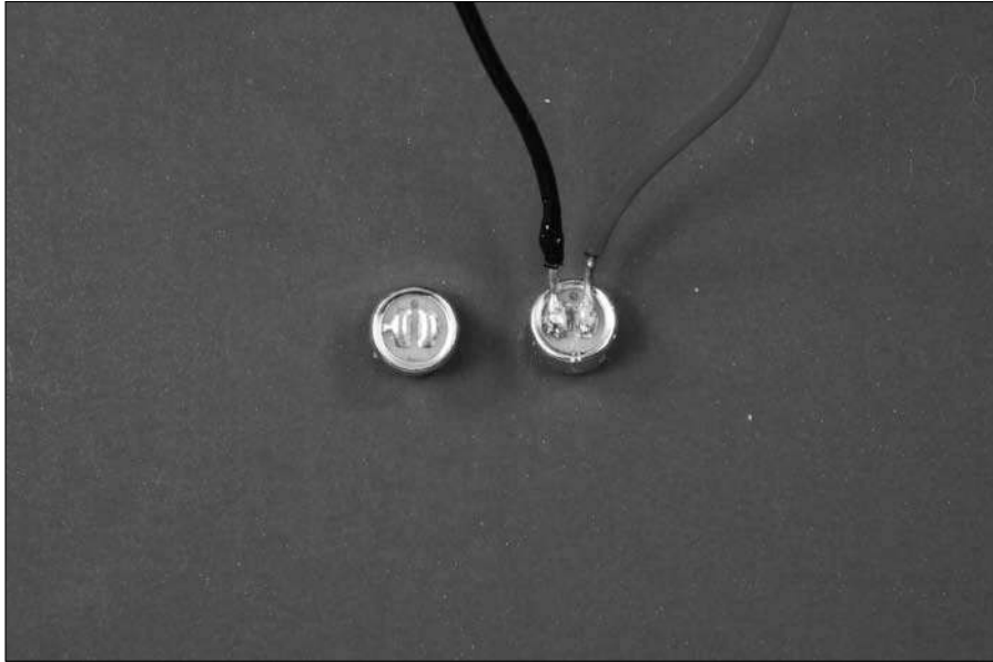
Figure 4-14: Soldering to flat contact pads.
