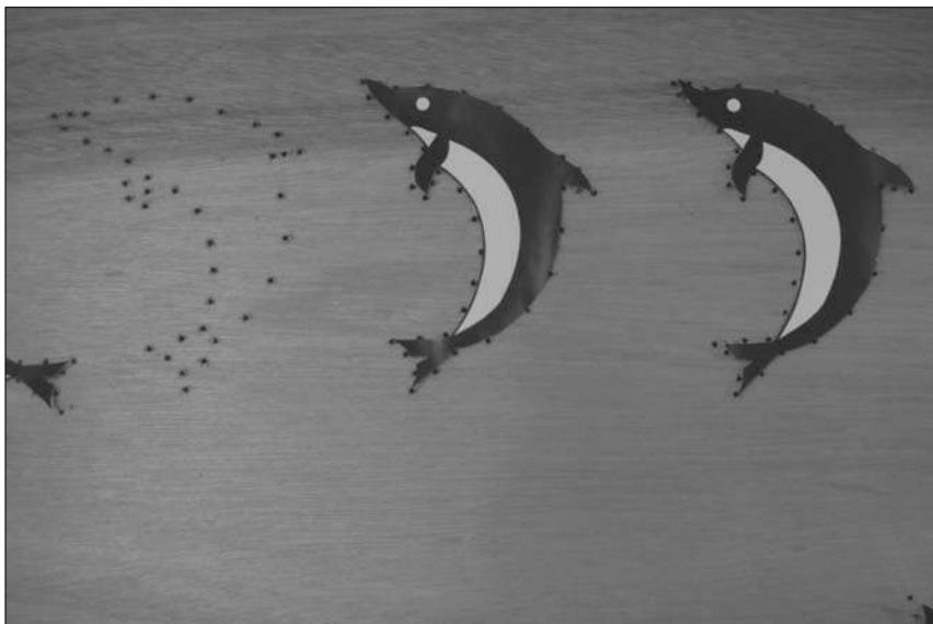
Figure 10-15: A closer look at the dolphin templates with all holes drilled.
