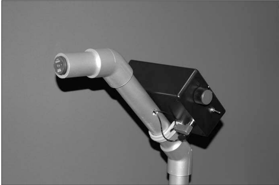
Figure 12-18: The finished metal detector.
