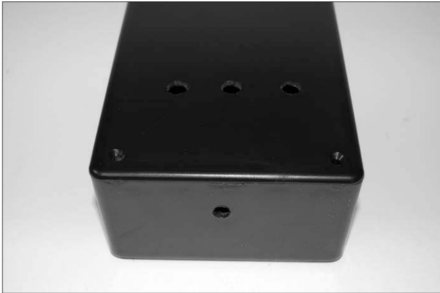
Figure 11-14: Drill holes for the LED and switches.
