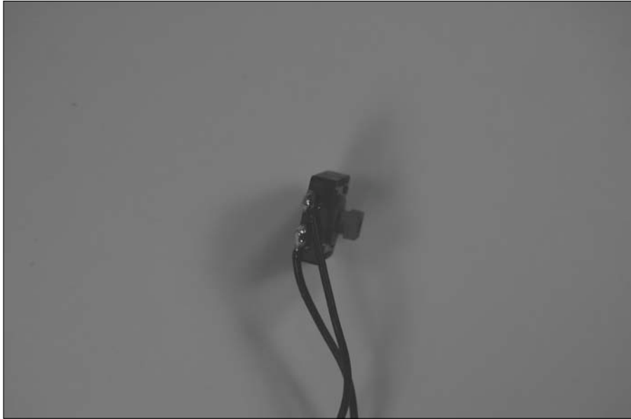
Figure 7-16: Solder wires to tactile switches.
