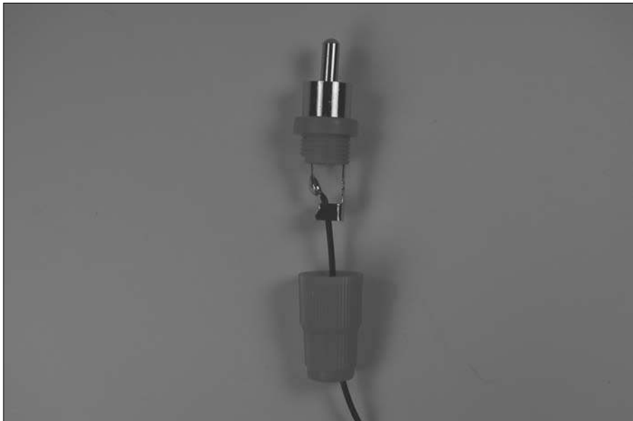
Figure 7-17: Solder wires to phono plugs.
