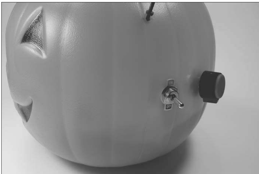
Figure 9-16: Silent pumpkin with switch and potenti- ometer installed.
