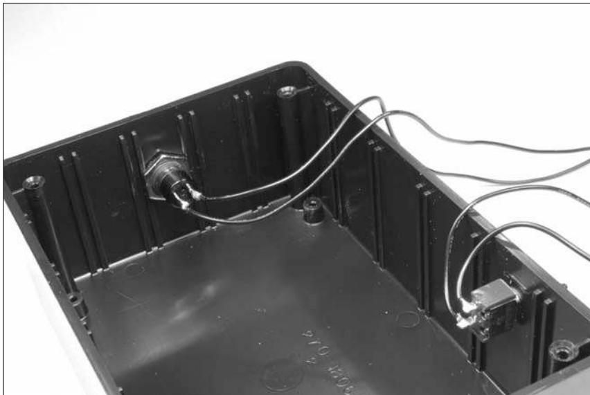
Figure 13-15: Wires soldered to the on/off switch and transmit switch.
