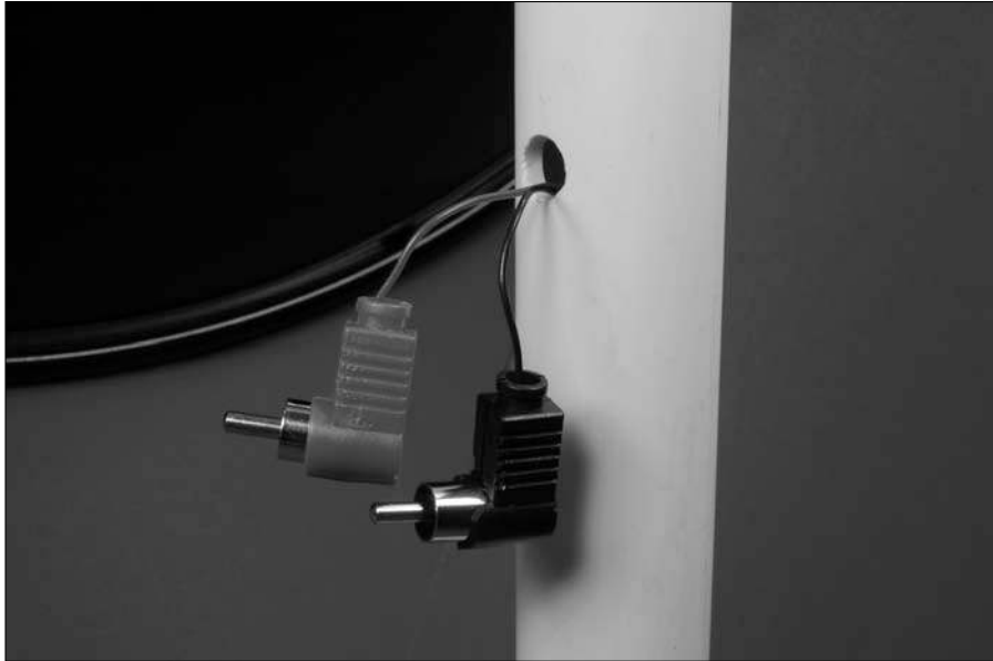
Figure 6-14: Thread wires from the microphone cartridge through the PVC fittings and pipe.
