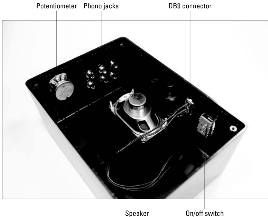
Figure 7-11: Mount components on the box.
