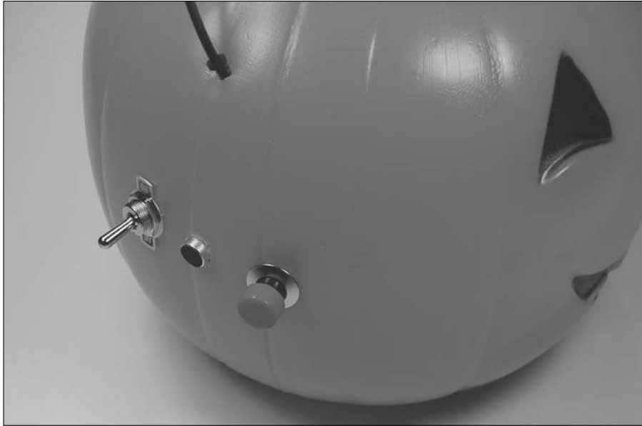
Figure 9-29: Switches and microphone mounted on pumpkin.
