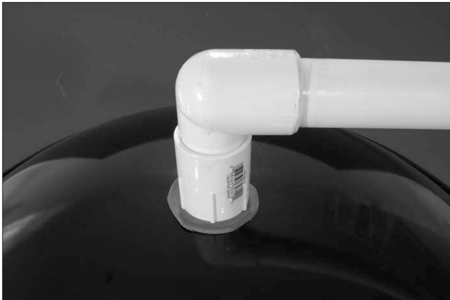
Figure 6-11: Fittings assembled on the parabolic dish.
