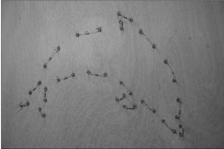
Figure 10-17: Resistors soldered and leads clipped.
