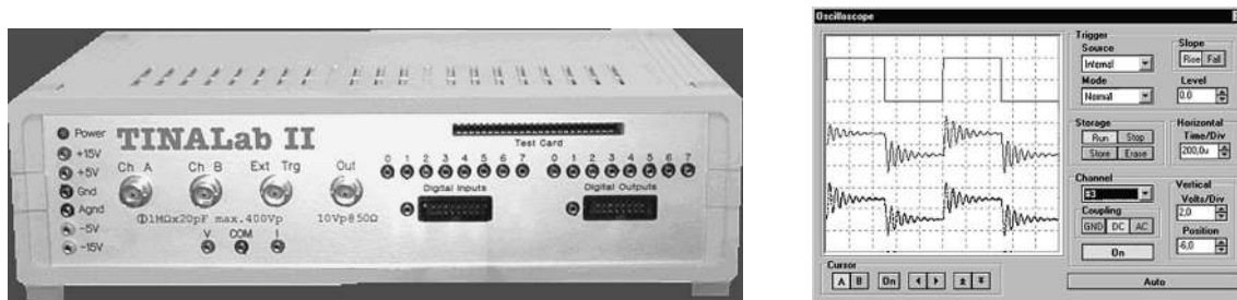
FIGURE 7.62 TINALab II from DesignSoft acts as a multifunction PC test instrument. Comes with digital oscilloscope, multimeter (optional), logic analyzer, signal analyzer, signal generator, and spectrum analyzer. Requires TINAPro circuit simulation software.
