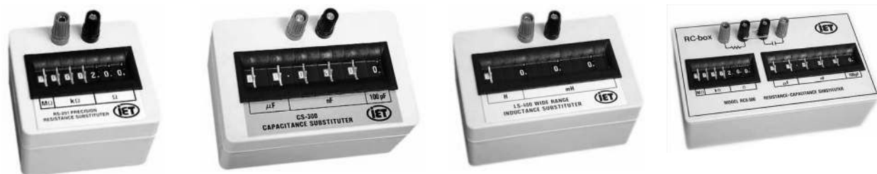
FIGURE 7.66 Selection of resistance, capacitance, inductance, and RC boxes from IET Labs, Inc. Resistance boxes come in seven- (0 to 9,999,999 Ω, 1-Ω resolution) and nine- (0 to 99,999,999.9 Ω, 0.1-Ω resolution) decade types. Capacitance boxes come in six (0 to 99.9999 vF, 100-pF resolution) decade types. Inductance boxes come in three (999 mH, 1-mH resolution) and four (9.999 mH, 1-mH resolution) decade types. RC boxes come with mixed decade selections given in provision R and C boxes. Uses thumbwheel switches to dial in resistance, capacitance, and inductance values. Accuracy is typically 1 percent or better.
