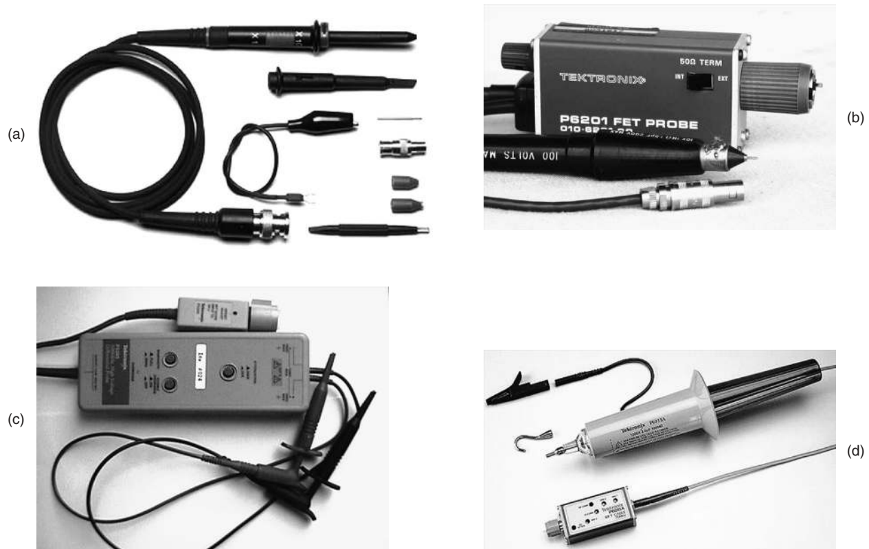
FIGURE 7.58 (a) General-purpose 1X/10X passive probe with assortment of probe attachments designed for use with a 1-M \Omega , 20-pF scope. At 1X, there is no attenuation, but the bandwidth is limited to between 4 and 34 MHz. At 10X, signals are reduced to one-tenth their original magnitude, while the bandwidth increases from between 60 and 300 MHz, depending on the probe and scope. (b) Active probe used primarily for high-frequency, low-voltage work. An active probe's internal FET provides extremely low-input capacitance (>1 pF) that allows for high bandwidths (500 MHz to 6 GHz) and minimal circuit loading. The probe typically comes with a 50- \Omega output impedance to drive a 50- \Omega cable, making it possible to increase probe cable length. It may require a special scope with a power connector/signal connector, or an external power source. A limited voltage range of \pm 40 V is typical. (c) Differential probe houses an internal differential amplifier that allows you to make differential measurements (between any two points, not just between one point and ground). Differential probes come in 50- \Omega and 1-M \Omega packages, and may require a special scope with a power connector/signal connector or an external power source. (d) High-voltage probe used for heavy-duty measurements of voltages over 2.5 kV. The P6015A from Tektronix can measure dc voltages up to 20 kV (RMS) and pulses up to 40 kV. It comes with a bandwidth of 75 MHz. Other high-voltage probes, often termed 100X, 1000X, will provide varying maximum voltage and bandwidth limits.
