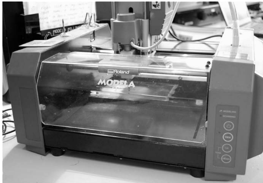
FIGURE 7.10 A CNC router cutting a PCB.
