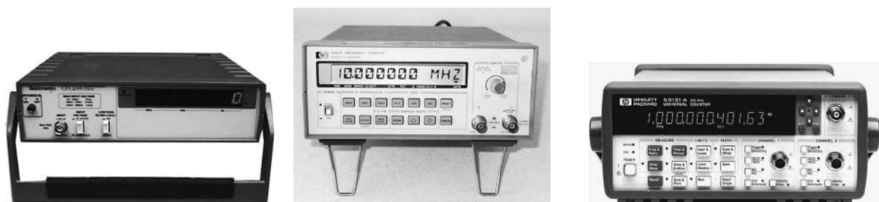
FIGURE 7.60 A selection of used frequency counters. Left: Tektronix CFC-250, dc to 100-MHz counter found new in the box for $95. Center: HP 5385A, 10-Hz to 1-GHz counter with eight-digit display, which comes with two input channels—found for around $200, used, on eBay. Right: HP 5342A, 10-Hz to 18-GHz counter with 12-digit display—expensive.
