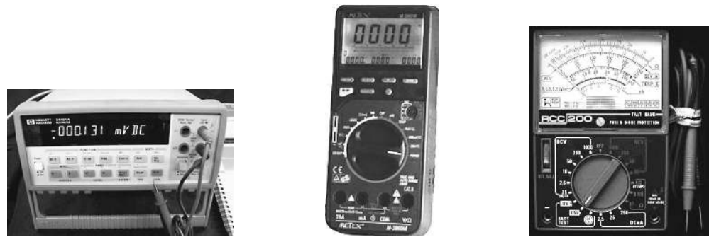
FIGURE 7.53 Left: HP 34401A bench DMM with 6.5-digit resolution and computer interface. Center: Metex M-3860M 3½ digital DMM loaded with handy features, such as an RS232 interface, true RMS, temperature, inductance, capacitance, logic analyzer, transistor hFE tester, diode tester, and frequency counter. Right: A simple analog meter useful for monitoring trends.
