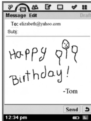
FIGURE 42.43 Example of ink messaging application for mobile devices. Users can draw or write with a stylus on the device screen to compose an e-mail in their own handwriting; no automatic recognition is necessarily involved.
