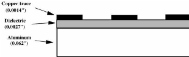
Figure 10.33 Single-layer insulated metal substrate cross section.
