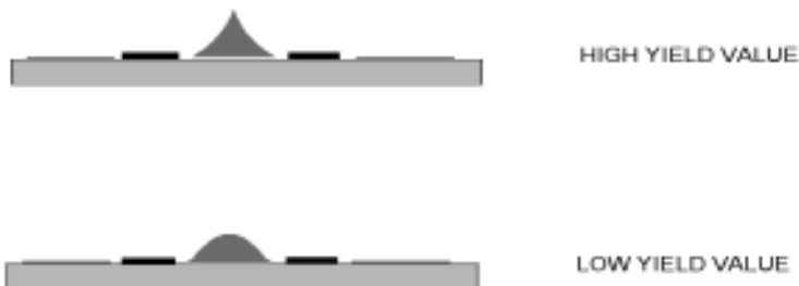
Figure 9.48 Effect of yield point on chip bonder dot profile.
