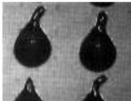
Figure 9.35 Photo of a stringing defect.
