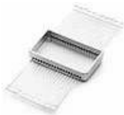
Figure 8.41 Flat ("butterfly") package.
