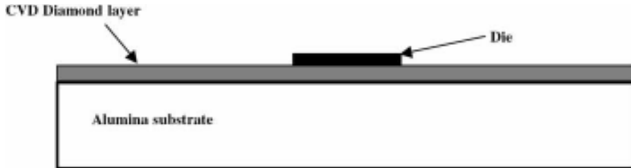
Figure 10.31 CVD diamond layer on alumina substrate.
