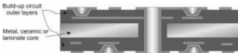
Figure 7.31 HDI construction Type 4, described in text.
