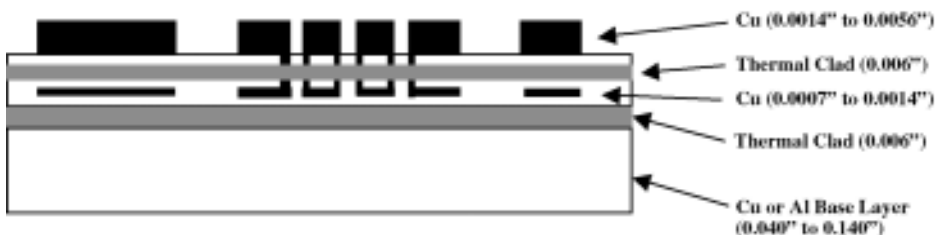
Figure 10.34 Two-layer insulated metal substrate cross section.
