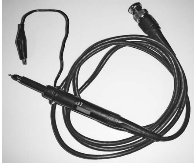
FIGURE 2-4 Oscilloscope probe, 10X/1X switchable
