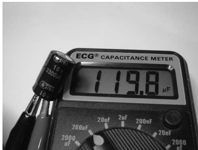
FIGURE 7-2 Bulging electrolytic capacitor with greatly reduced capacitance
