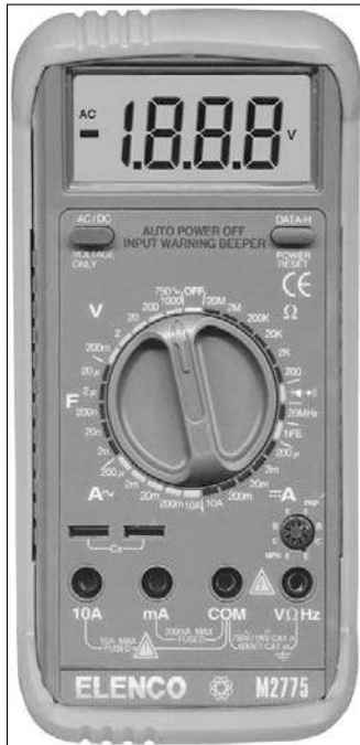
Figure 9-2: Multimeters measure voltages, resistance and current.
