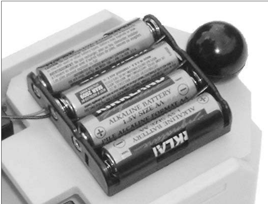
Figure 8-4: Four 1.5-volt batteries tucked into a battery holder produce about 6 volts across the red and black leads.
