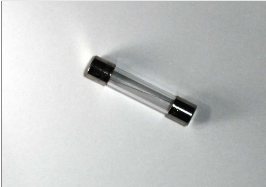
Figure 2-6: A 2 A, 1-1/4" x 1/4" AGC fuse.
