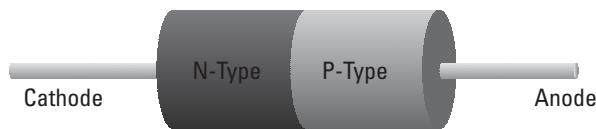
Figure 5-5: A diode has a single p-n junction.
