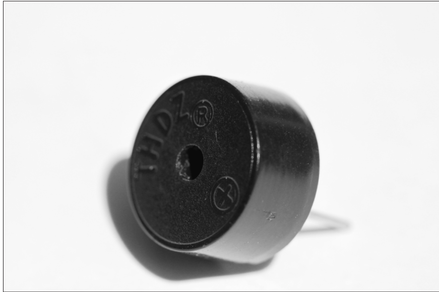
Figure 4-1: The piezo- electric speaker that comes with the BASIC Stamp Activity Kit.
