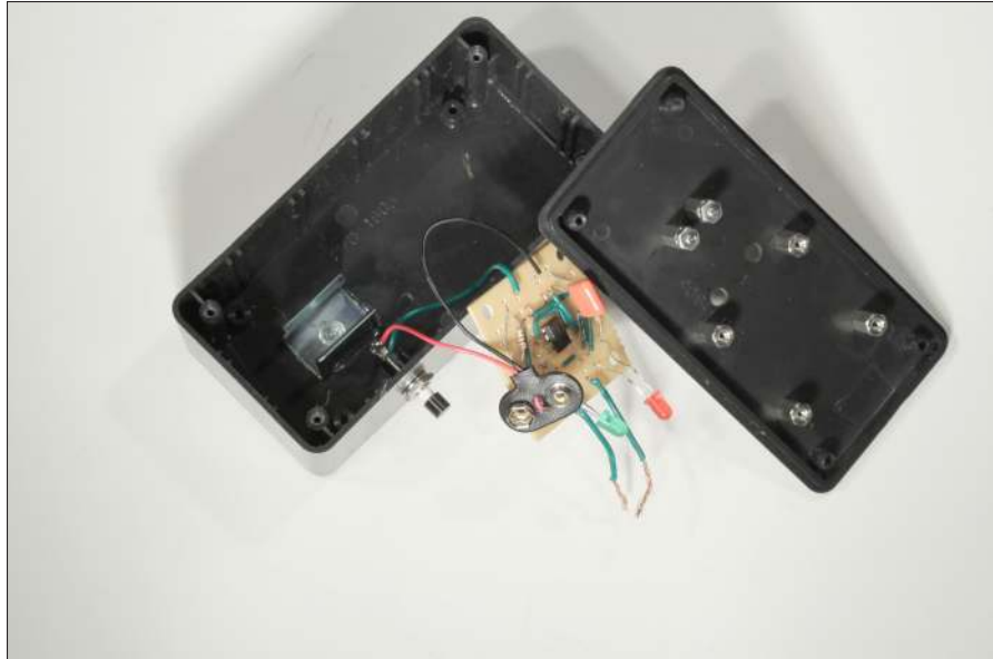
Figure 6-20: The box with the pushbutton, battery holder, and standoffs installed.
