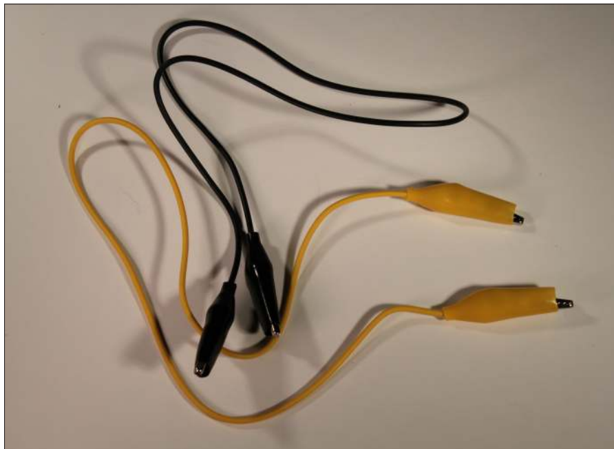
Figure 3-14: Jumper clips are great for making quick connections.
