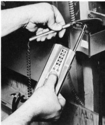
Figure 14-6 Voltage tester. Courtesy Amprobe Instrument Division of SOS Consolidated, Inc.
