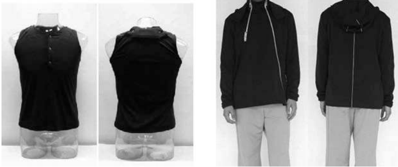
FIGURE 2.10 Design prototype of bio-monitoring clothing for measuring electrocardiogram. Left: Design for innerwear. Right: Design for outerwear.
