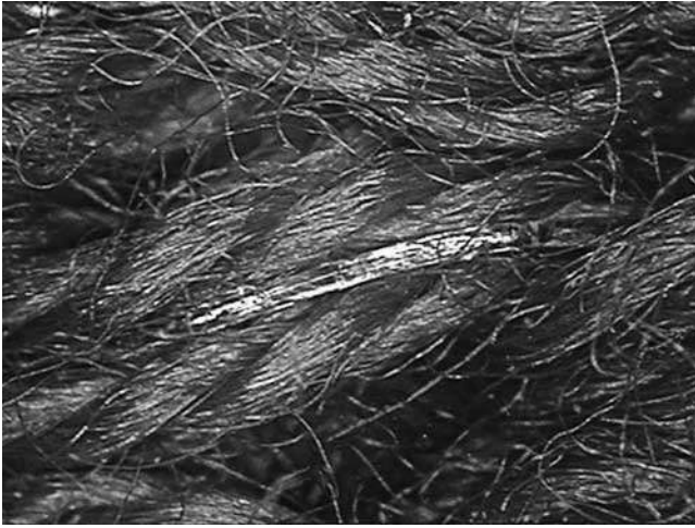
FIGURE 5.11 POF-integrated weft knitted fabric.
