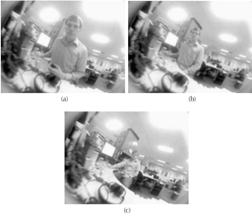
FIGURE 9.9 Three images captured with a fisheye lens. Image (a) was captured at a distance of 0.5 m; image (b) was captured at 1 m; and image (c) was captured at 1.5 m.
