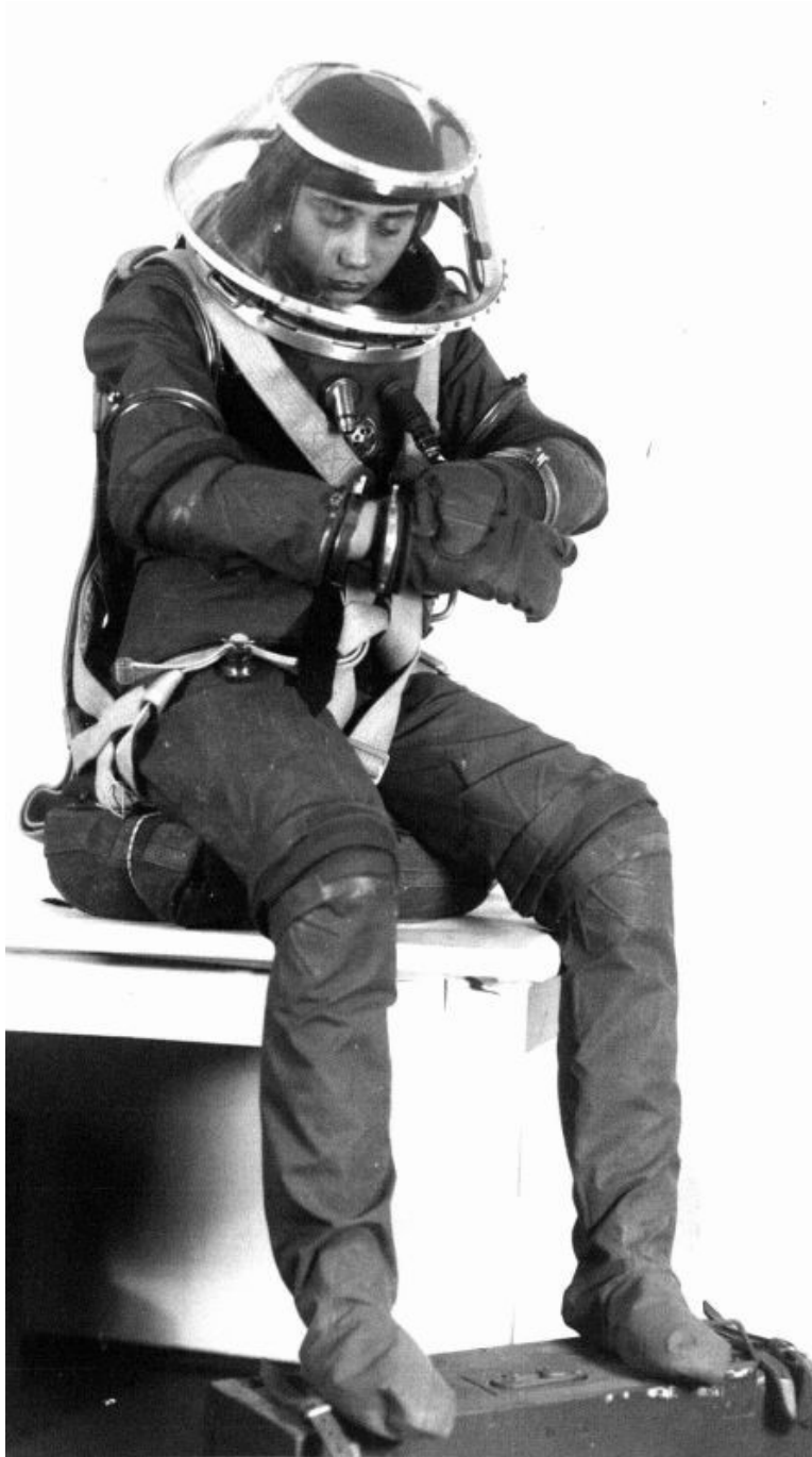
Figure 5.17: Dräger pressure-suit "Leichter Druckanzug, Modell 8" from 1943. Reproduced by permission from the Bundesarchiv.
