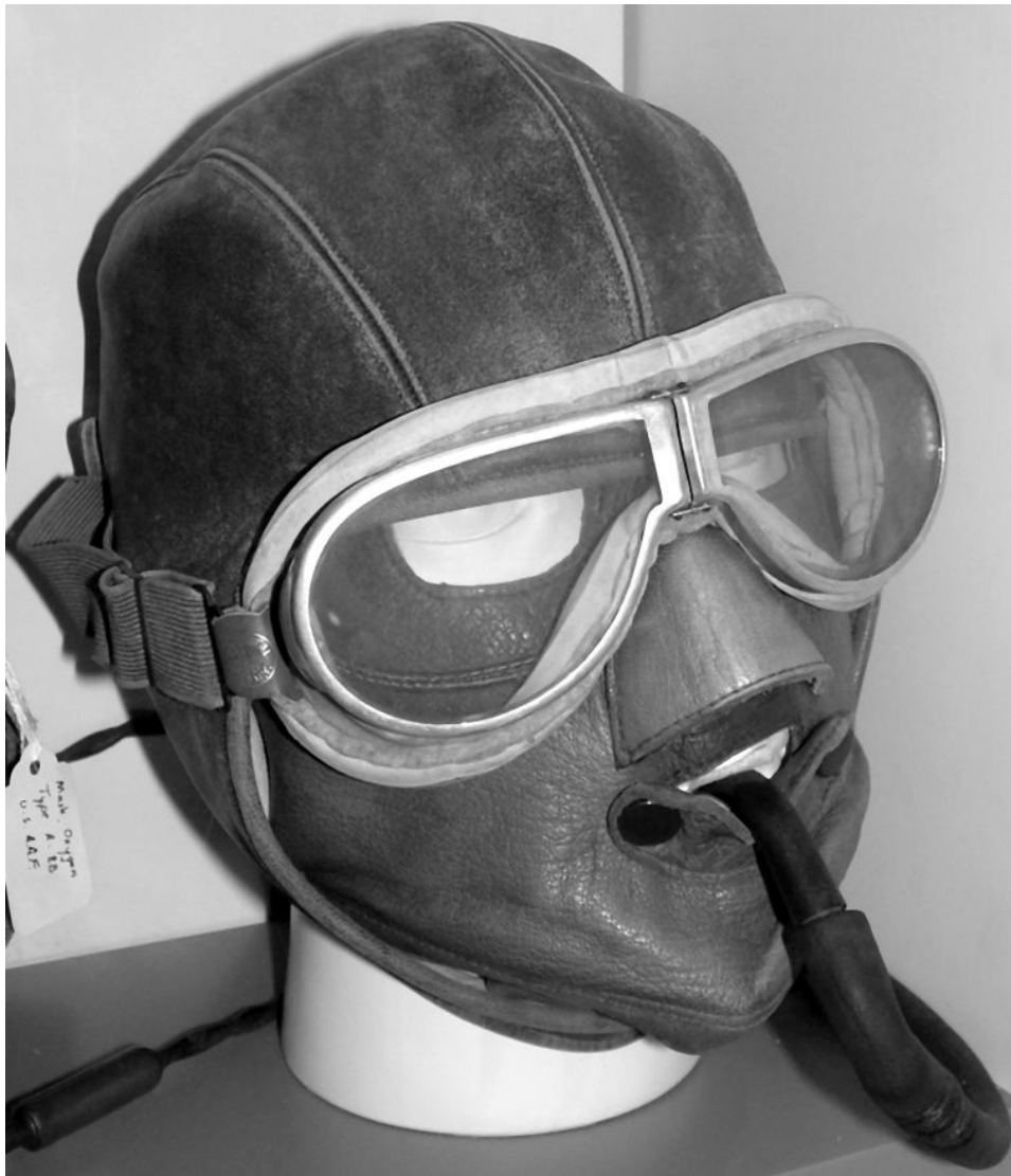
Figure 5.44: Pipestem system with face mask, USA, c. 1920s/30s, on display in the NASM.
