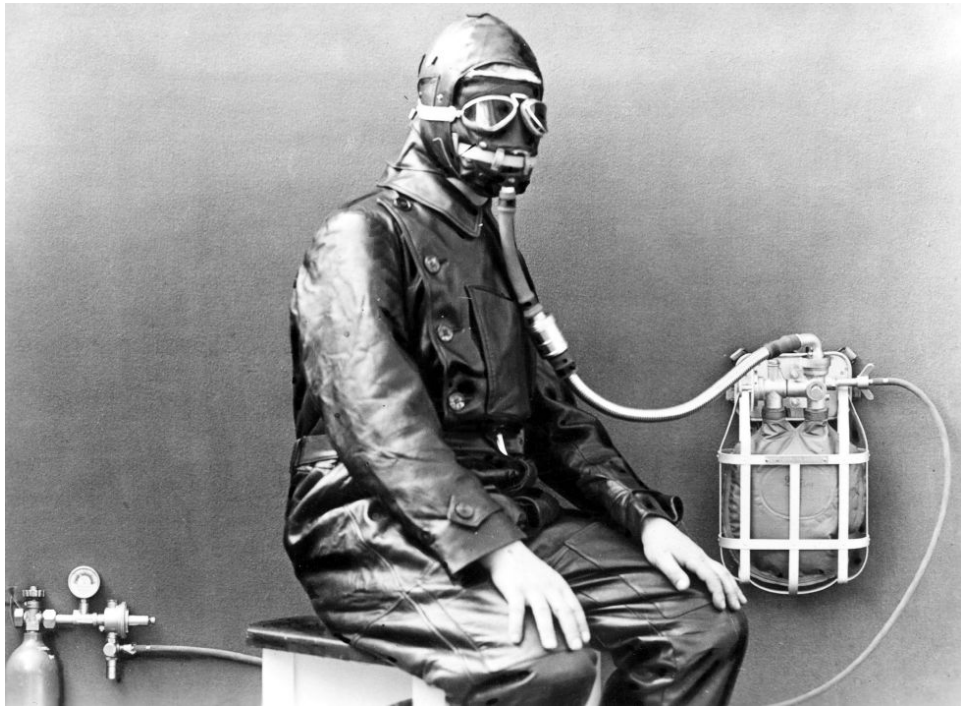
Figure 5.41: Pilot's garment and high altitude breather, c. 1929. Reproduced by permission from the Deutsches Museum.
