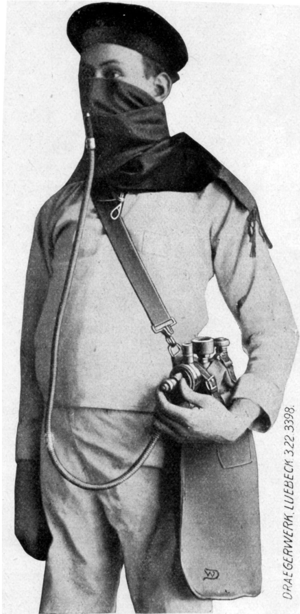
Figure 5.43: Dräger high-altitude breather with pipe-stem and face mask. Taken from Dräger-Hefte, 1922.
