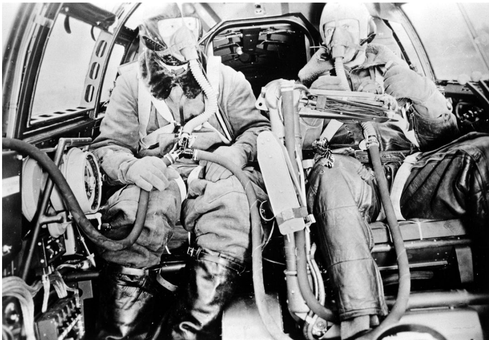
Figure 5.42: German bomber pilots in a Heinkel He111 in 1941, using Dräger high-altitude breathers. Reproduced by permission from the Deutsches Museum.
