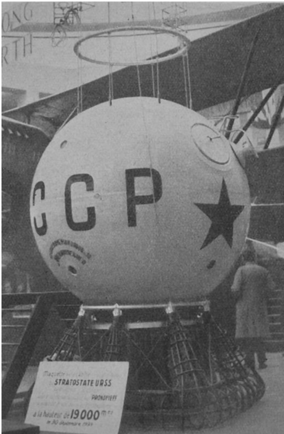
Figure 5.5: Sealed gondola of the Soviet balloon “USSR”, taken from the magazine “Luftwelt”, 1934.
