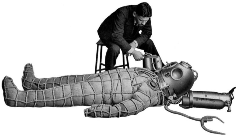
Figure 5.25: Dräger Recompression Suit from 1915, illustration from Umschau (1918).
