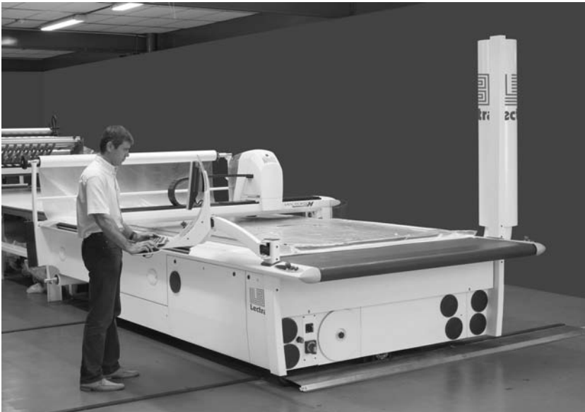
Figure 2.15 Computer-controlled knife cutting and table. (© Lectra Systems Ltd., reproduced by permission.)
