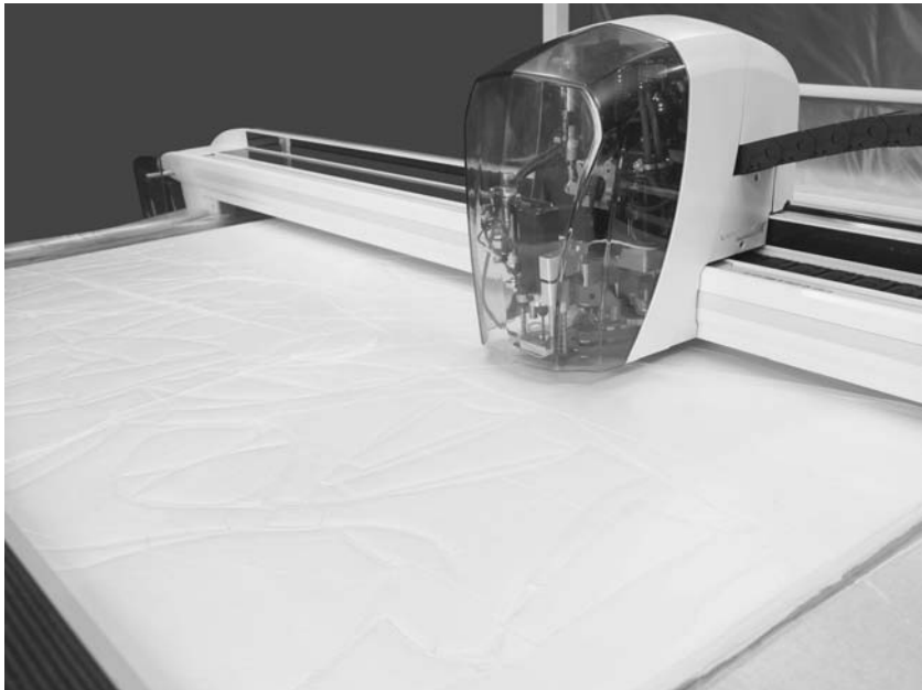
Figure 2.16 Computer-controlled cutting head in action. (© Lectra Systems Ltd., reproduced by permission.)
