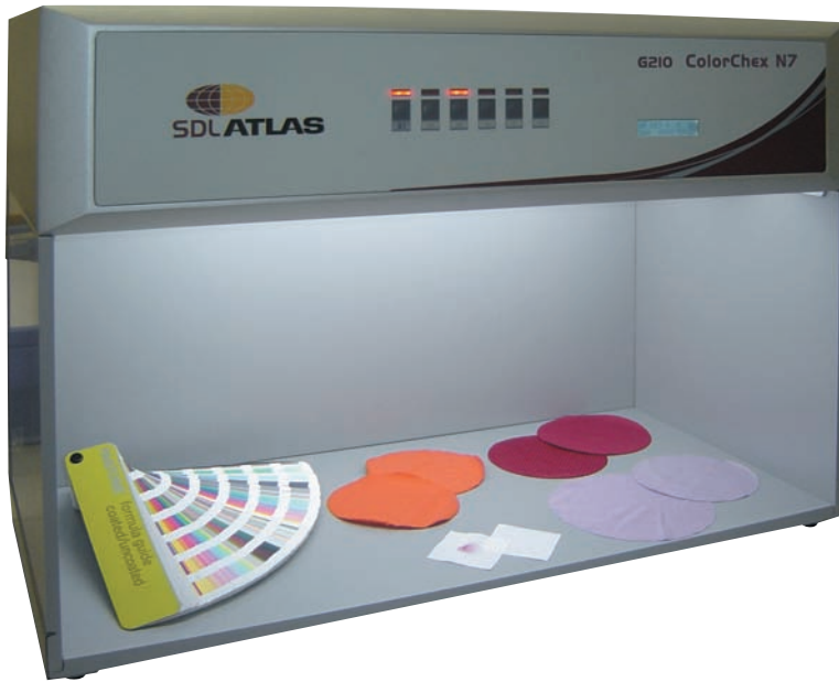
Figure 8.5 Light cabinet. (Reproduced by permission of ASL Atlas Inc.)
