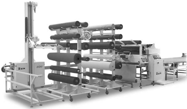
Figure 2.9 Automated system for handling open-width rolls. (Reproduced by permission of Macpi Group.)
