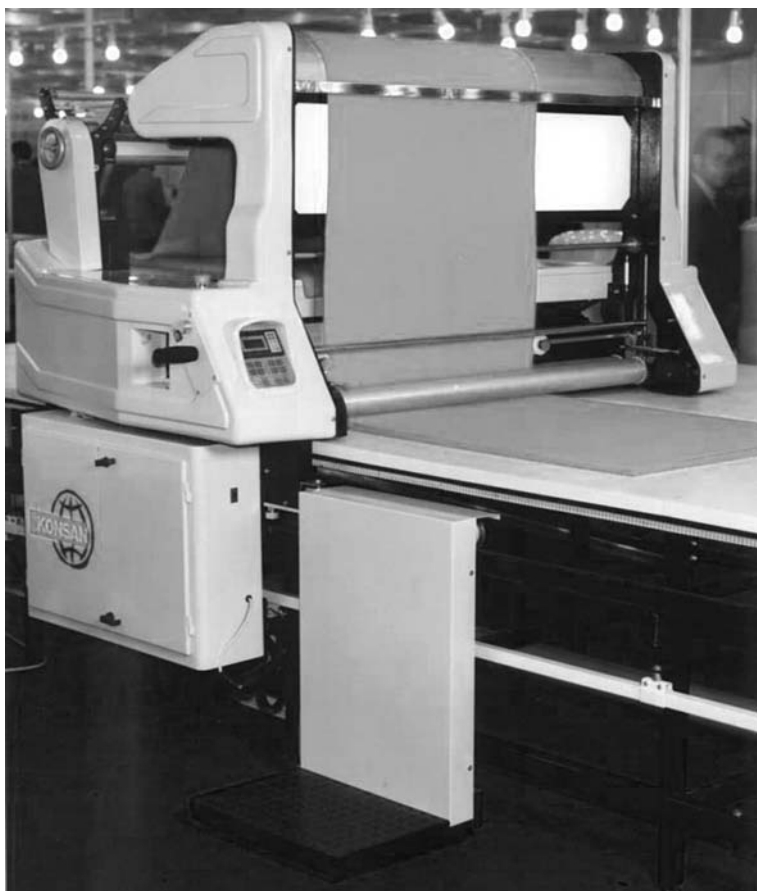
Figure 2.8 Spreading machine for tubular knitted fabric (Reproduced by permission of the Konsan Machinery Co.)
