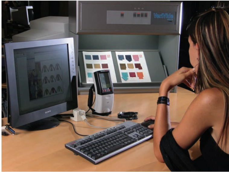
Figure 8.3 The Kaledo Color Match for colour management and communication, with calibrated VDU, portable spectrophotometer and light cabinet for swatches. (© Lectra Systems and used with permission.)
