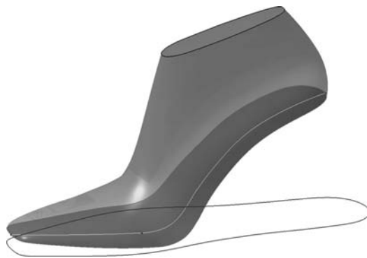
FIGURE 10.19 A last model showing the last bottom surface, the last bottom featherline (in orange), the last bottom centerline, and the surface development of the last bottom onto the bottom plane (in red).
