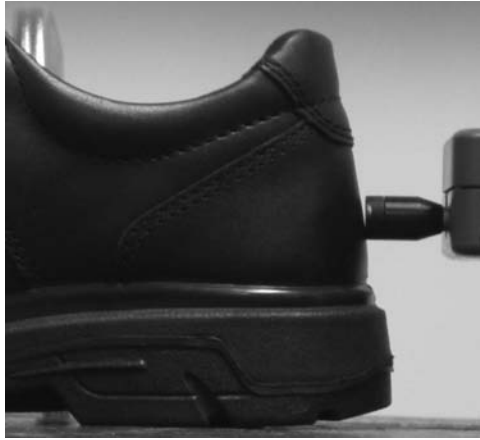
FIGURE 20.6 Alignment of soft-faced indenter at posterior aspect of heel counter.
