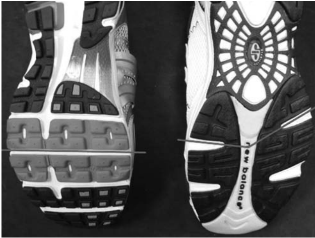
FIGURE 16.3 Sole flex angles differ between sole design, altering forefoot propulsion.
