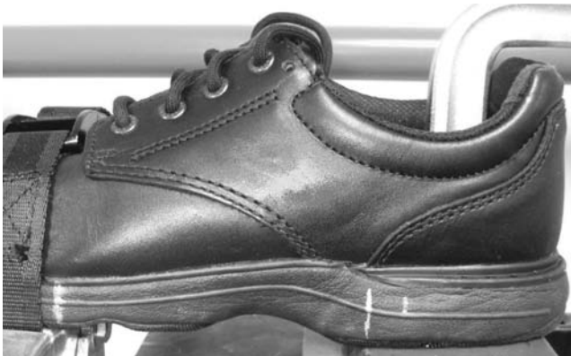
FIGURE 20.9 Torsional stiffness test rig setup showing clamp to grip heel and restraining strap for front platform. Note that the shoe is located according to 30% and 66% marks.
