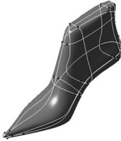
FIGURE 10.6 Tessellated model is subdivided into patches by forming intersection curves. The intersection curves are subsequently smoothed.
