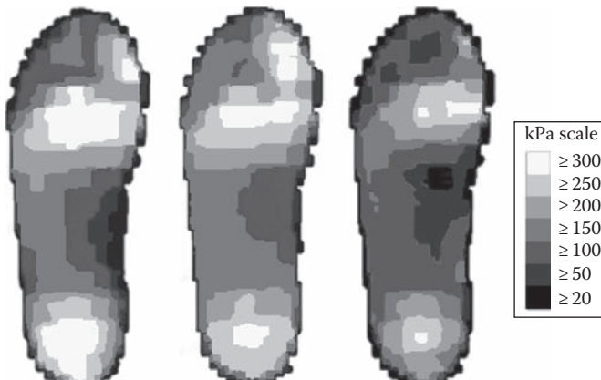
FIGURE 22.1 Peak plantar pressure distributions when running barefoot on grass (left), when running in Nike Free footwear (middle), and when running in footwear with a conventional foam and encapsulated air bladder midsole (right). Maximum pressures are developed at different regions at different times during stance. (Data from Pisciotta, J., Woo, H., Mientjes, M., Bloomer, L., Gregg, M., Nike Sport Research Lab, Beaverton, OR.)
