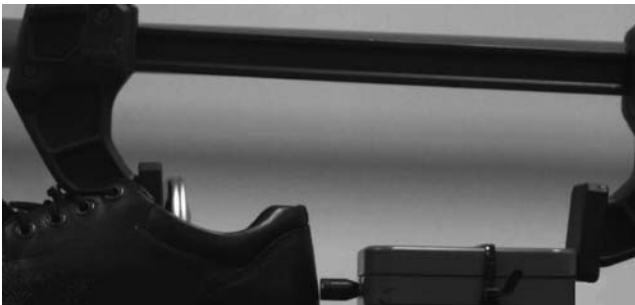
FIGURE 20.5 Setup for heel counter stiffness test rig showing first clamp in throat of shoe to maintain stability and second clamp with trigger grip providing compression through force gauge.
