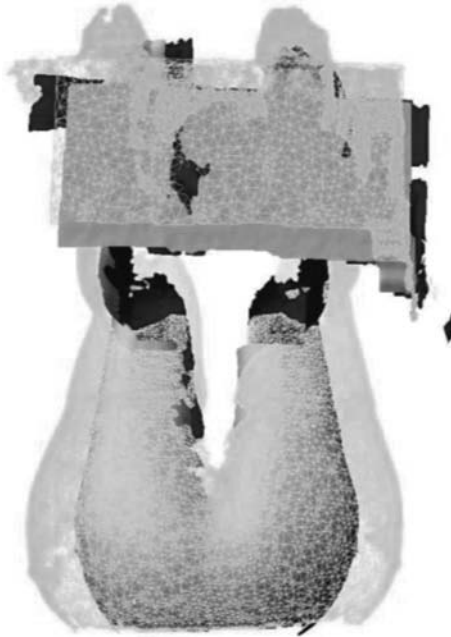
FIGURE 6.10 3D Scan overlay of multiple subjects to determine the overall contour of the seat pan.
