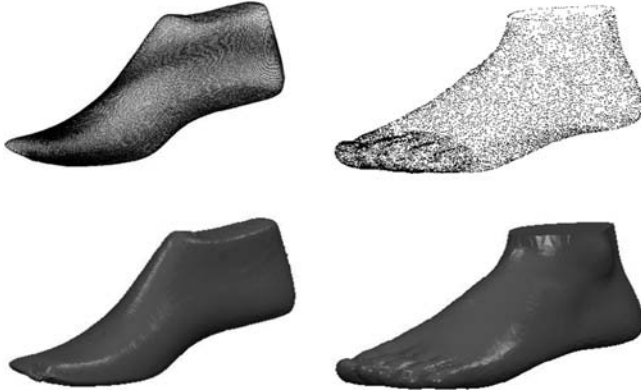
FIGURE 7.9 Last and foot point clouds and the recovered surfaces.
