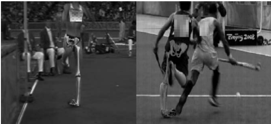
FIGURE 27.2 Using model-based image-matching (MBIM) technique, skeleton model was superimposed on the body image in order to measure the ankle joint kinematics. (From Mok, K.M. et al., Am. J. Sports Med. , 39(7), 1548, 2011a, http://ajs.sagepub.com/content/39/7/1548 )
