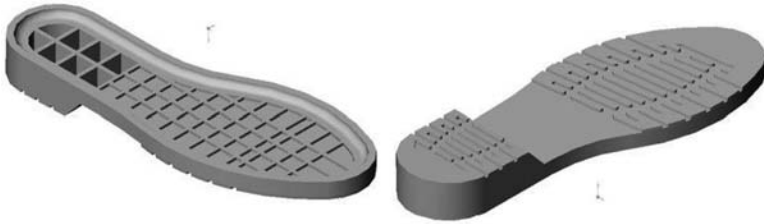
FIGURE 10.26 Two views of an outsole for a men's dress shoe.
