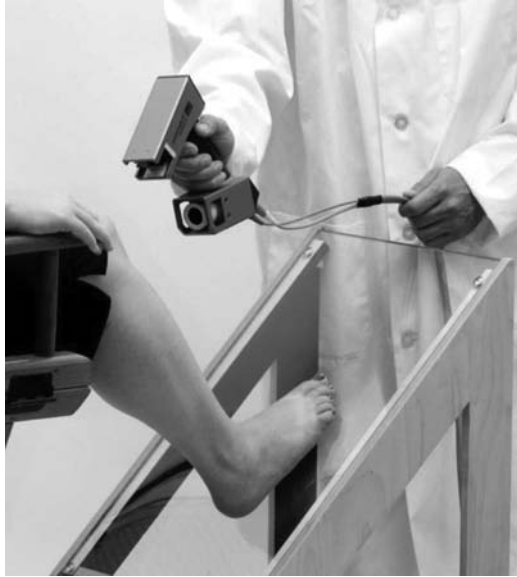
FIGURE 5.2 3D scanner—scanGogh II.
