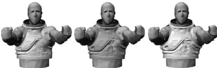
FIGURE 6.11 Merging of CAD models with the 3D scan images.
