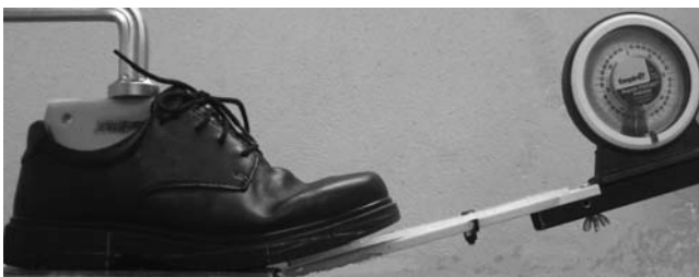
FIGURE 20.7 Flexion stiffness test rig setup showing restraining clamp acting through truncated last and hinged platform with inclinometer.
