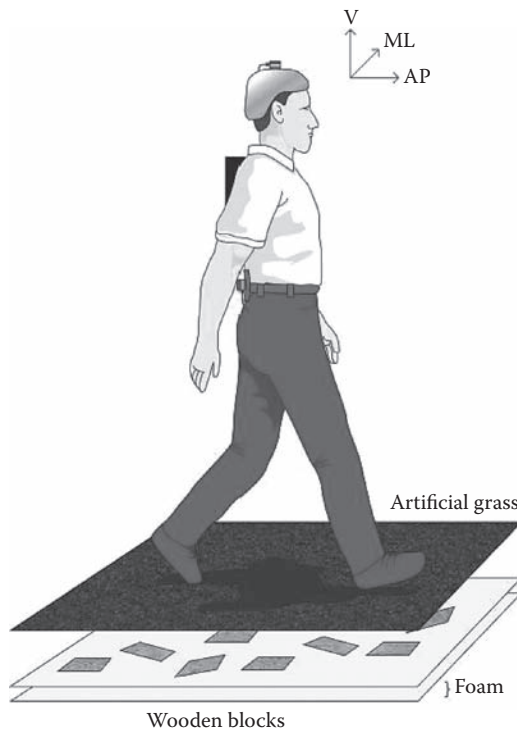
FIGURE 24.7 Irregular surface created using layers of foam, wooden blocks, and artificial grass.
