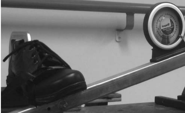
FIGURE 20.8 Torsional stiffness test rig setup showing front platform with central axis of rotation.
