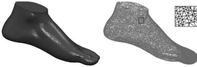
FIGURE 7.12 Reconstructed mesh surface using Voronoi method.
