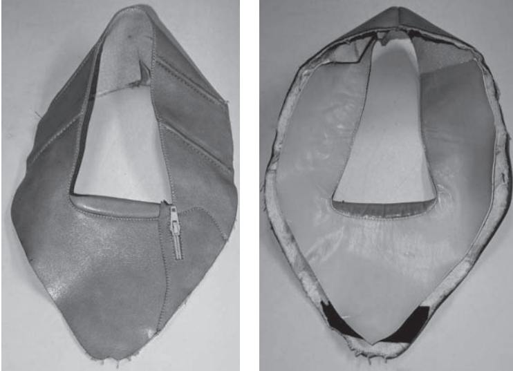
FIGURE 10.32 Views of outer and inner sides of a stitched shoe upper.
