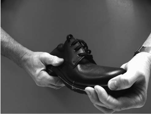
FIGURE 20.4 Method for manual assessment of torsional stiffness showing twist through length of the shoe.
