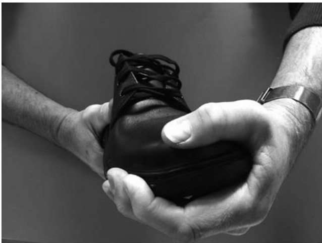
FIGURE 20.3 Method for manual assessment of torsional stiffness showing inversion of forefoot.
