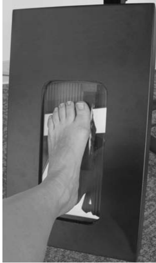
FIGURE 13.8 Laser scanner for creating a 3D image of the foot morphology.
