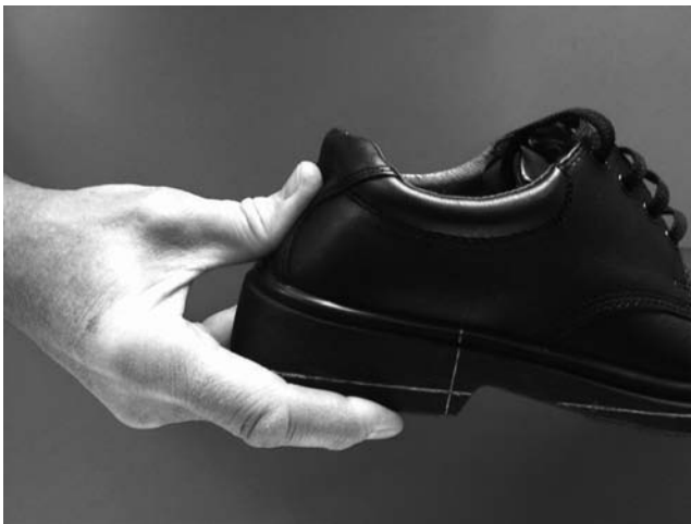
FIGURE 20.1 Method for manual assessment of heel counter stiffness.
