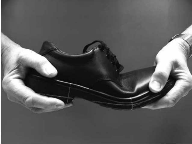
FIGURE 20.2 Method for manual assessment of flexion stiffness.
