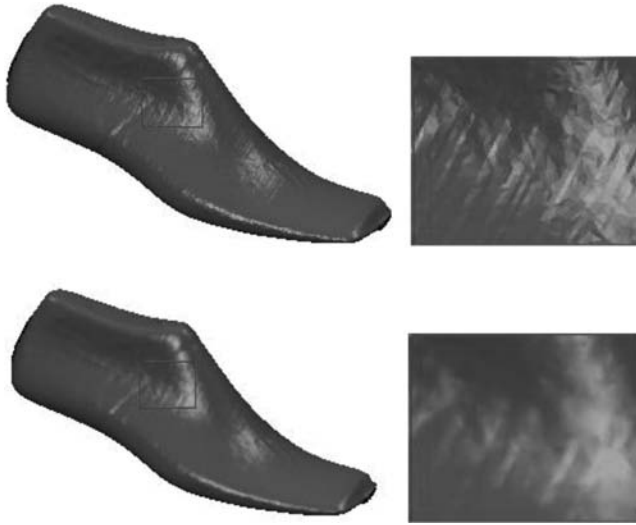
FIGURE 7.2 Original point cloud model with noise and denoised model.
