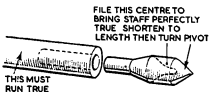
FIG. 290a.—METHOD OF PUTTING IN A NEW CONICAL PIVOT AND SHOULDER TO A CHRONOMETER BALANCE STAFF OR 'SCAPE PINION.
