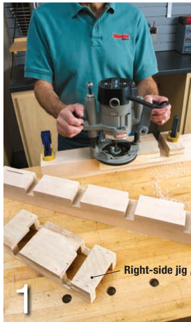
Use a jig (see illustration, p. 10) and a router with a straight bit and a guide to mill the bench-top laminations.
